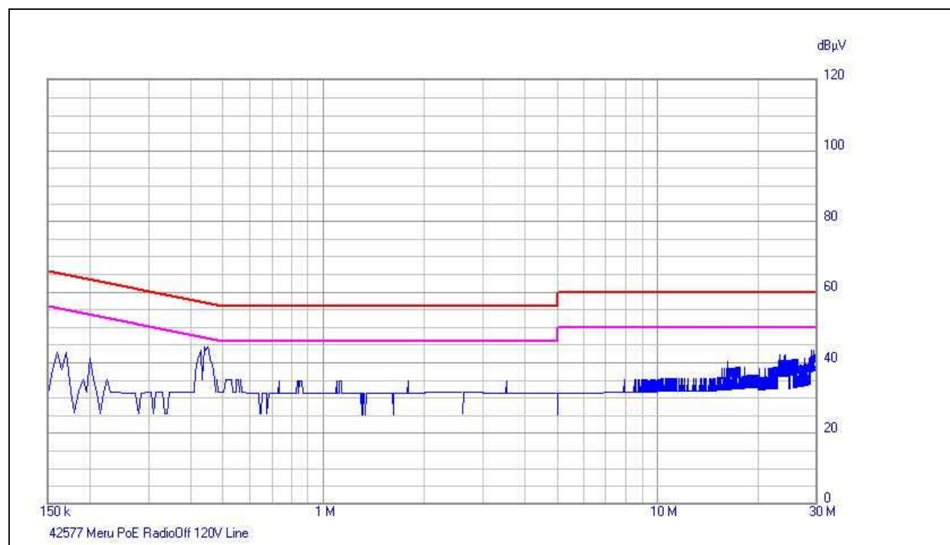
Plot 9. Conducted Emissions, 15.207(a), Phase Line, PoE
