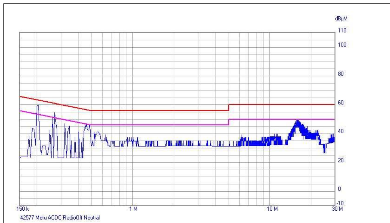
Plot 4. Conducted Emissions, Neutral Line, AC/DC
