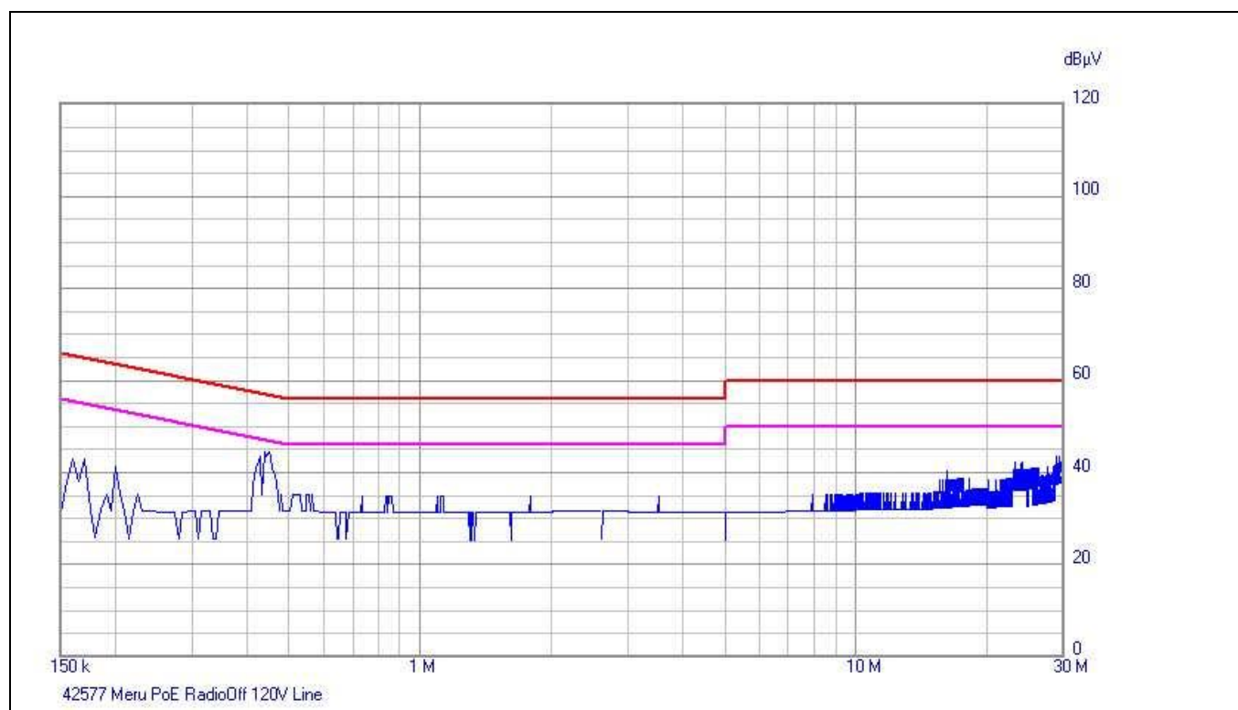
Plot 1. Conducted Emissions, Phase Line, PoE
