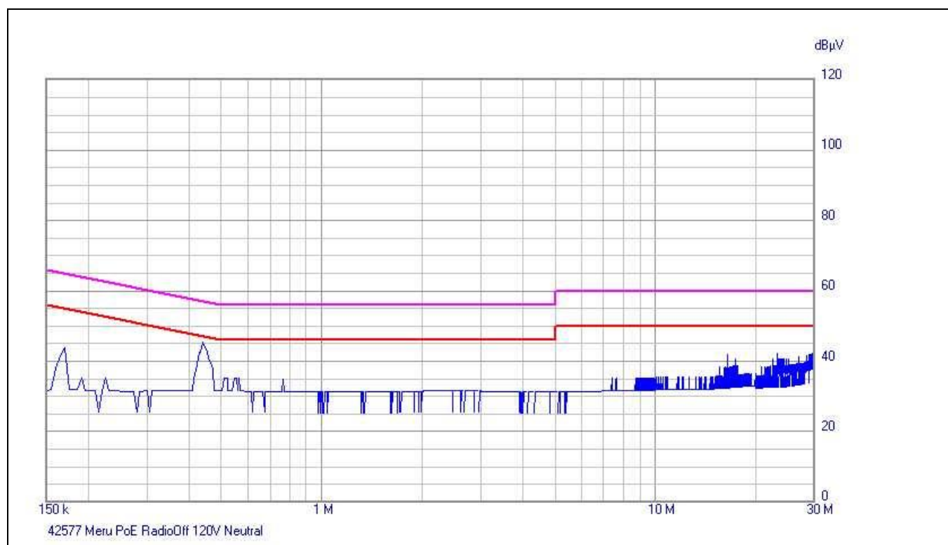
Plot 10. Conducted Emissions, 15.207(a), Neutral Line, PoE
