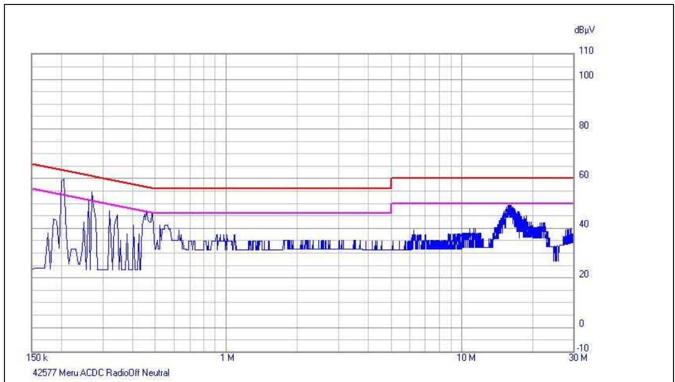
Plot 12. Conducted Emissions, 15.207(a), Neutral Line, AC/DC
