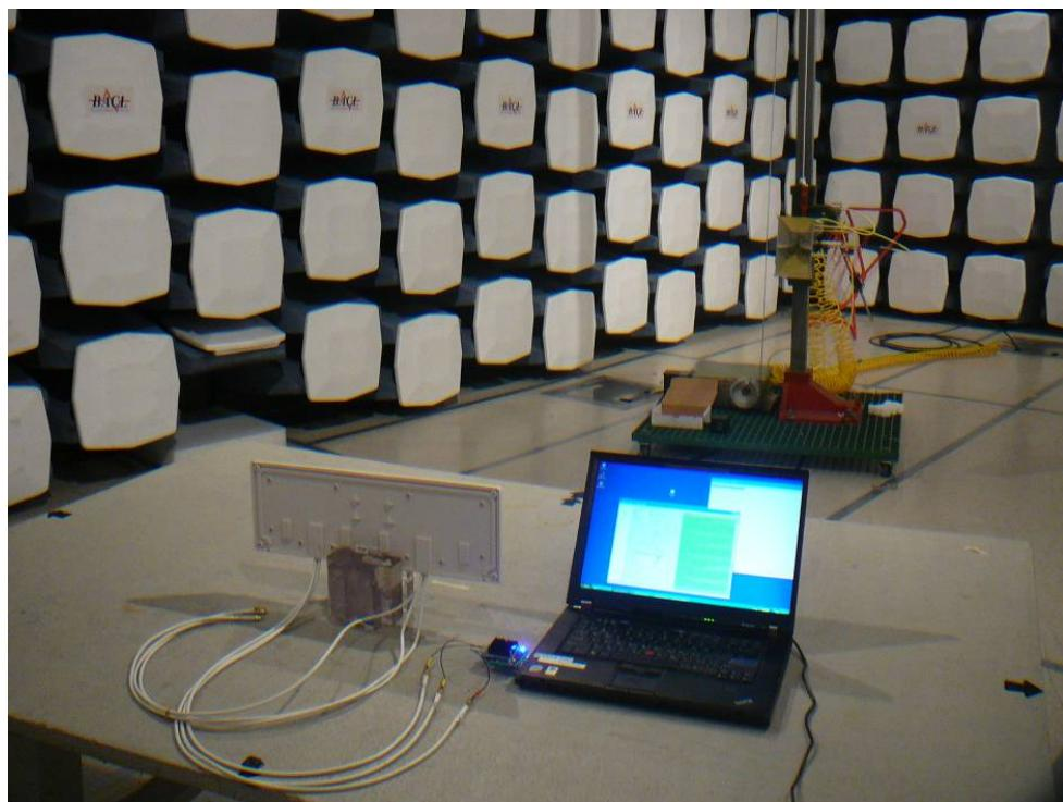
**15.9 Radiated Emission below 1 GHz Front View @ACC-ANT-BG080-NM**
