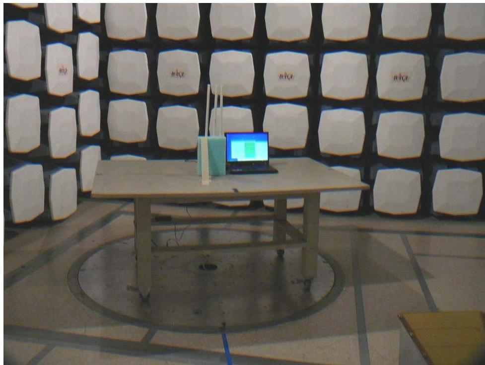
**15.12 Radiated Emission above 1 GHz Rear View @ACC-ANT-BG080-NM**
