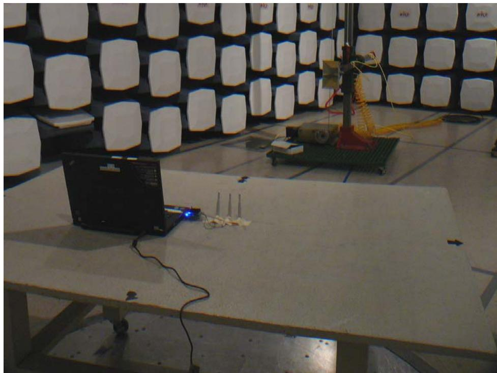
**15.5 Radiated Emission below 1 GHz Front View @ACC-ANT-06ABGN-0607-PT**
