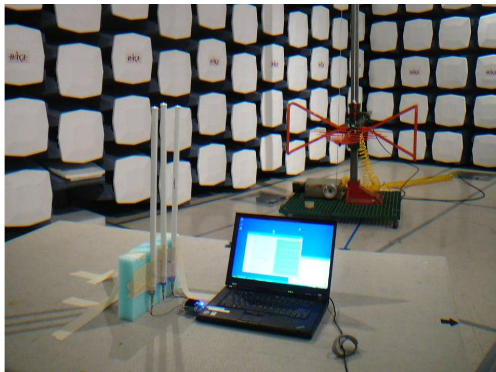
**15.11 Radiated Emission above 1 GHz Front View @ACC-ANT-BG080-NM**
