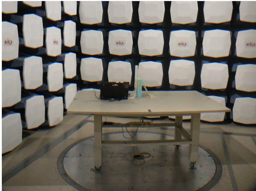
**15.14 Radiated Emission below 1 GHz Rear View @ACC-ANT-A080-NM-1**
