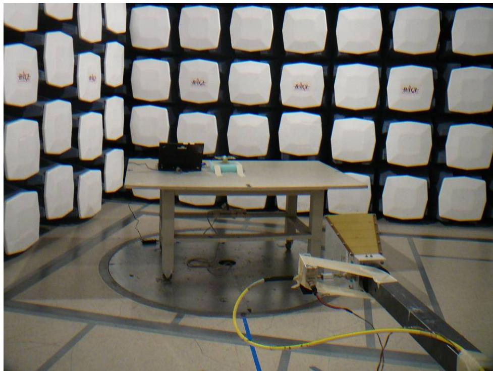
**15.20 Radiated Emission above 1 GHz Rear View @ACC-ANT-A080-NM-1**
