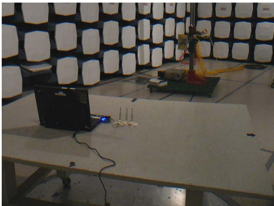
**15.3 Radiated Emission above 1 GHz Front View @ACC-ANT-ABGN230-N**
