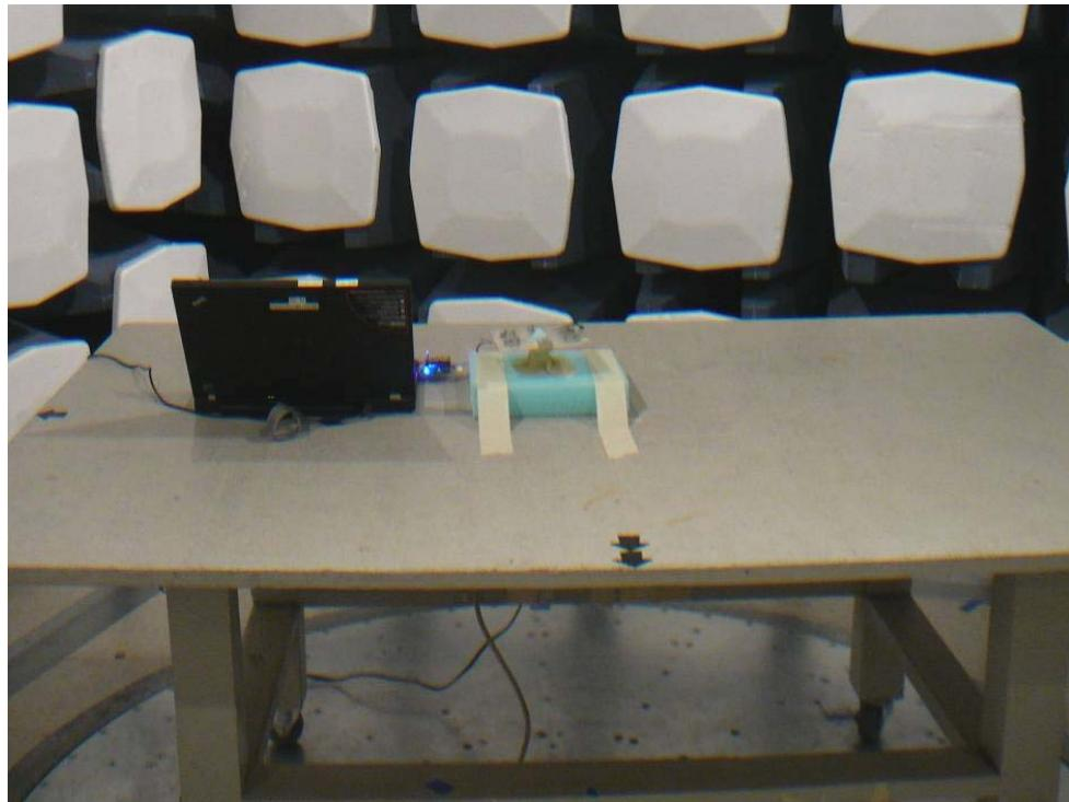
**15.18 Radiated Emission below 1 GHz Rear View @MERU-ANT-PI622**
