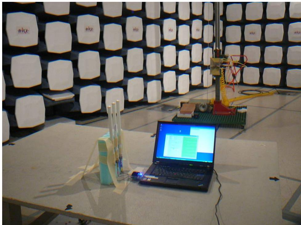
**15.17 Radiated Emission below 1 GHz Front View @MERU-ANT-PI622**
