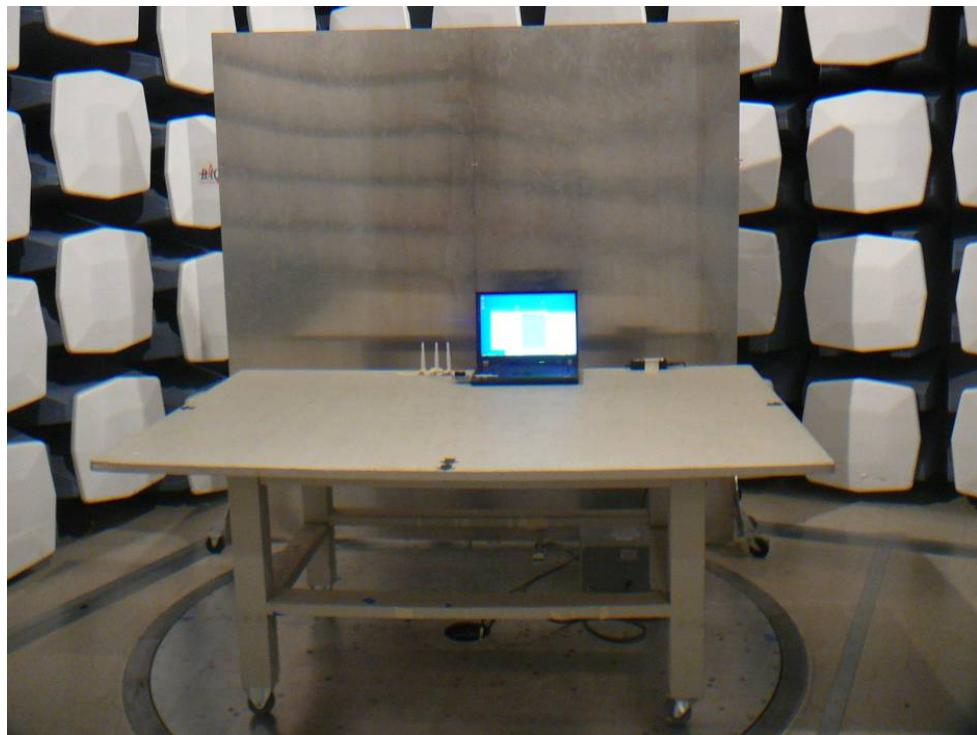
**15.22 Conducted Emission side View @ACC-ANT-ABGN230-W**
