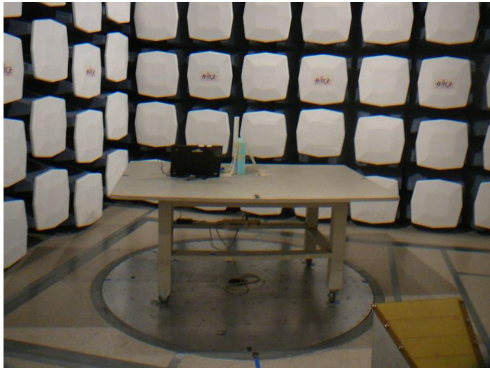
**15.16 Radiated Emission above 1 GHz Rear View @ACC-ANT-A080-NM-1**
