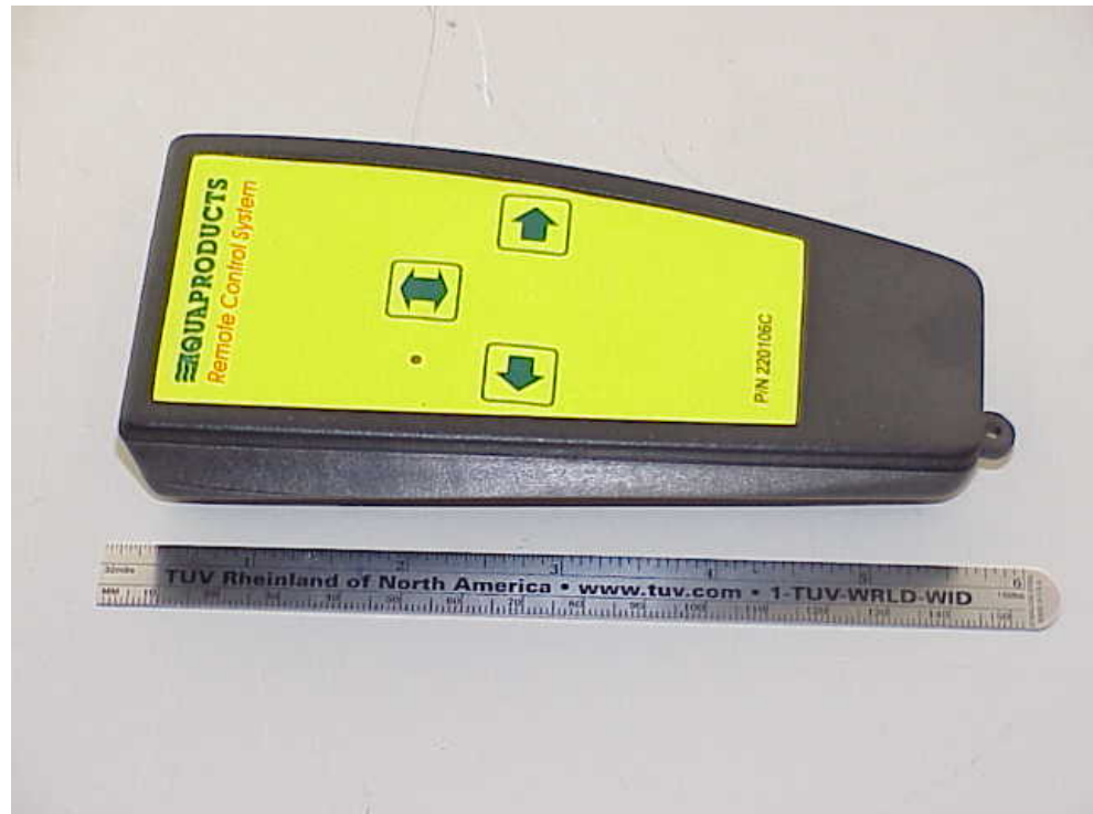
Overall View of Transmitter module
