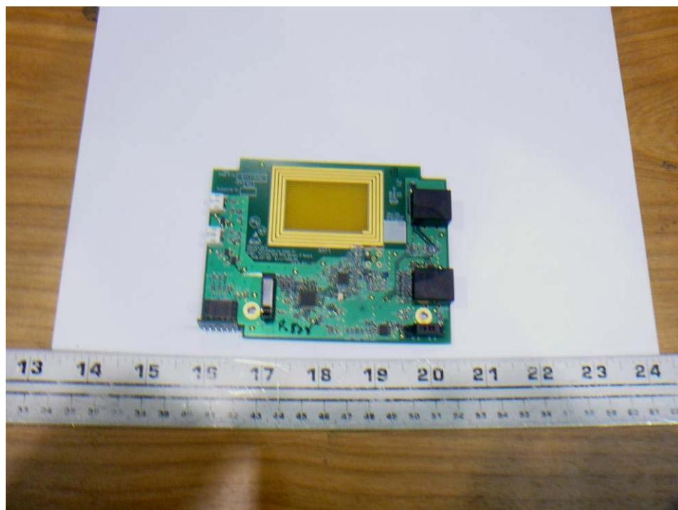
**11.11 EUT – RFID Sensor Solder View**
