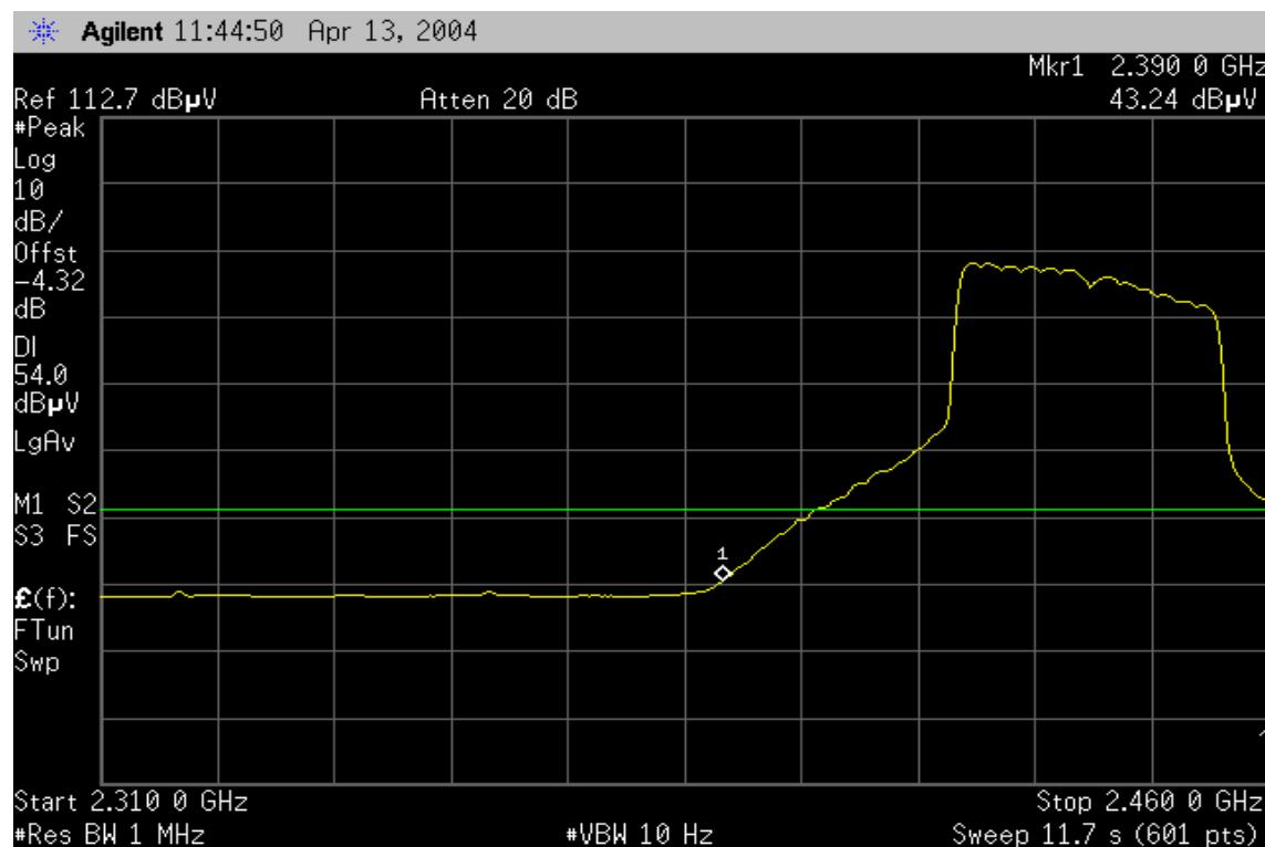
**Band Edges (Upper edge)****Detector mode: Peak****Polarity: Vertical**
