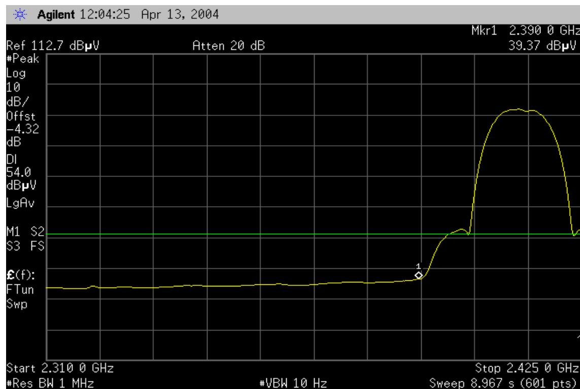
**Band Edges (CH High)****Detector mode: Peak****Polarity: Vertical**
