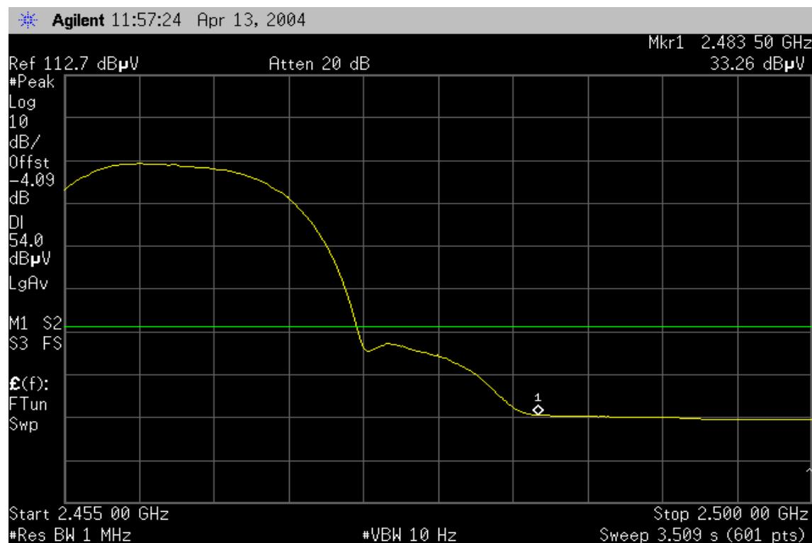
**IEEE 802.11g / Base mode****Band Edges (CH Low)****Detector mode: Peak****Polarity: Vertical**
