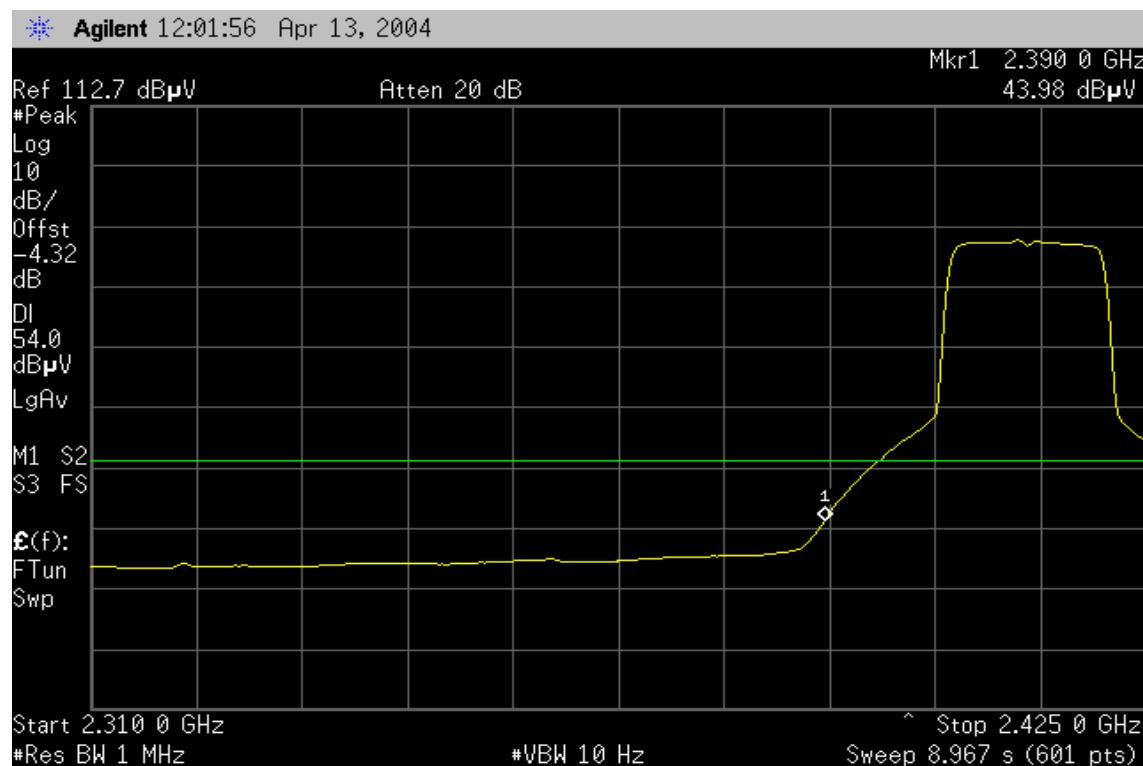
**Band Edges (CH High)****Detector mode: Peak****Polarity: Vertical**
