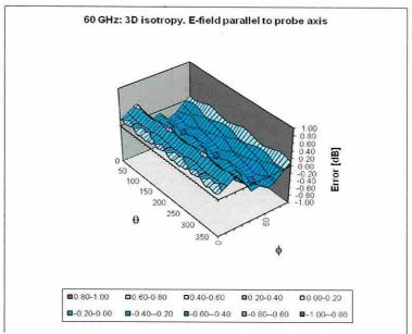
Probe isotropy for E<sub>tot</sub>: probe rotated  $\phi$  = 0° to 360°, tilted from field propagation direction  $\vec{k}$  Parallel to the field propagation ( $\psi$  =0° - 90°) at 30 GHz: deviation within ± 0.42 dB Parallel to the field propagation ( $\psi$  =0° - 90°) at 60 GHz: deviation within ± 0.46 dB
