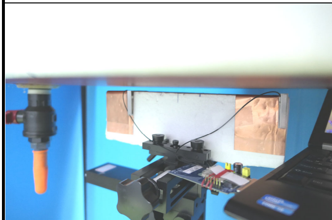
Left Side of EUT Tested at 5 mm
