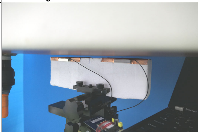
Bottom Side of EUT Tested at 5 mm
