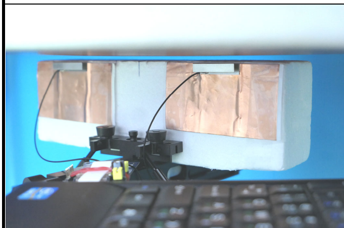
Top Side of EUT Tested at 5 mm
