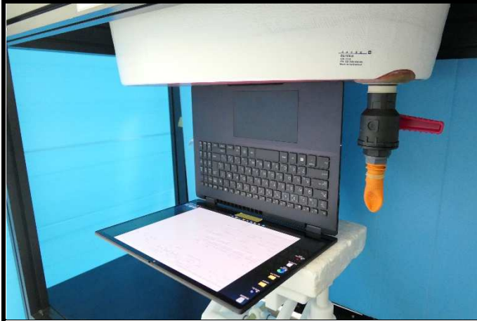
Front Face of Laptop of EUT Tested at 0 mm
