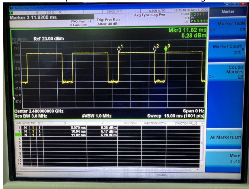
Time-domain plot for Bluetooth transmission signal
