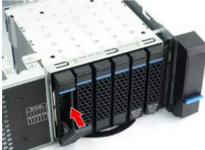
Figure 29 Install SSD Tray
