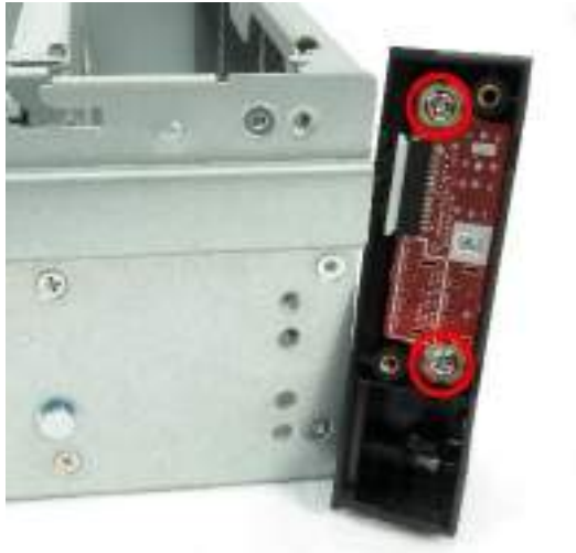
Figure 123 Remove FIO Board Screws
