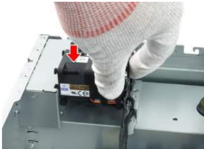
Figure 77 Lower Side Fan
