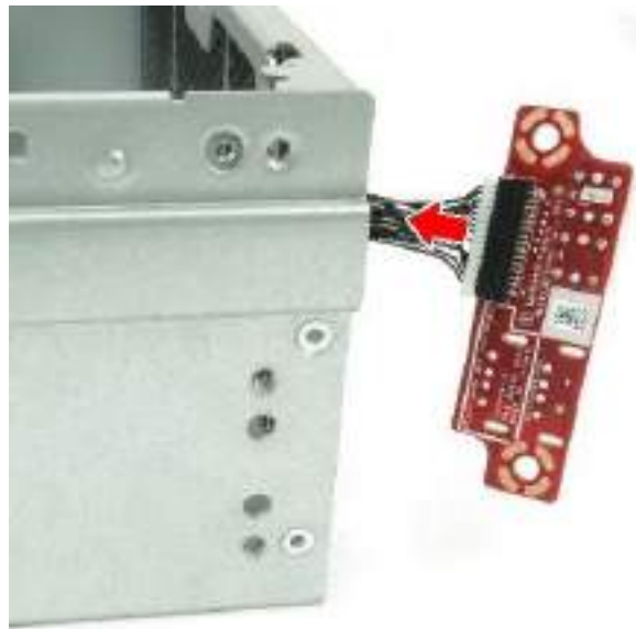
Figure 124 Release FIO Board
