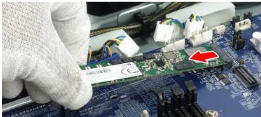
Figure 108 Remove M.2 SSD
