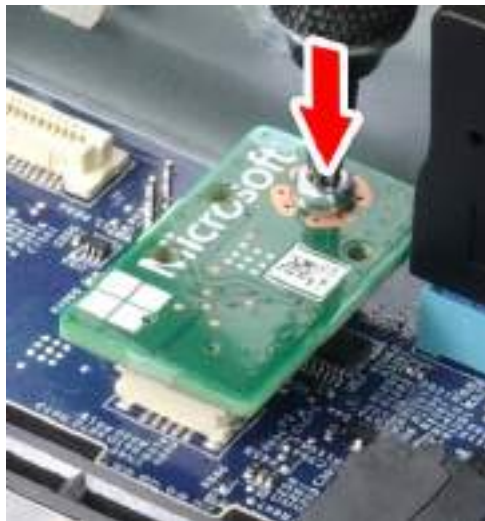
Figure 118 Secure TPM Card
