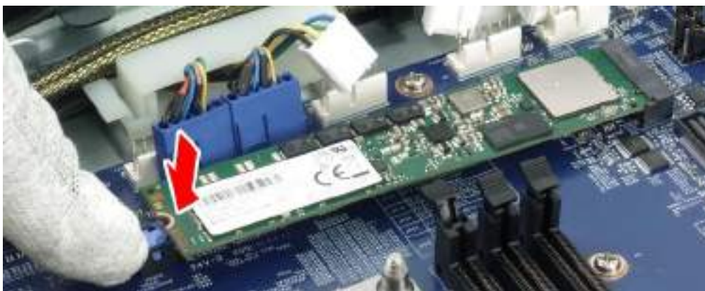
Figure 110 Install M.2 SSD
