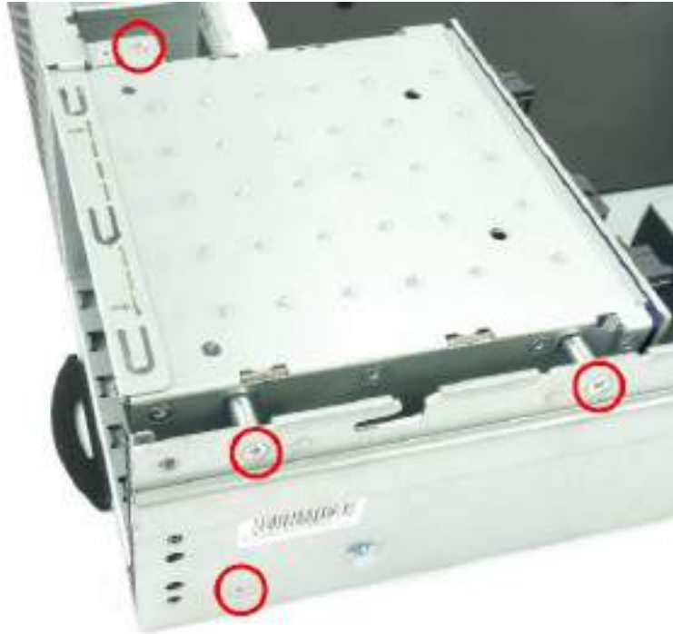
Figure 32 Loosen and Remove SSD Cage Screws
