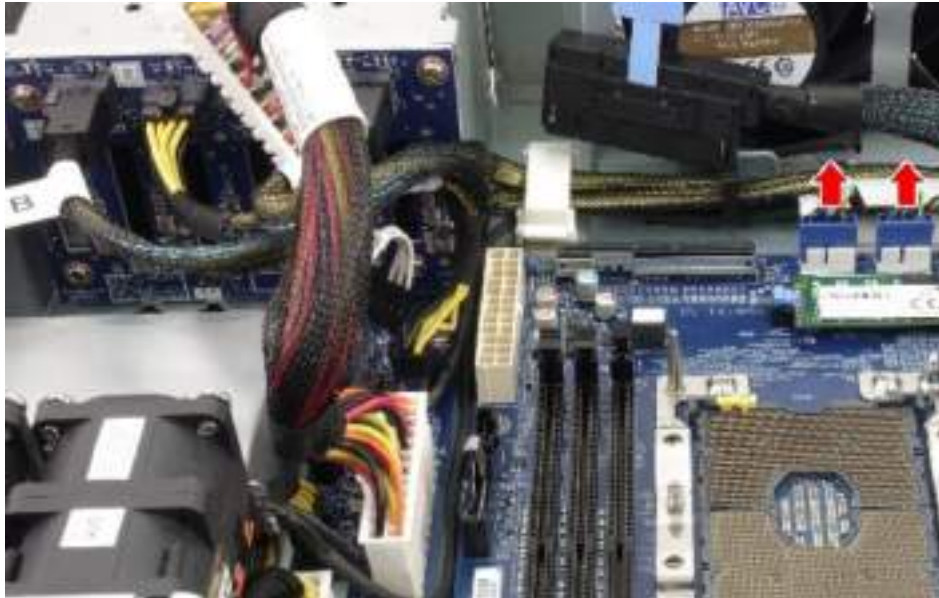
Figure 74 Disconnect Side Fan Connectors
