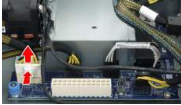
Figure 95 Remove CPU Power Connector
