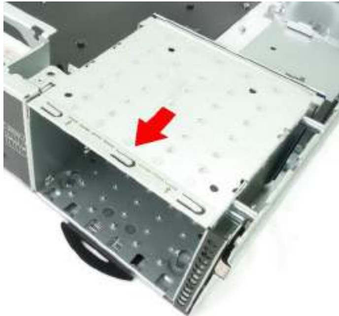
Figure 33 Slide SSD Cage Outward
