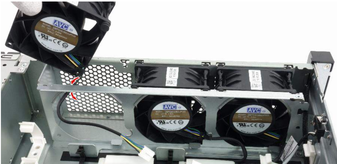
Figure 83 Insert Front Fan Cable
