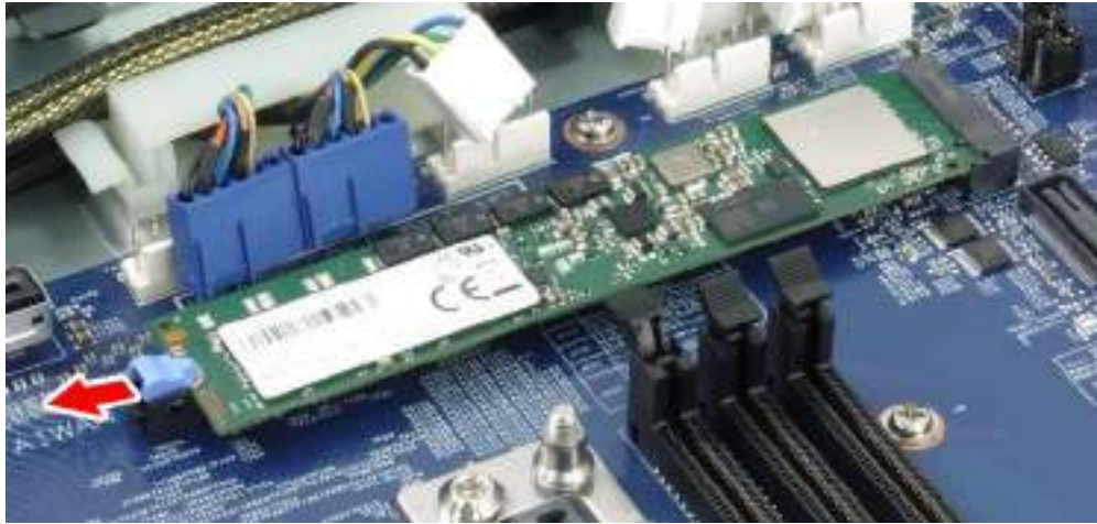
Figure 107 Pull Spring Latch of M.2 SSD Module
