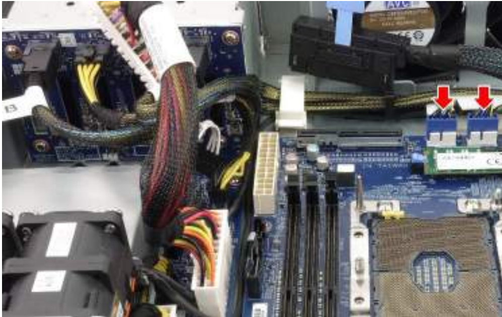
Figure 78 Connect Side Fan Connectors
