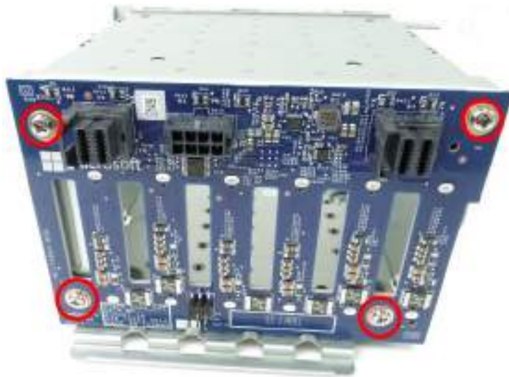
Figure 39 Remove SATA BP Board Screws
