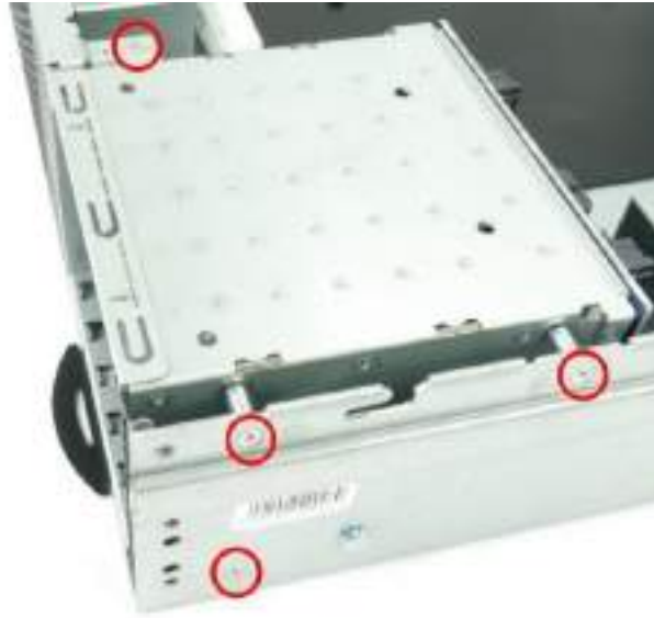
Figure 36 Secure SSD Cage
