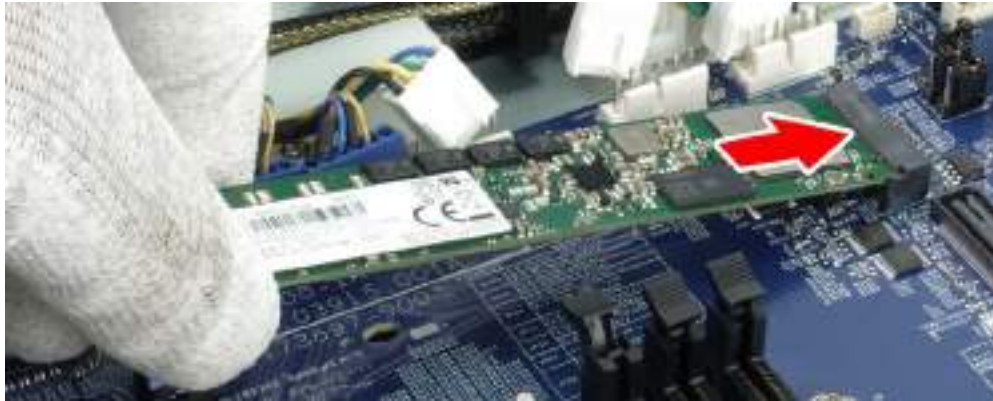
Figure 109 Insert M.2 SSD
