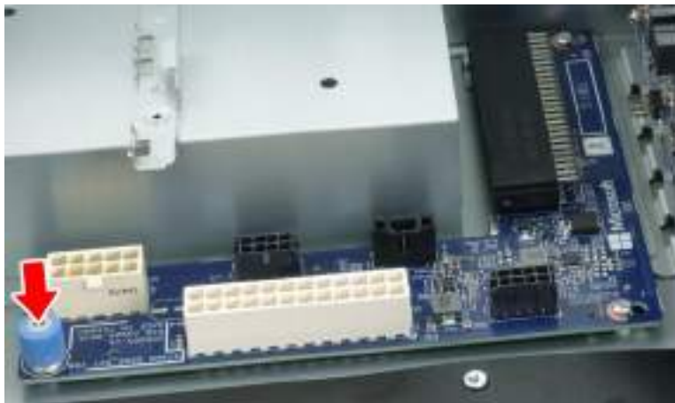
Figure 101 Tighten PDB Thumbscrew
