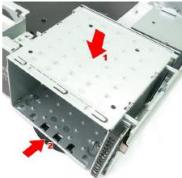
Figure 35 Attach SSD Cage to Chassis
