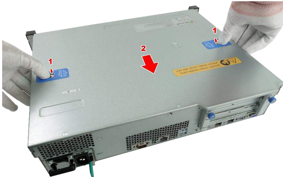
Figure 6 Press Thumbpads and Slide Top Cover
