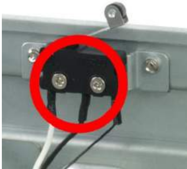
Figure 90 Position and Secure Intrusion Switch
