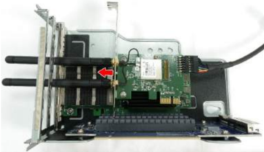
Figure 65 Insert Second PCIe Card 1
