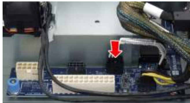
Figure 104 Install PSU Control Connector
