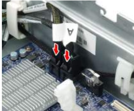
Figure 138 Install SATA Connectors onto Mainboard
