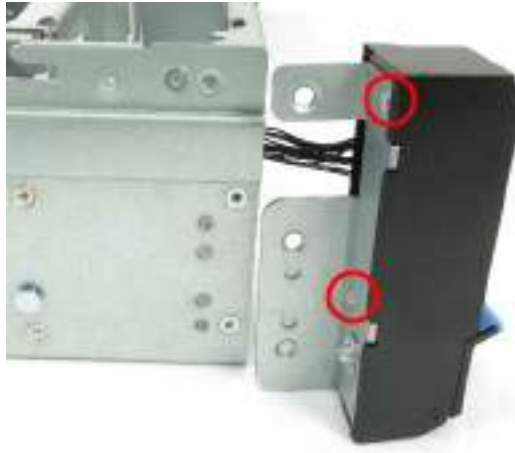
Figure 127 Secure FIO Bracket Screws
