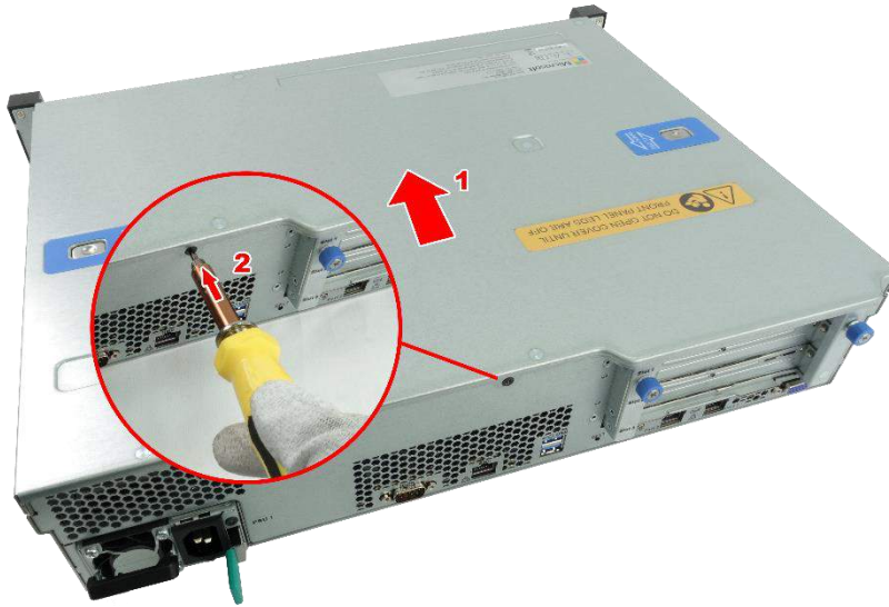
Figure 9 Slide Top Cover and Secure with Screw
