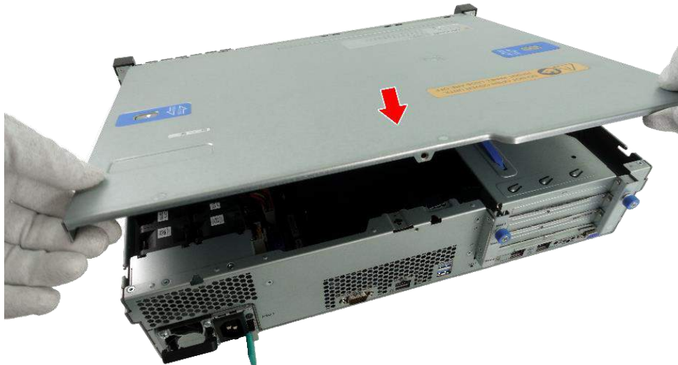
Figure 8 Lower the Top Cover
