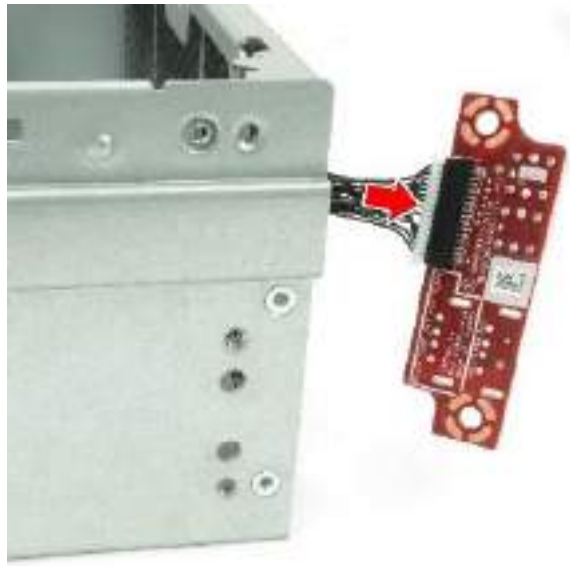
Figure 125 Connect FIO Board Connector Cable to FIO Board
