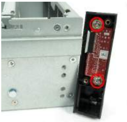
Figure 126 Secure FIO Board to Left Ear Module
