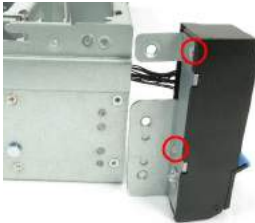
Figure 122 Remove FIO Bracket Screws
