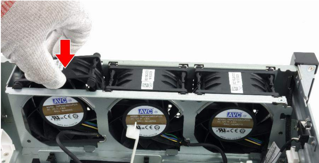
Figure 84 Insert Front Fan
