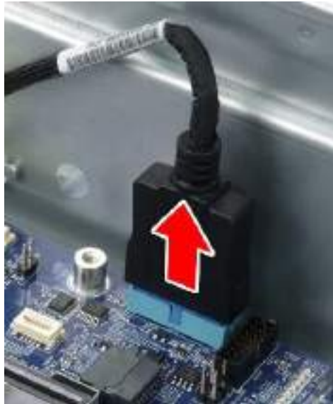
Figure 119 Remove FIO-to-MB Connector
