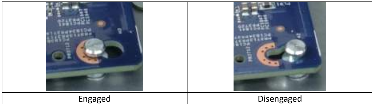
Figure 100 Lower PDB and Engage Standoffs
