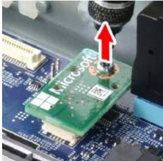
Figure 115 Remove TPM Card Screw
