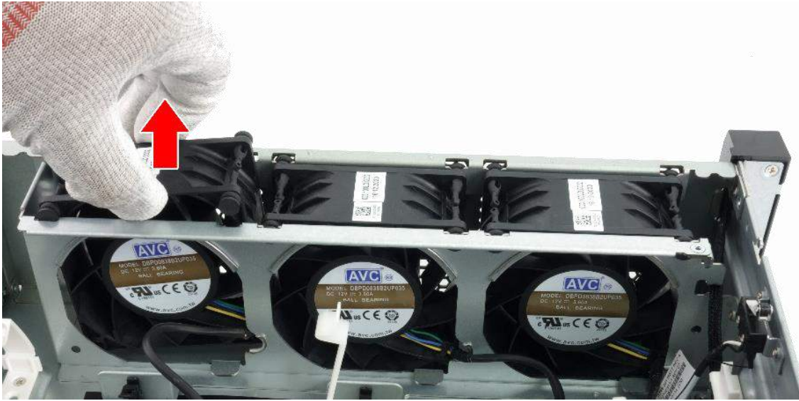
Figure 82 Remove Front Fan
