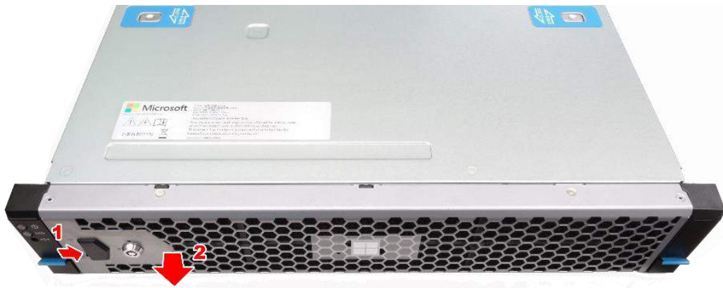
Figure 11 Unlock Slide Lock and Pull Bezel Out
