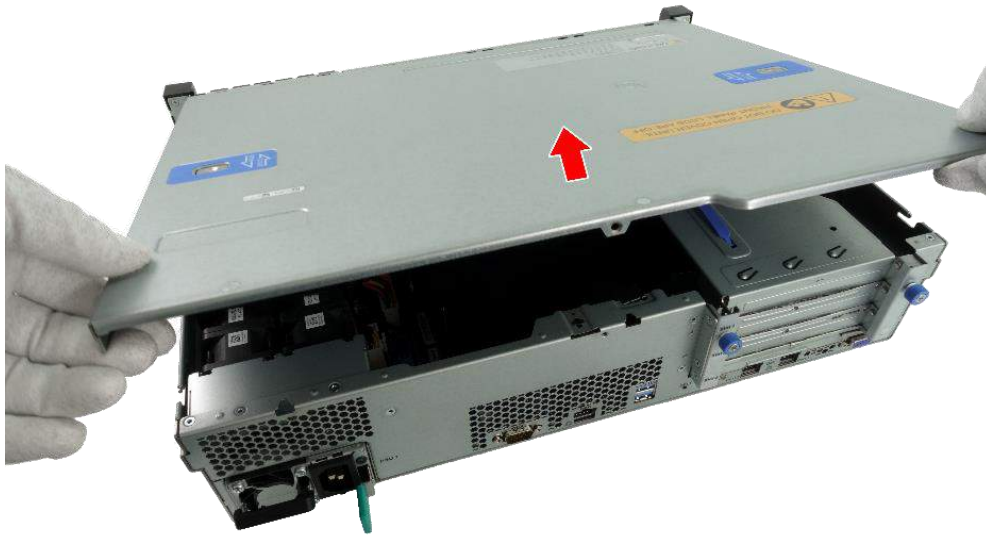
Figure 7 Remove Top Cover
