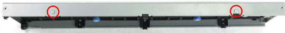
Figure 13 Remove Filter Bracket Screws
