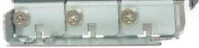
Figure 68 Secure PCIe Cards to Window Slots
