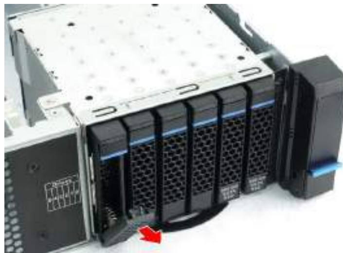
Figure 26 Pull to Remove SSD Tray
