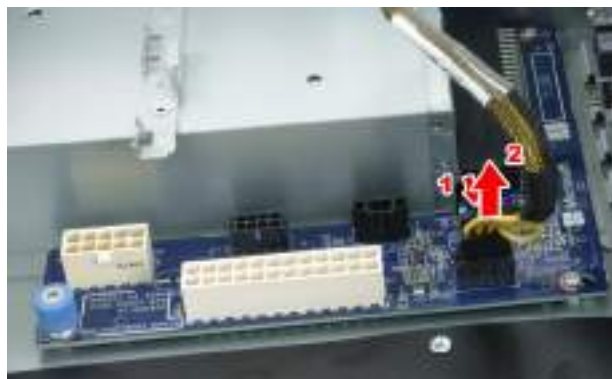
Figure 94 Remove SATA BP Board Connector
