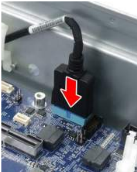
Figure 130 Insert the FIO-to-MB Connector
