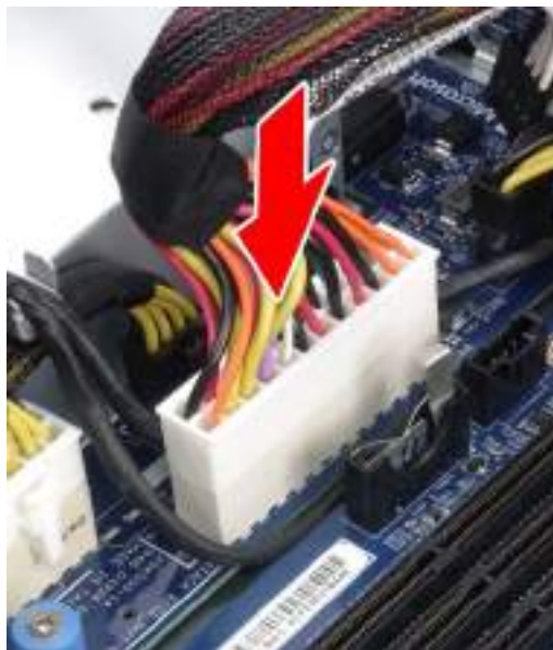
Figure 106 Install Mainboard-to-Power Connector
