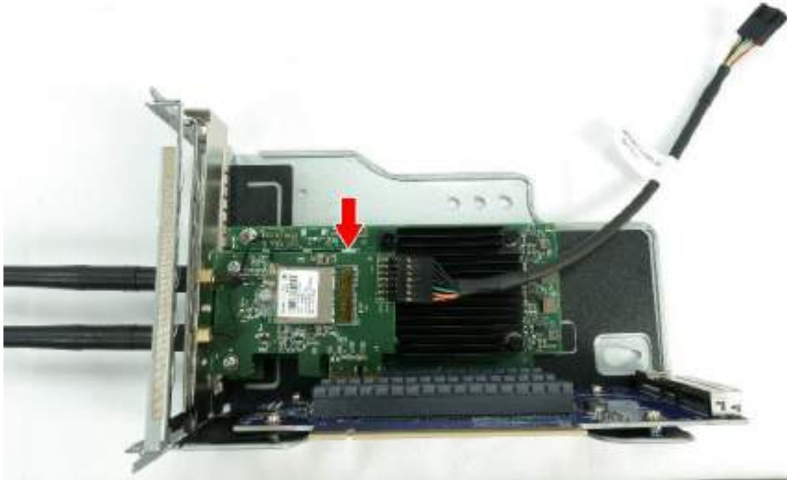
Figure 66 Insert Second PCIe Card 2
