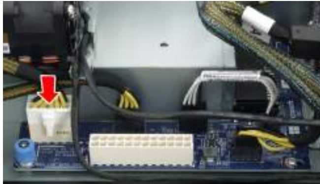
Figure 102 Install CPU Power Connector
