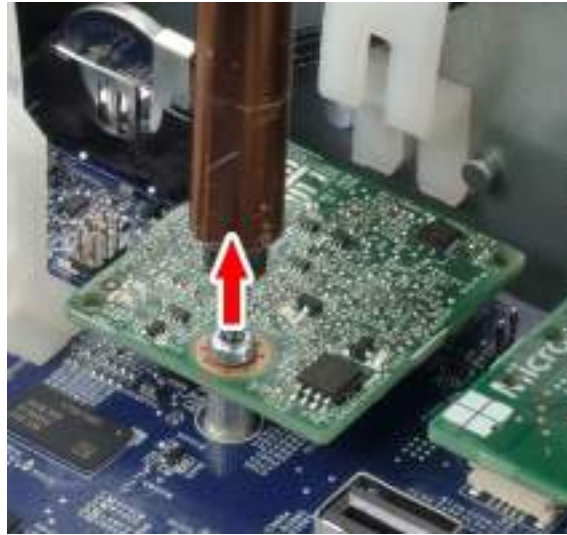
Figure 111 Remove Cerberus Card Screw
