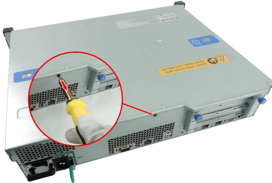
Figure 5 Remove Top Cover Screw
