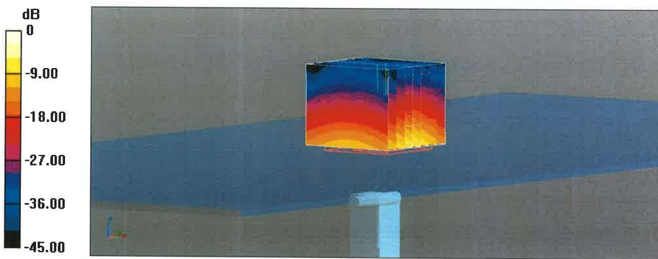
$$0 \text{ dB} = 19.6 \text{ W/kg} = 12.92 \text{ dBW/kg}$$
