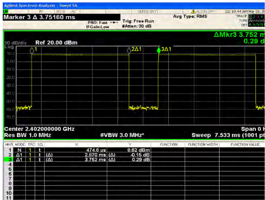
Time-domain plot for Bluetooth transmission signal
