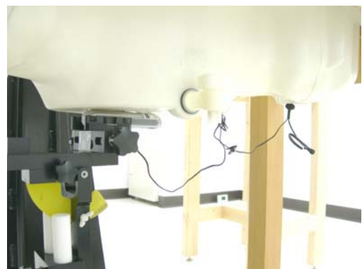
Figure 18. Body SAR Test Setup (Flat Section)
