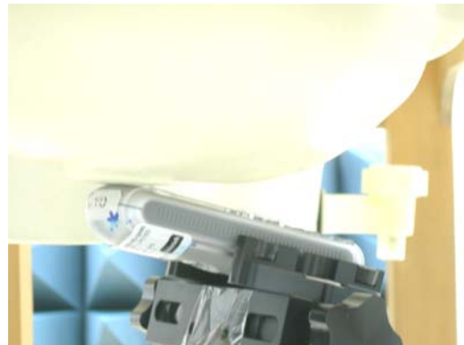
Figure 14. Right Head SAR Test Setup (Tilted)
