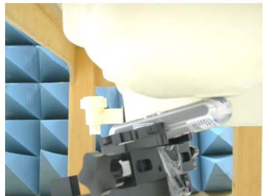
Figure 16. Left Head SAR Test Setup (Tilted)
