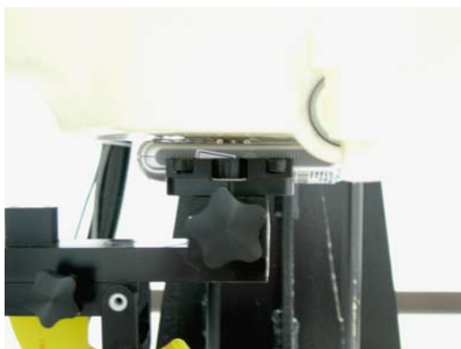
Figure 17. Body SAR Test Setup (Flat Section)
