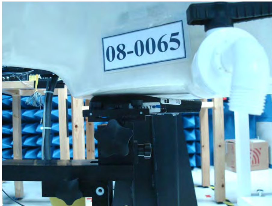
Figure 18.Body SAR Test Setup_ (Flat Section)
