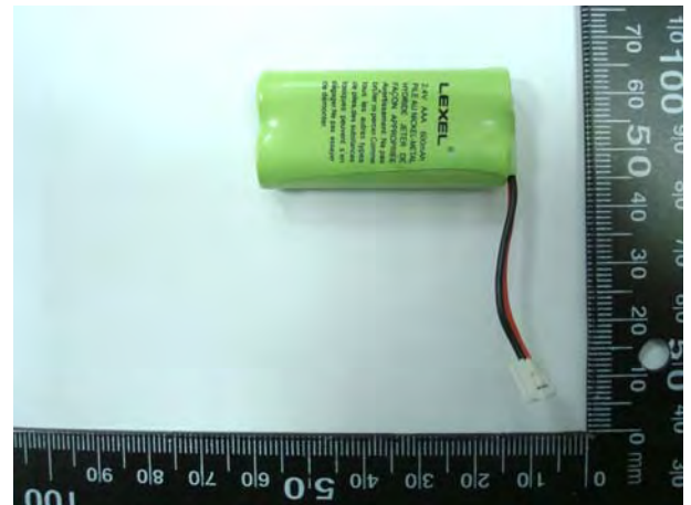
Figure 3. Battery (Ni-MH 2.4V , 600mAh)
