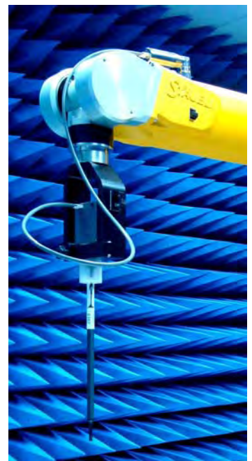
Figure 8. Probe setup on robot
