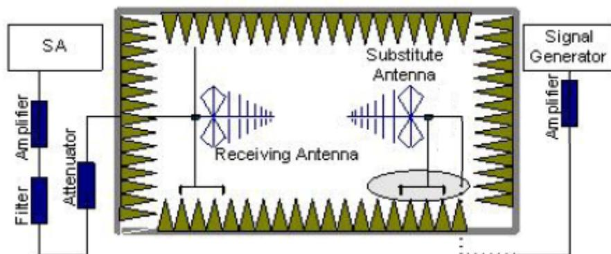
In the chamber, a substitution antenna for the frequency band of interest is placed at the reference point of the chamber. An RF signal source for the frequency band of interest is connected to the substitution antenna with a cable that has been constructed to not interfere with the radiation pattern of the antenna. A power ( $P_{Mea}$ ) is applied to the input of the substitution antenna. Adjust the level of the signal generator output until the value of the
