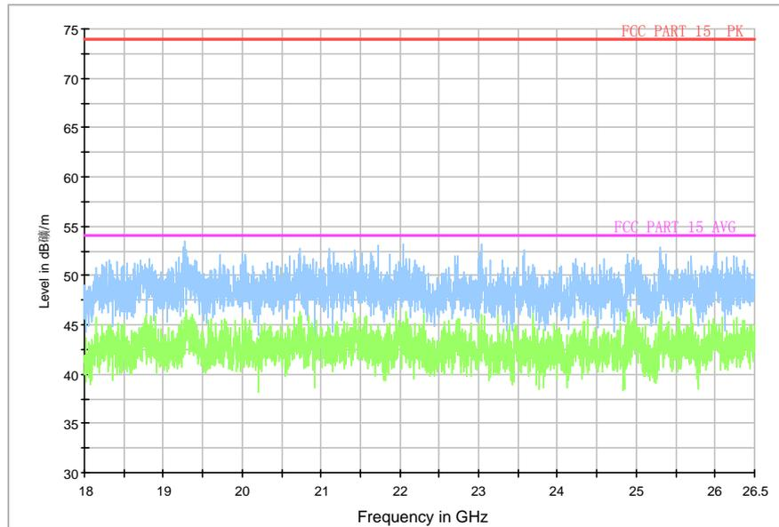
Fig.28. Transmitter Spurious Emission - Radiated: GFSK, 18 GHz - 26 GHz
