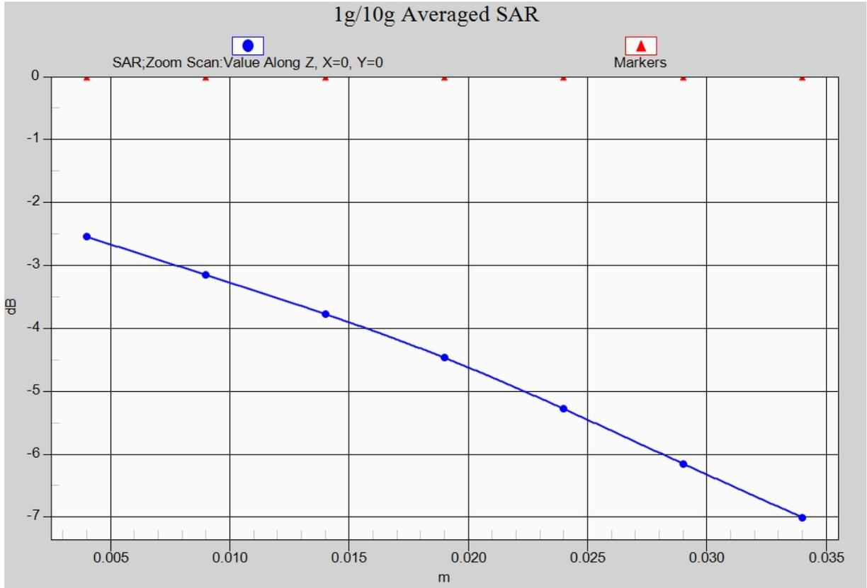
Fig. 5-1 Z-Scan at power reference point (LTE Band13)
