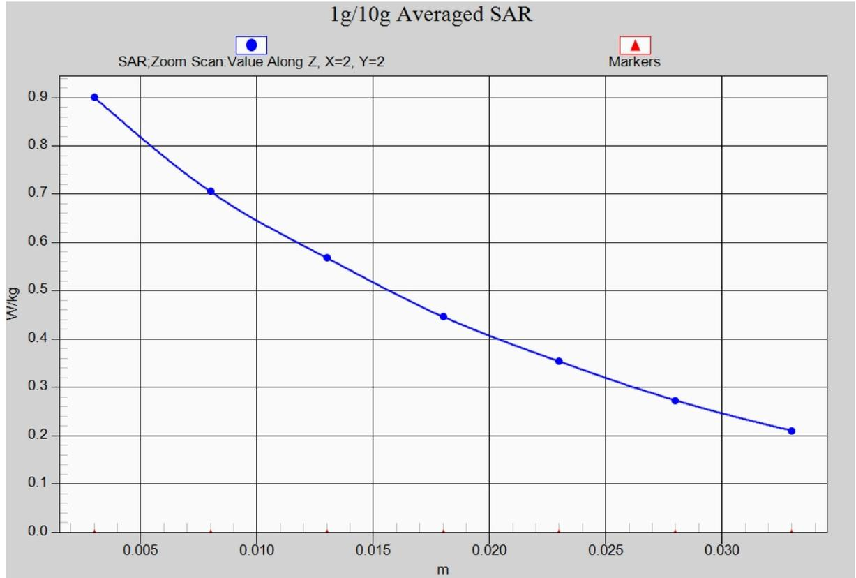
Fig. 2-1 Z-Scan at power reference point (CDMA BC0)
