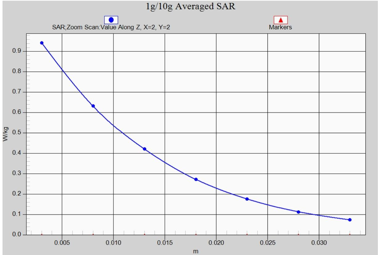
Fig.4-1 Z-Scan at power reference point (CDMA BC1)
