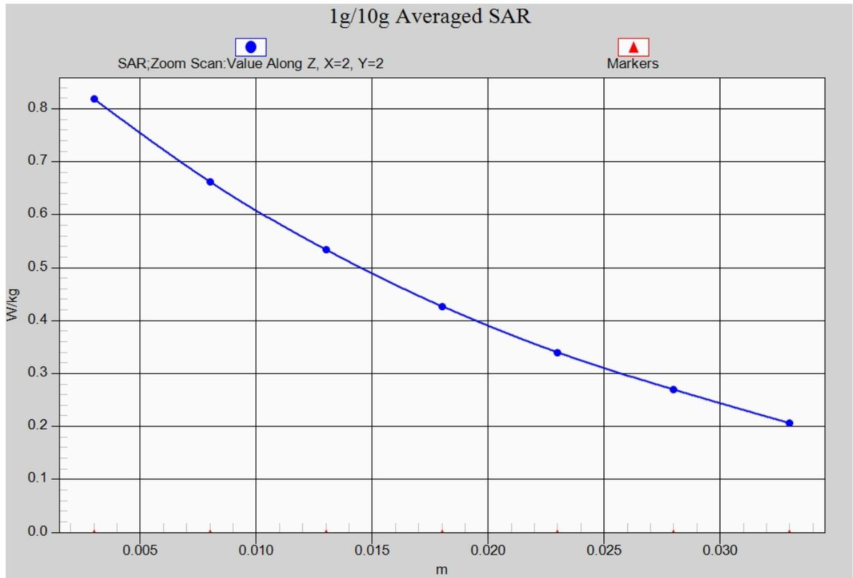
Fig. 6-1 Z-Scan at power reference point (LTE Band13)
