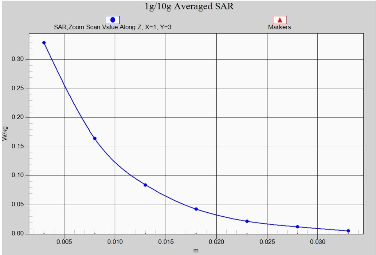
Fig. 8-1 Z-Scan at power reference point (2450 MHz)
