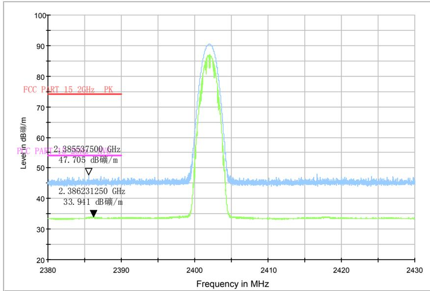
Fig.85. Radiated emission (Power): 8DPSK, low channel
