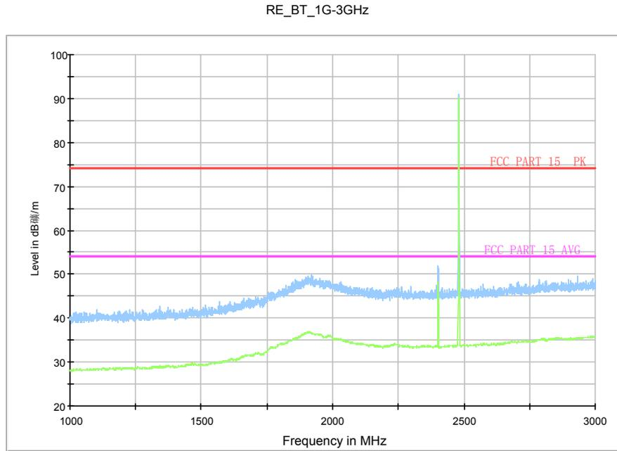
Fig.63. Radiated emission: GFSK, Channel 78, 1 GHz - 3 GHz
