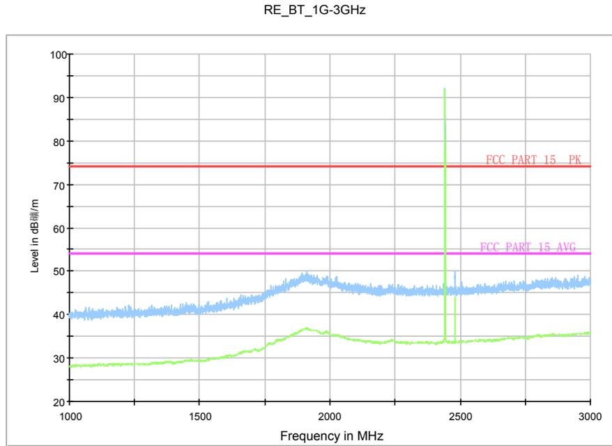
Fig.61. Radiated emission: GFSK, Channel 39, 1 GHz - 3 GHz
