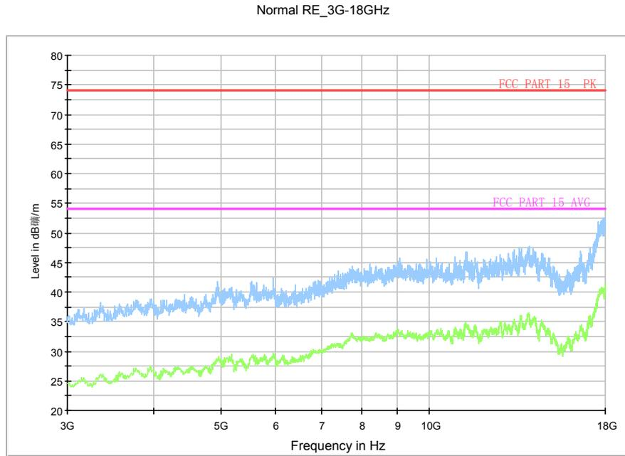
Fig.79. Radiated emission: 8DPSK, Channel 0, 3 GHz - 18 GHz
