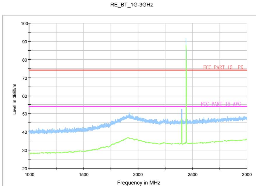
Fig.71. Radiated emission:  $\pi/4$  DQPSK, Channel 39, 1 GHz - 3 GHz
