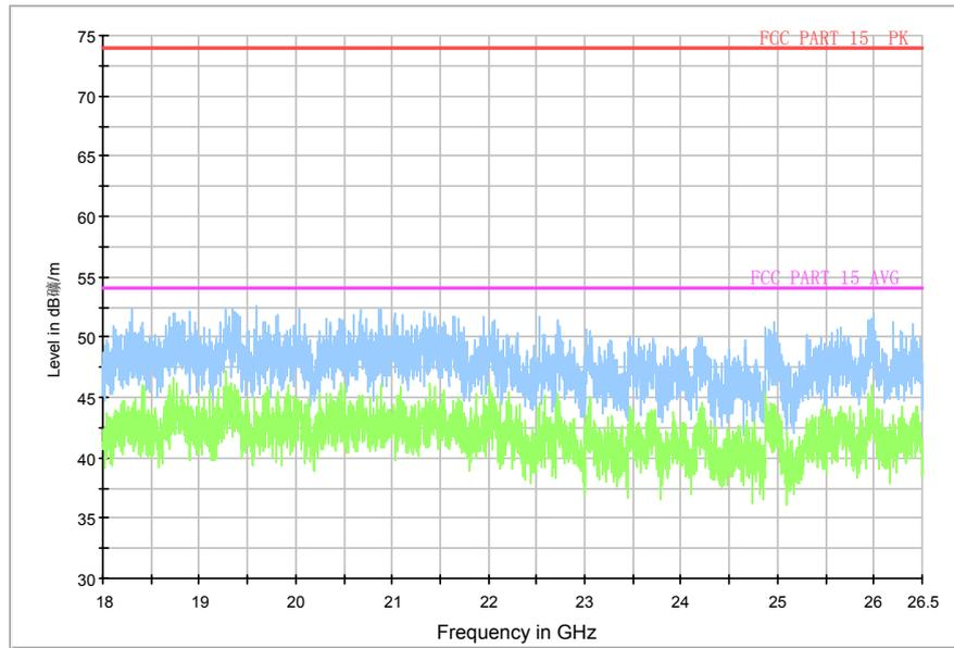
Fig.87. Radiated emission: 8DPSK, 18 GHz - 26 GHz
