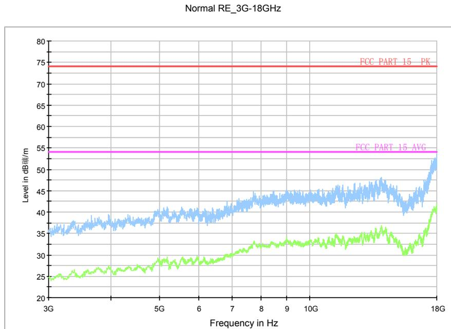
Fig.69. Radiated emission:  $\pi/4$  DQPSK, Channel 0, 3 GHz - 18 GHz
