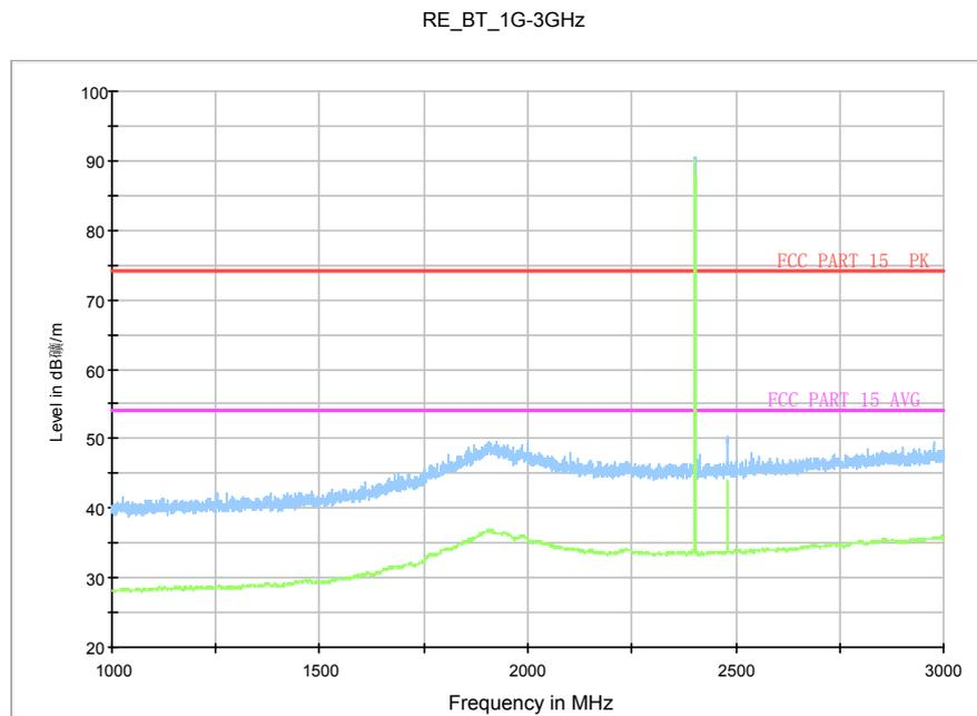
Fig.58. Radiated emission: GFSK, Channel 0, 1 GHz - 3 GHz
