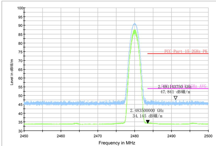
Fig.86. Radiated emission (Power): 8DPSK, high channel
