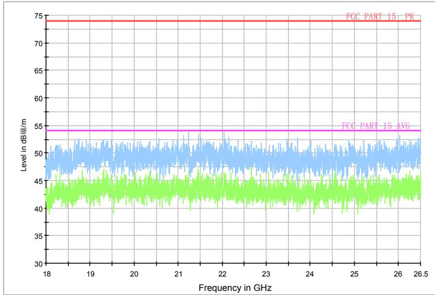
Fig.67. Radiated emission: GFSK, 18 GHz - 26 GHz
