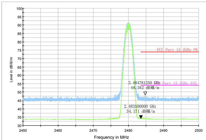
Fig.66. Radiated emission (Power) GFSK, high channel
