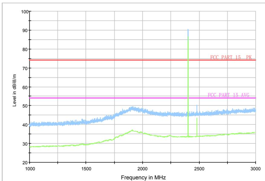
Fig.78. Radiated emission: 8DPSK, Channel 0, 1 GHz - 3 GHz
