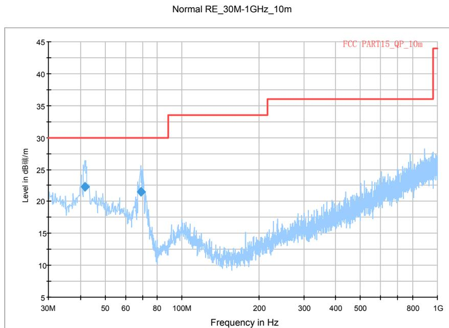
Fig.80. Radiated emission: 8DPSK, Channel 39, 30 MHz - 1 GHz
