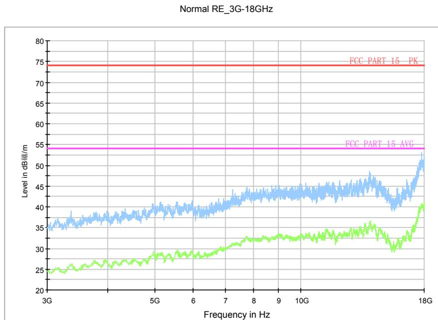
Fig.82. Radiated emission: 8DPSK, Channel 39, 3 GHz - 18 GHz
