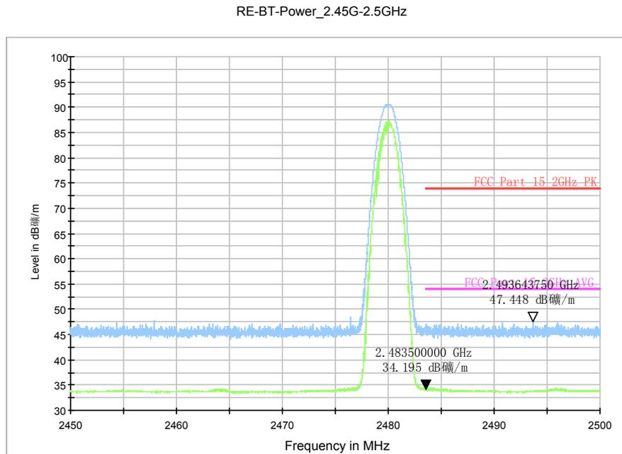
Fig.76. Radiated emission (Power):  $\pi/4$  DQPSK, high channel
