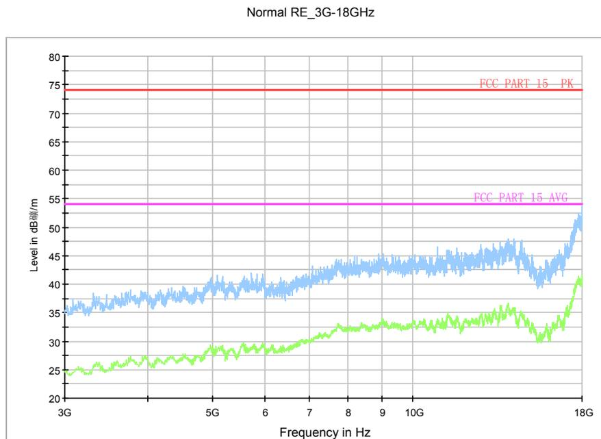
Fig.72. Radiated emission:  $\pi/4$  DQPSK, Channel 39, 3 GHz - 18 GHz
