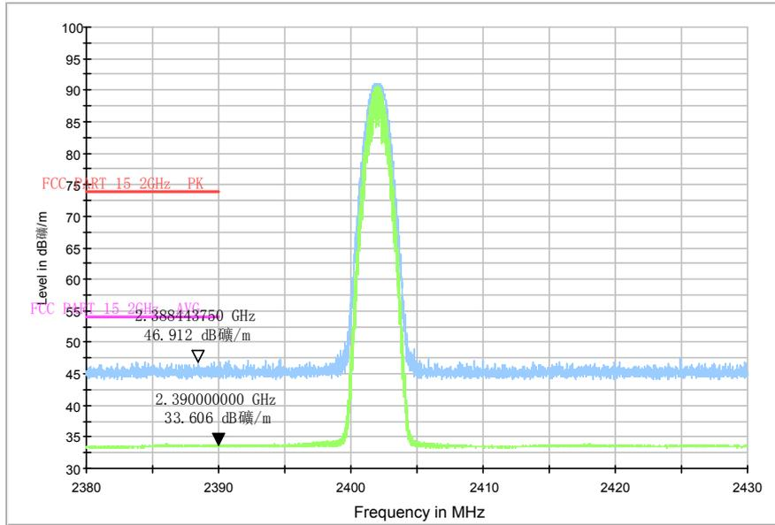
Fig.65. Radiated emission (Power): GFSK, low channel
