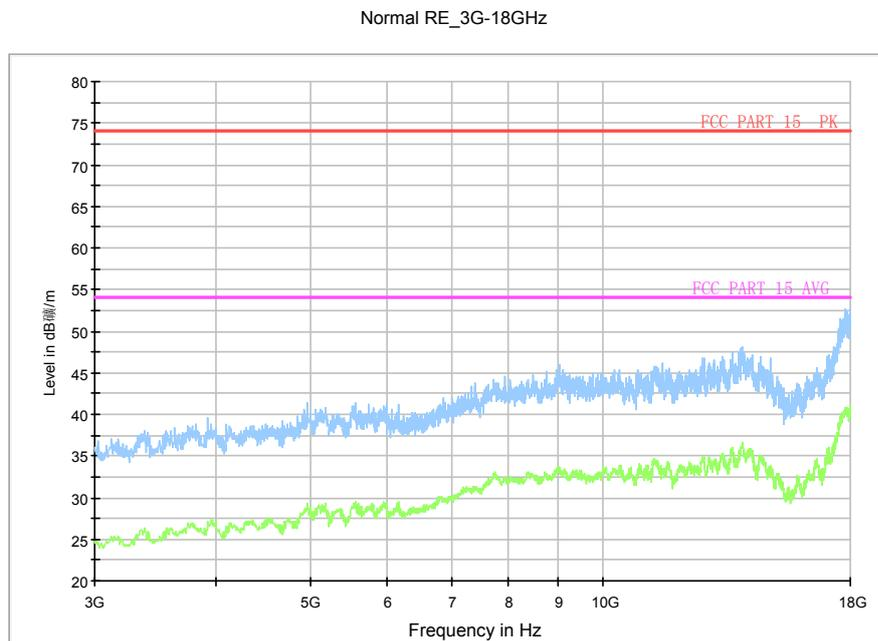
Fig.84. Radiated emission: 8DPSK, Channel 78, 3 GHz - 18 GHz
