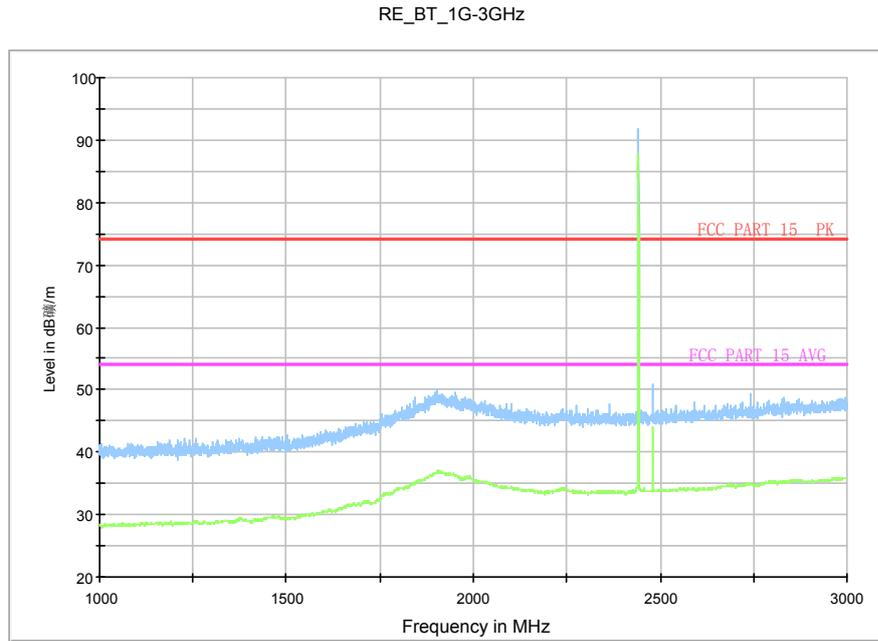
Fig.81. Radiated emission: 8DPSK, Channel 39, 1 GHz - 3 GHz
