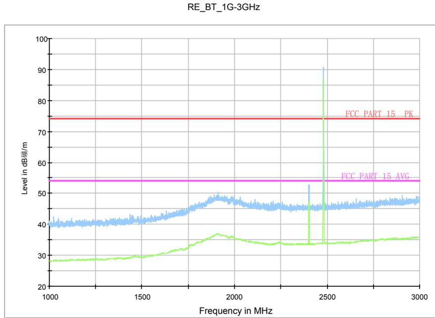
Fig.83. Radiated emission: 8DPSK, Channel 78, 1 GHz - 3 GHz
