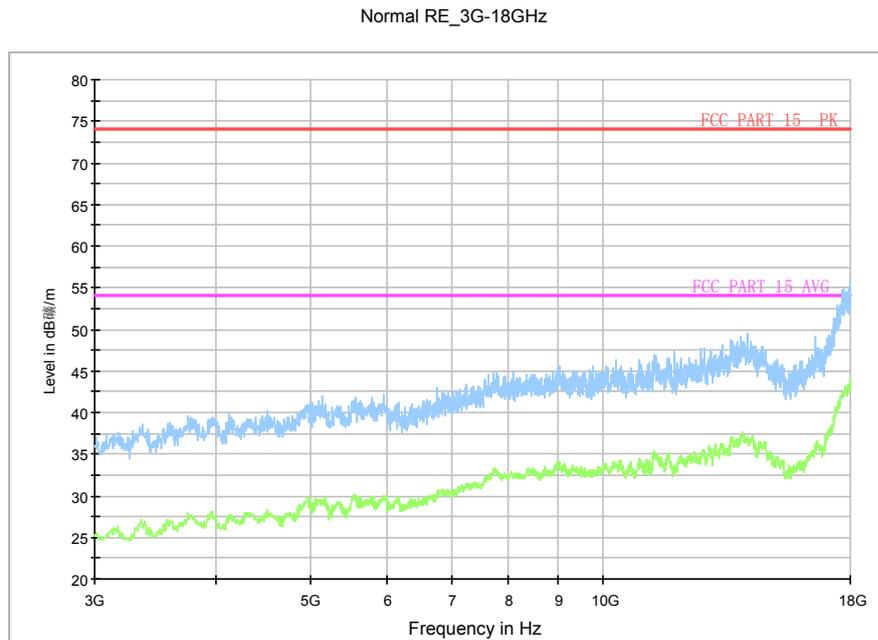
Fig.59. Radiated emission: GFSK, Channel 0, 3 GHz - 18 GHz
