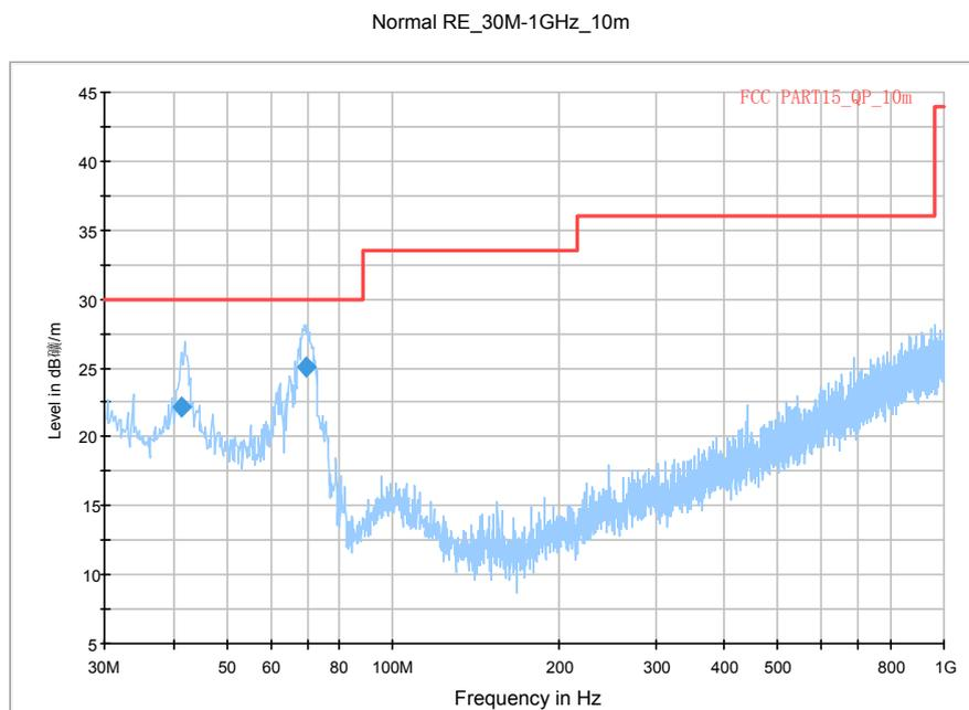
Fig.60. Radiated emission: GFSK, Channel 39, 30 MHz - 1 GHz
