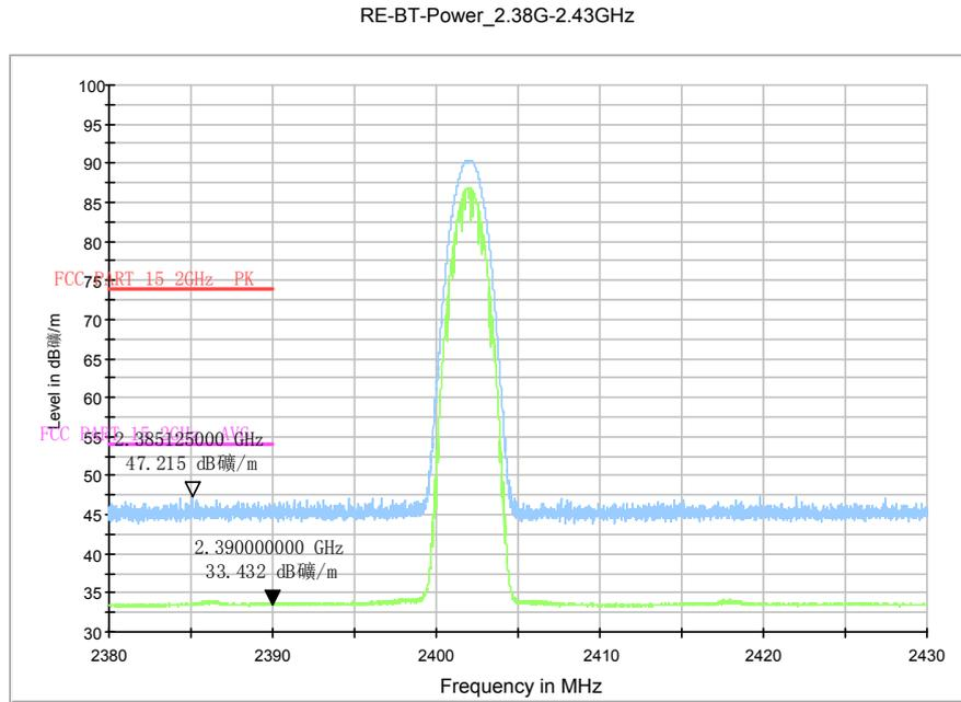
Fig.75. Radiated emission (Power):  $\pi/4$  DQPSK, low channel
