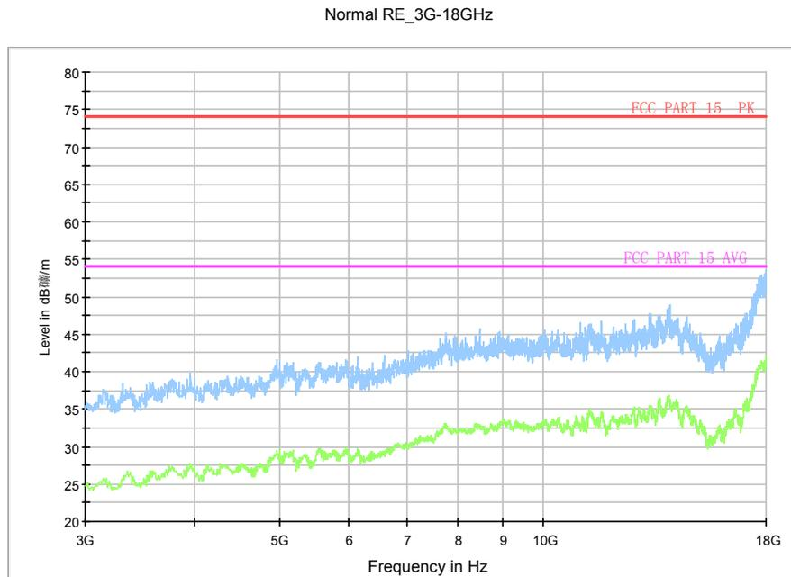
Fig.64. Radiated emission: GFSK, Channel 78, 3 GHz - 18 GHz
