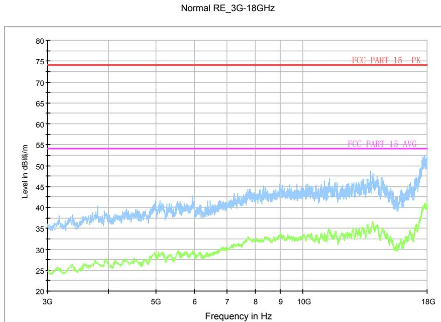
Fig.74. Radiated emission:  $\pi/4$  DQPSK, Channel 78, 3 GHz - 18 GHz
