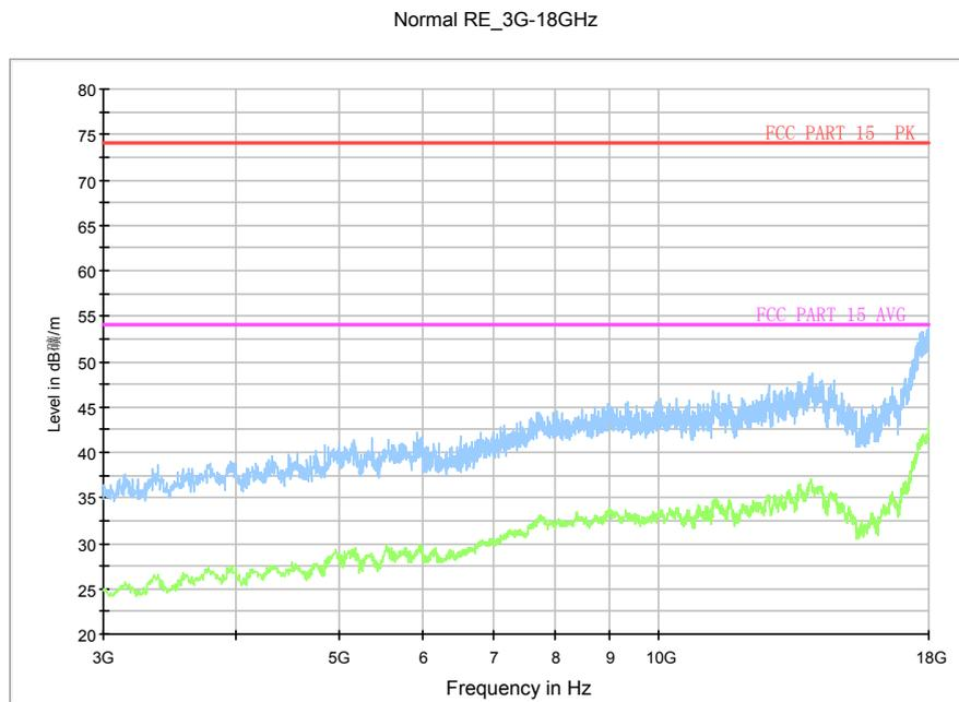
Fig.62. Radiated emission: GFSK, Channel 39, 3 GHz - 18 GHz
