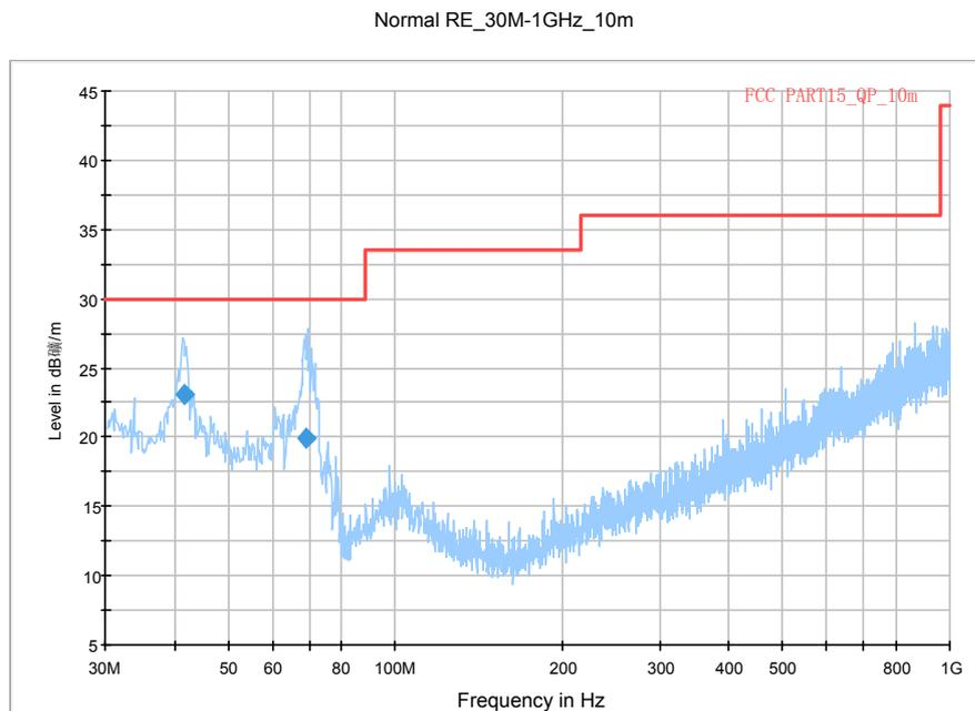
Fig.70. Radiated emission:  $\pi/4$  DQPSK, Channel 39, 30 MHz - 1 GHz
