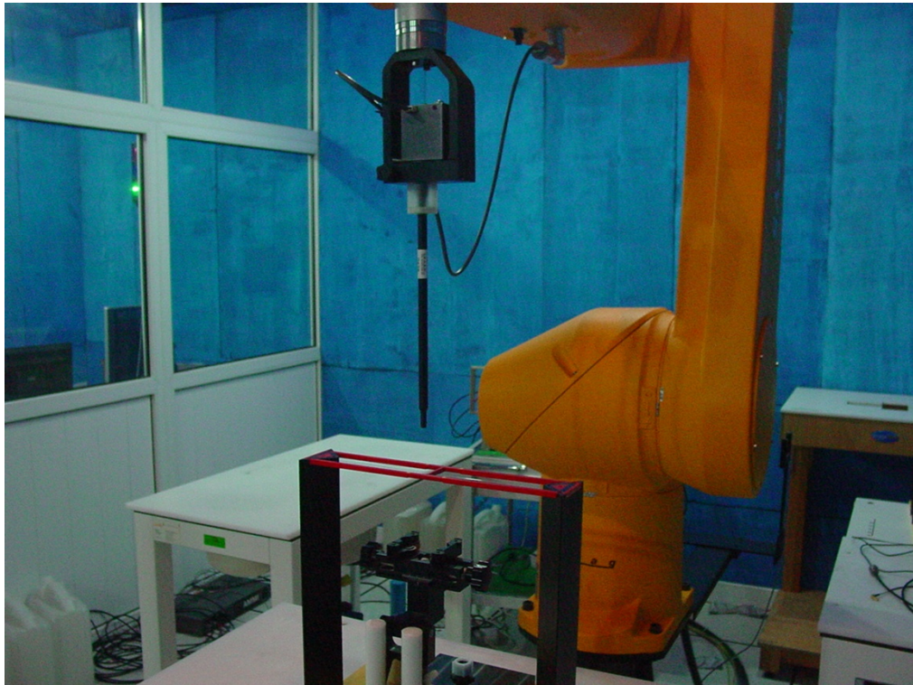
Picture A1: HAC RF System Layout
