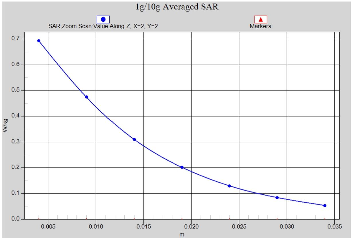
Fig. 7-1 Z-Scan at power reference point (WCDMA1900 CH9538)
