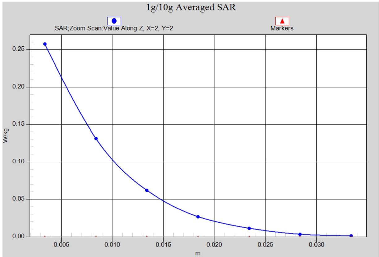
**Fig. 10-1 Z-Scan at power reference point (2450 MHz CH6)**
