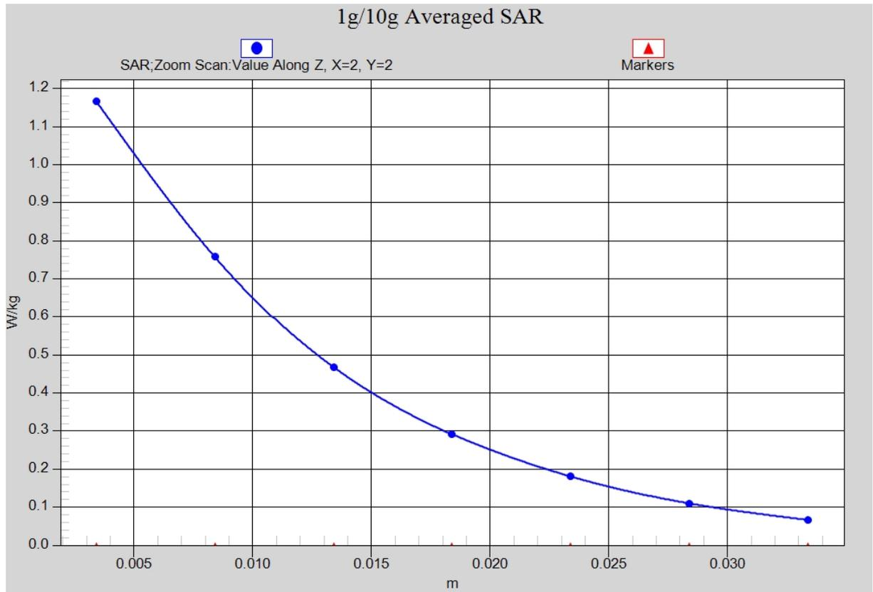
**Fig. 8-1 Z-Scan at power reference point (WCDMA1900 CH9262)**
