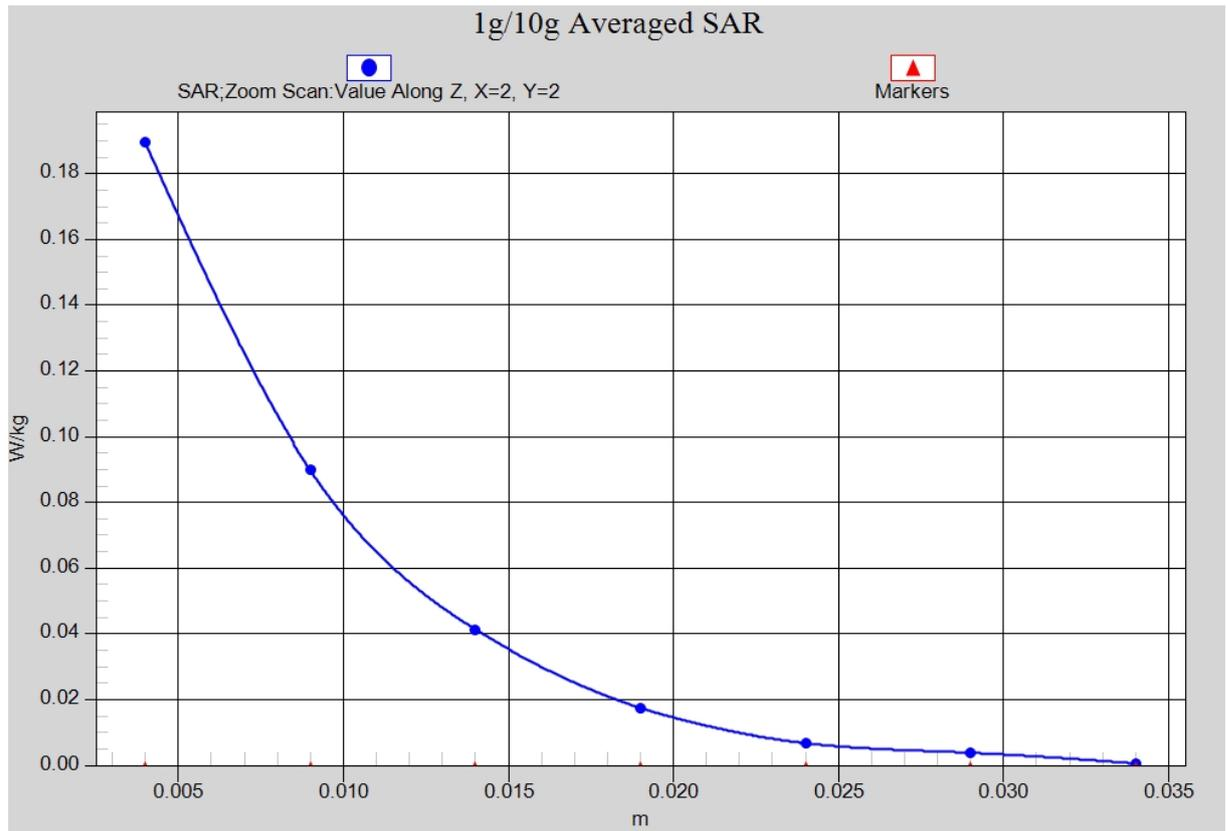
**Fig. 9-1 Z-Scan at power reference point (2450 MHz CH6)**
