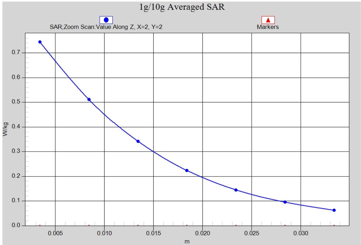
**Fig.4-1 Z-Scan at power reference point (1900 MHz CH512)**
