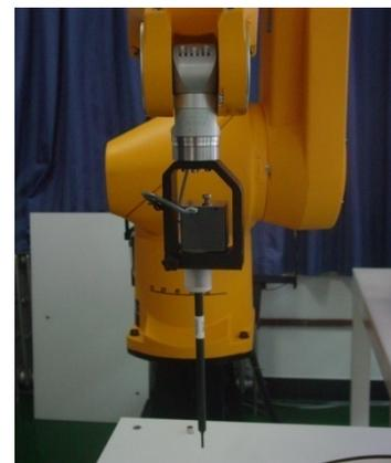
Picture C.3 E-field Probe
