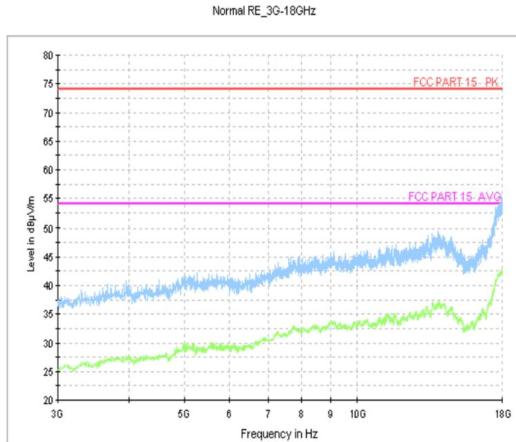
Fig.22. Radiated emission: GFSK, 2440MHz, 3 GHz - 18 GHz
