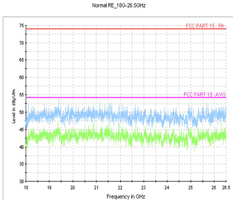
Fig.27. Radiated emission: GFSK, 18 GHz - 26 GHz
