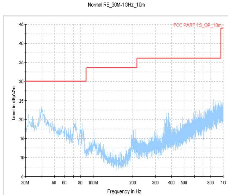
Fig.20. Radiated emission: GFSK, 2440MHz, 30 MHz - 1 GHz
