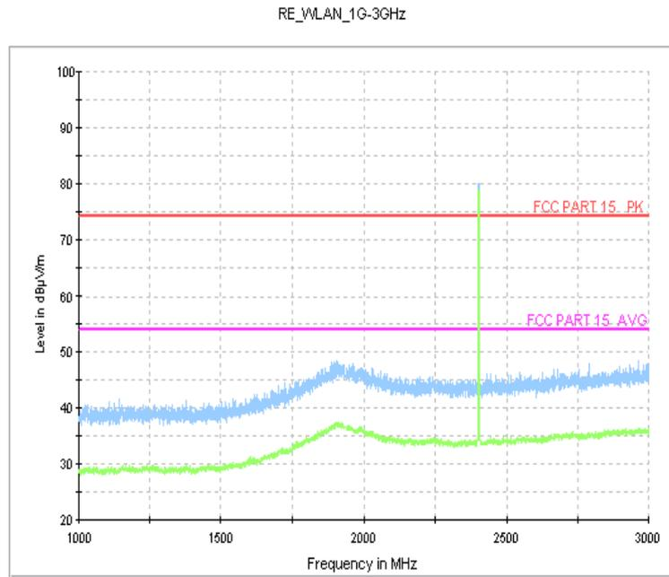
Fig.18. Radiated emission: GFSK, 2402MHz, 1 GHz - 3GHz
