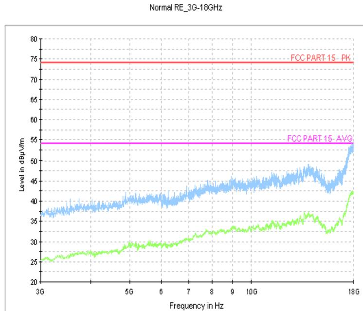
Fig.19. Radiated emission: GFSK, 2402MHz, 3 GHz - 18 GHz
