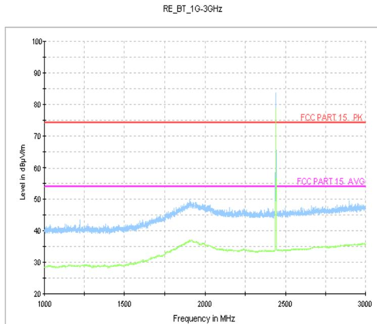
Fig.21. Radiated emission: GFSK, 2440MHz, 1 GHz - 3 GHz
