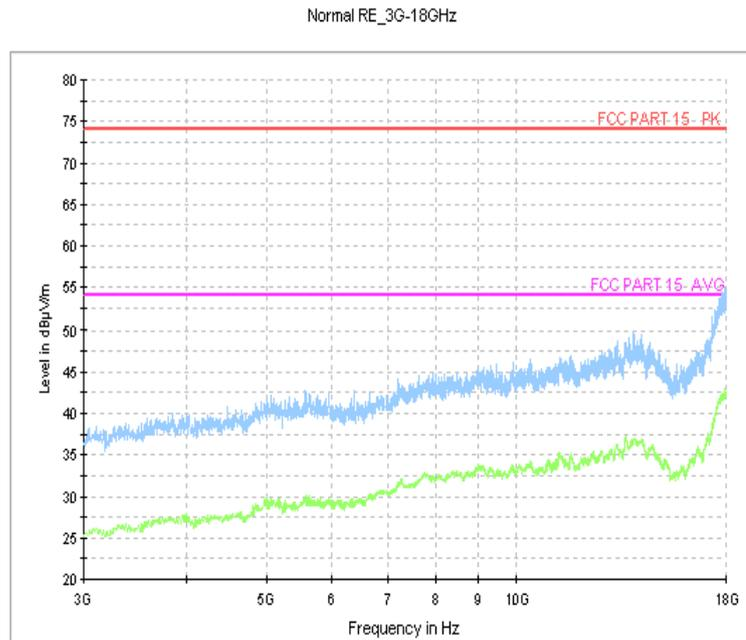
Fig.24. Radiated emission: GFSK, 2480MHz, 3 GHz - 18 GHz
