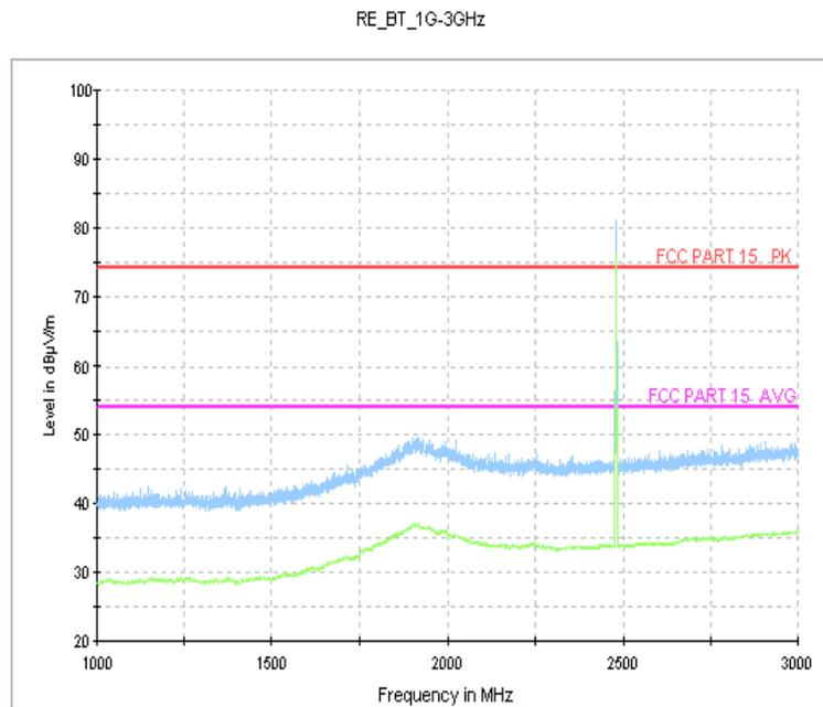
Fig.23. Radiated emission: GFSK, 2480MHz, 1 GHz - 3 GHz
