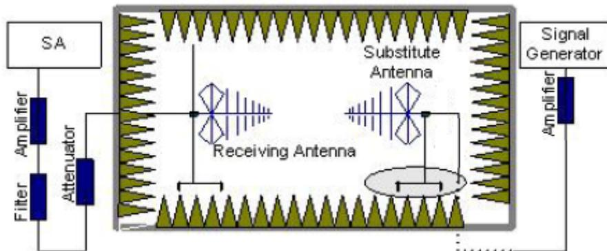
In the chamber, an substitution antenna for the frequency band of interest is placed at the reference point of the chamber. An RF Signal source for the frequency band of interest is
