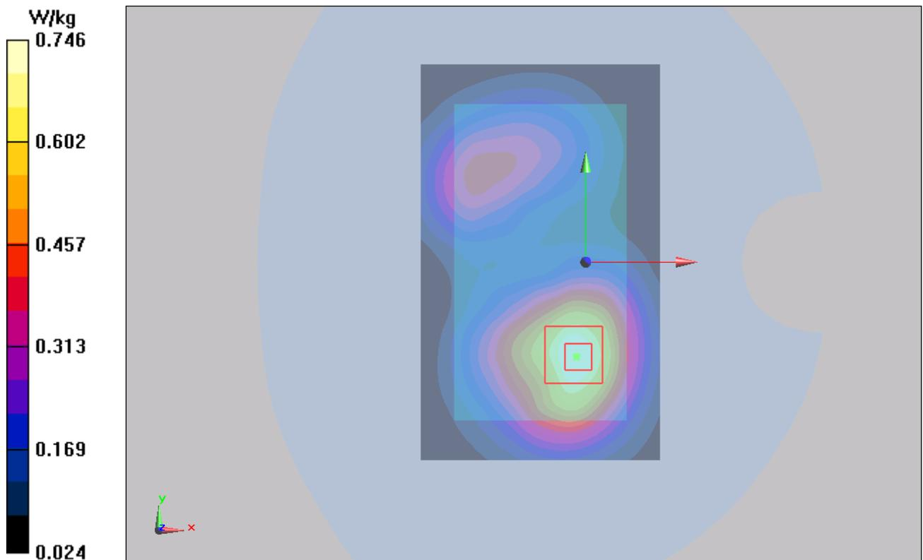
Figure 60 Body, Front Side, UMTS Band II Channel 9538
