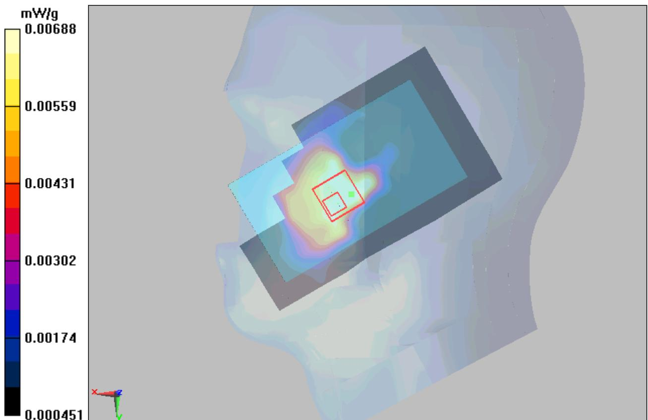
Figure 17 Right Hand Touch Cheek GSM 850 Channel 190
