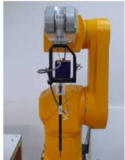
**Figure 3. EX3DV4 E-field probe**
