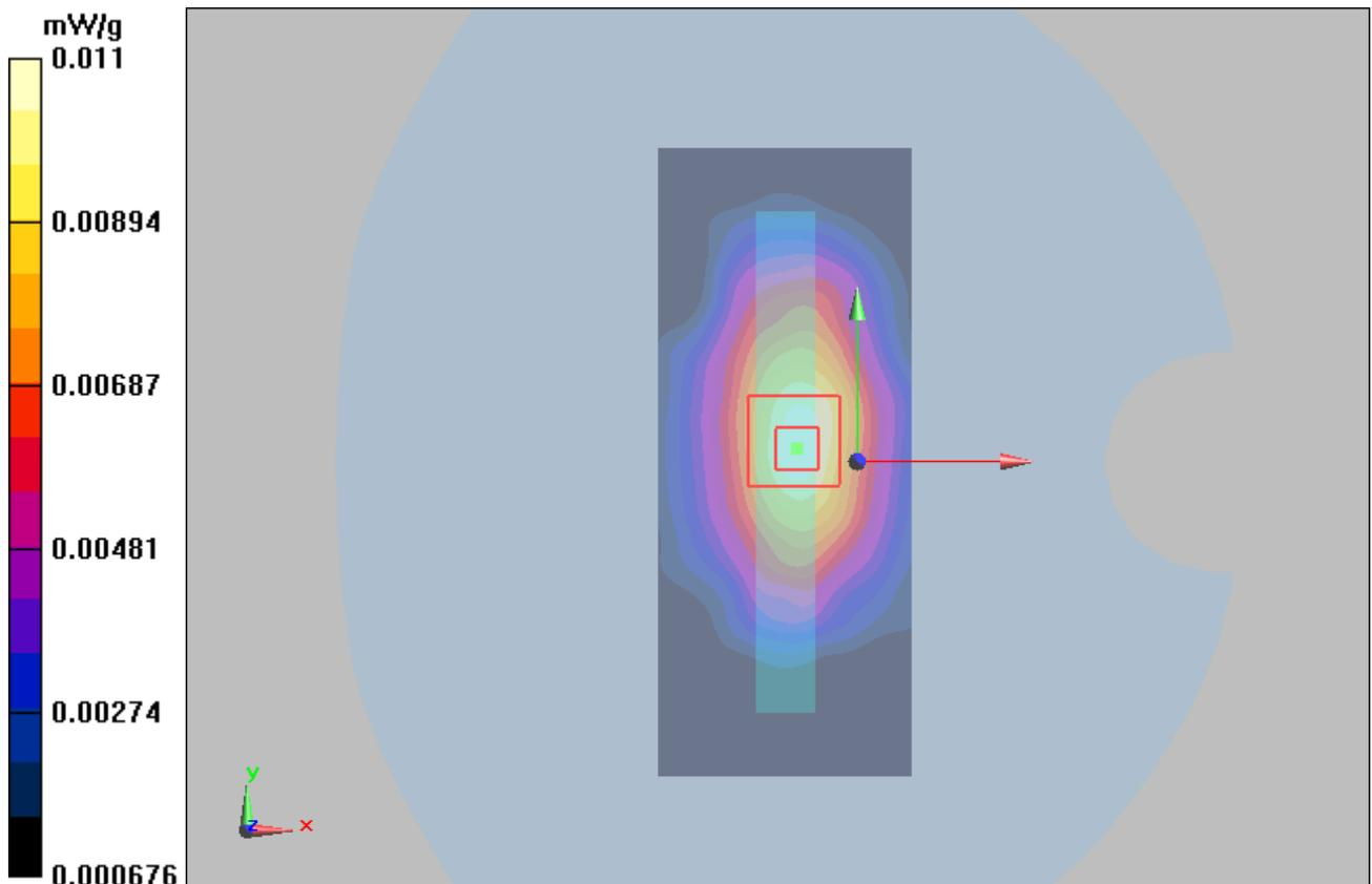
Figure 23 Body, Right Edge, GSM 850 GPRS (4Txslots) Channel 190
