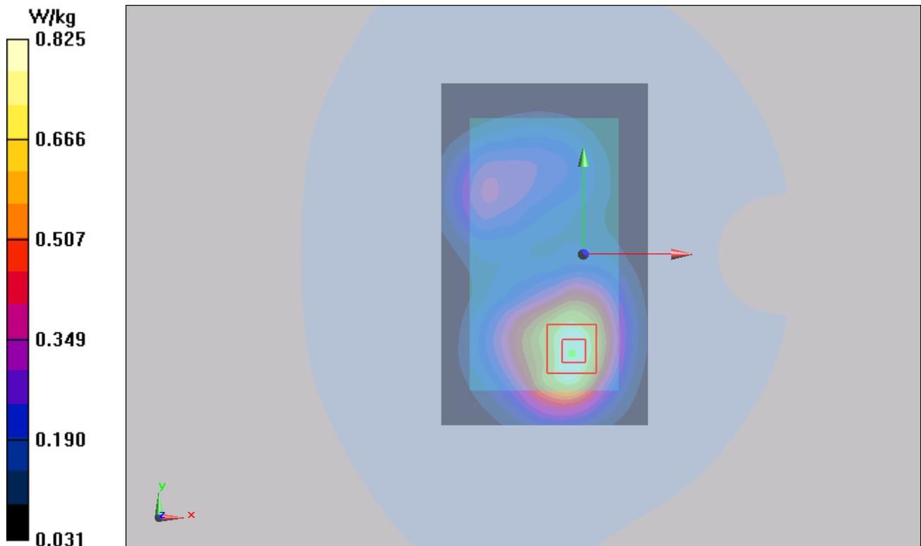
Figure 41 Body, Front Side, GSM 1900 GPRS (4Txslots) Channel 512
