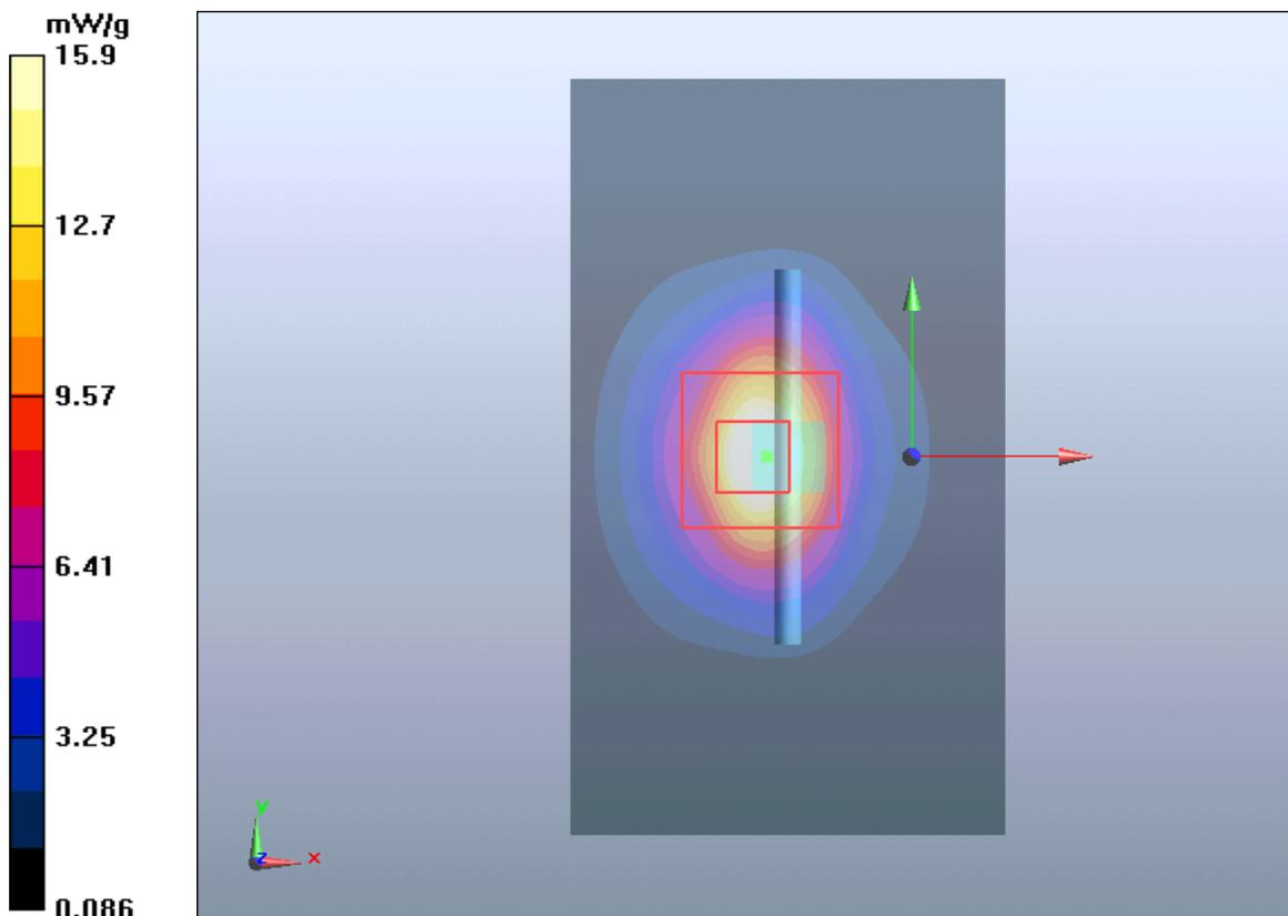
Figure 13 System Performance Check 2450MHz 250mW
