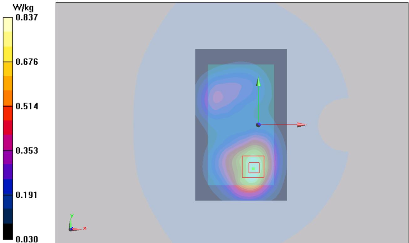
Figure 40 Body, Front Side, GSM 1900 GPRS (4Txslots) Channel 661
