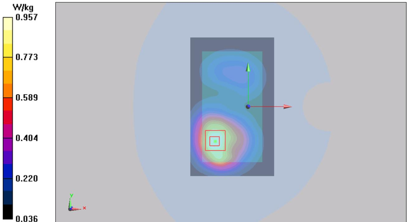
Figure 47 Body, Back Side, GSM 1900 GPRS (4Txslots) Channel 810
