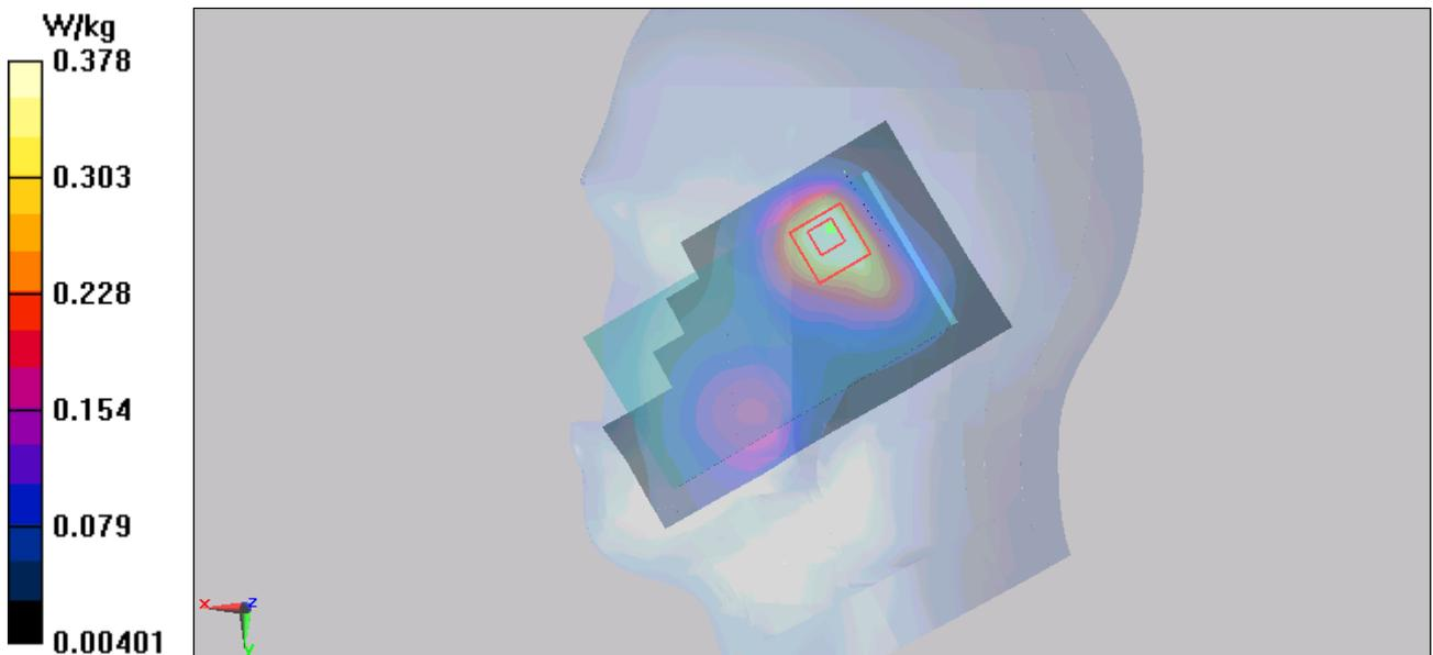
Figure 34 Right Hand Tilt 15° GSM 1900 Channel 661
