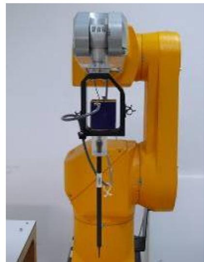
**Figure 3. EX3DV4 E-field probe**
