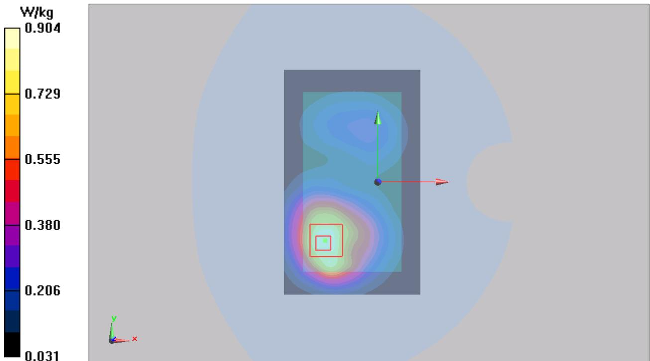
Figure 37 Body, Back Side, GSM 1900 GPRS (4Txslots) Channel 661
