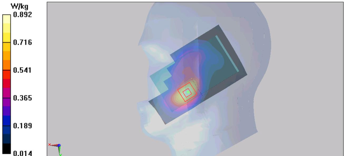
Figure 31 Right Hand Touch Cheek GSM 1900 Channel 810
