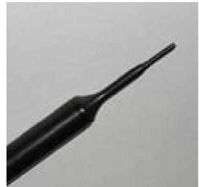
**Figure 2. EX3DV4 E-field Probe**
