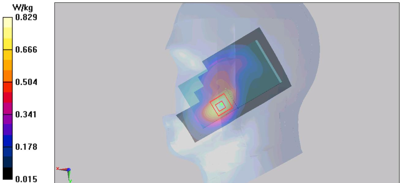
Figure 33 Right Hand Touch Cheek GSM 1900 Channel 512
