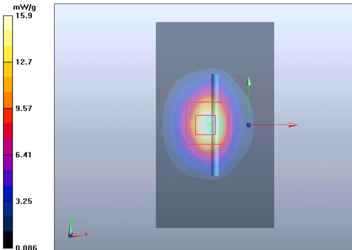
Figure 13 System Performance Check 2450MHz 250mW
