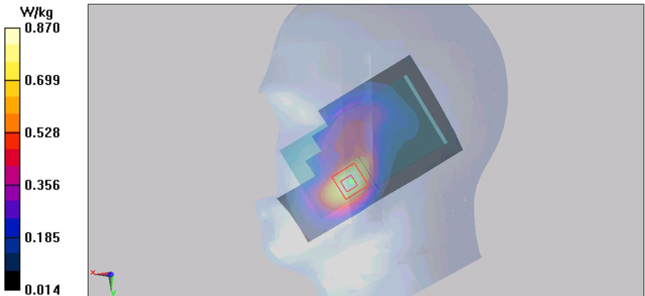
Figure 32 Right Hand Touch Cheek GSM 1900 Channel 661
