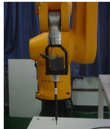
Picture C.3 E-field Probe
