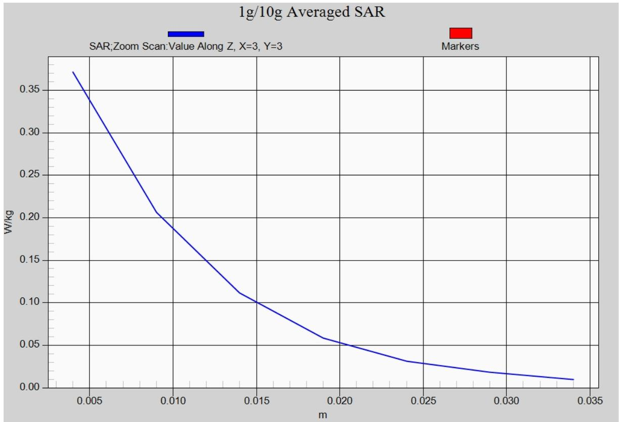
Fig. 9-1 Z-Scan at power reference point (2450 MHz CH1)
