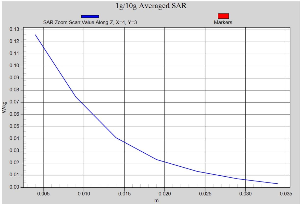
Fig. 10-1 Z-Scan at power reference point (2450 MHz CH1)
