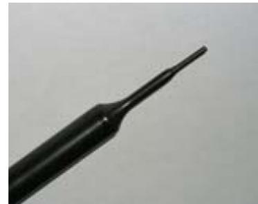
Picture C.2 Near-field Probe
