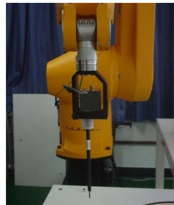
Picture C.3 E-field Probe
