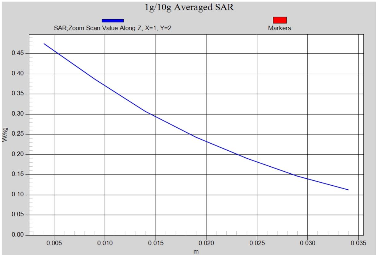
**Fig. 5-1 Z-Scan at power reference point (WCDMA 850 CH4233)**
