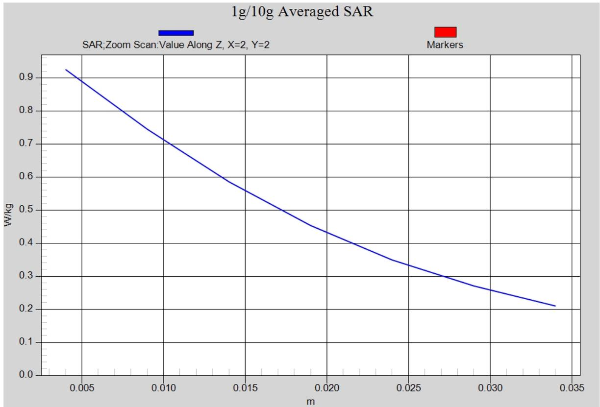
**Fig. 6-1 Z-Scan at power reference point (WCDMA850 CH4182)**
