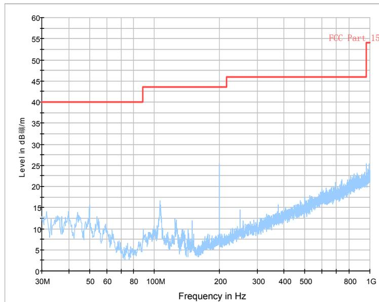
Fig.73. Radiated emission:  $\pi/4$  DQPSK, Channel 39, 30 MHz - 1 GHz
