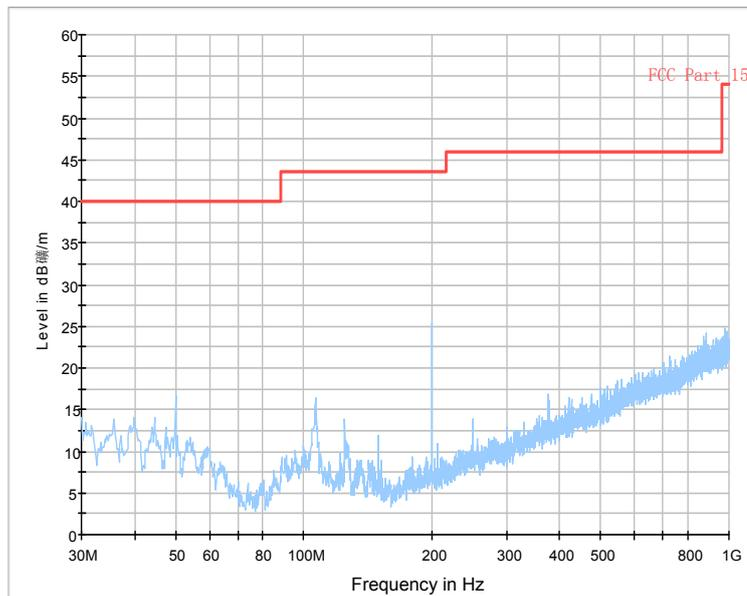
Fig.61. Radiated emission: GFSK, Channel 39, 30 MHz - 1 GHz
