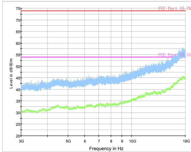
Fig.72. Radiated emission:  $\pi/4$  DQPSK, Channel 0, 3 GHz - 18 GHz
