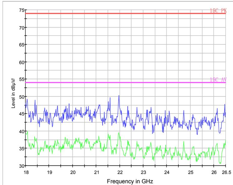
Fig.69. Radiated emission: GFSK, 18 GHz - 26 GHz
