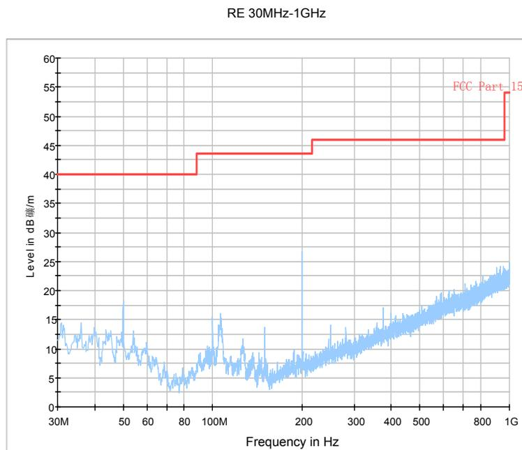
Fig.85. Radiated emission: 8DPSK, Channel 39, 30 MHz - 1 GHz
