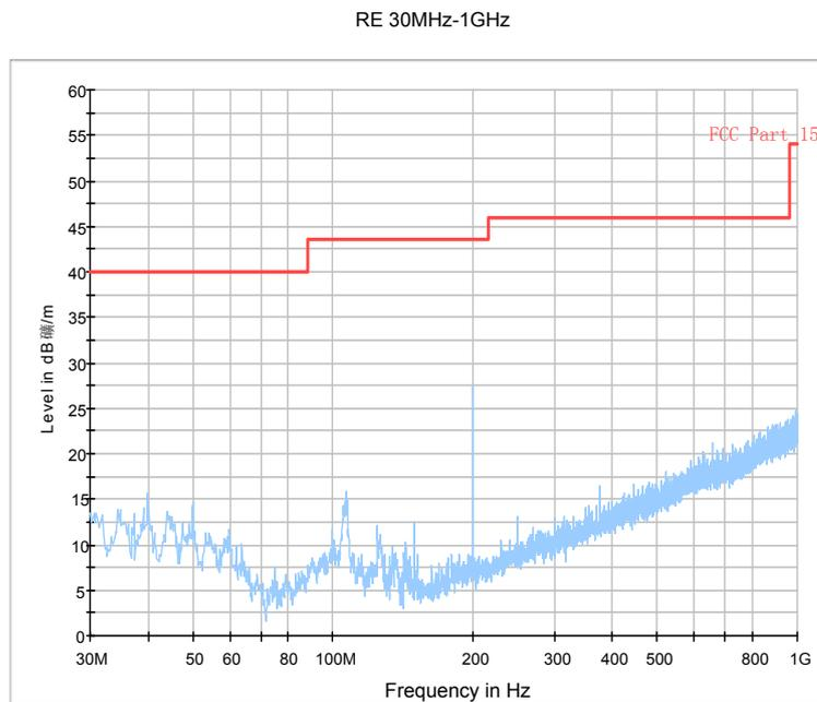
Fig.88. Radiated emission: 8DPSK, Channel 78, 30 MHz - 1 GHz
