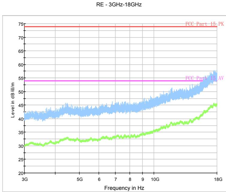
Fig.66. Radiated emission: GFSK, Channel 78, 3 GHz - 18 GHz
