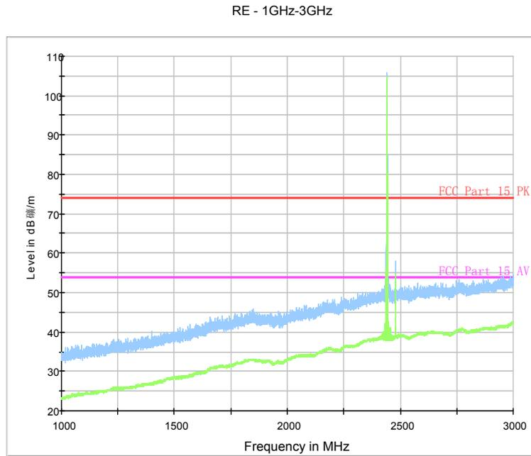
Fig.62. Radiated emission: GFSK, Channel 39, 1 GHz - 3 GHz
