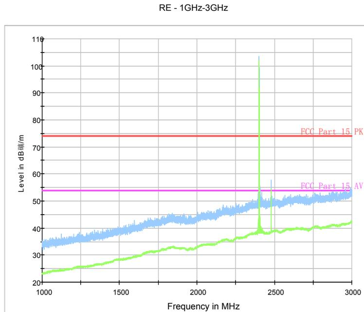
Fig.71. Radiated emission:  $\pi/4$  DQPSK, Channel 0, 1 GHz - 3 GHz
