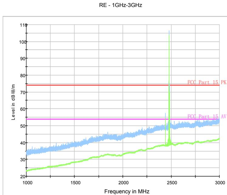
Fig.65. Fig.47 Radiated emission: GFSK, Channel 78, 1 GHz - 3 GHz
