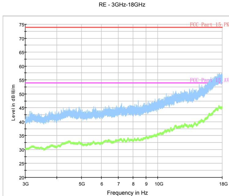
Fig.90. Radiated emission: 8DPSK, Channel 78, 3 GHz - 18 GHz
