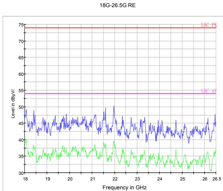
Fig.93. Radiated emission: 8DPSK, 18 GHz - 26 GHz
