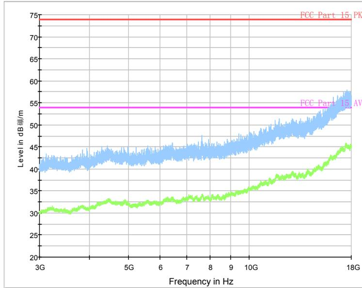
Fig.60. Radiated emission: GFSK, Channel 0, 3 GHz - 18 GHz
