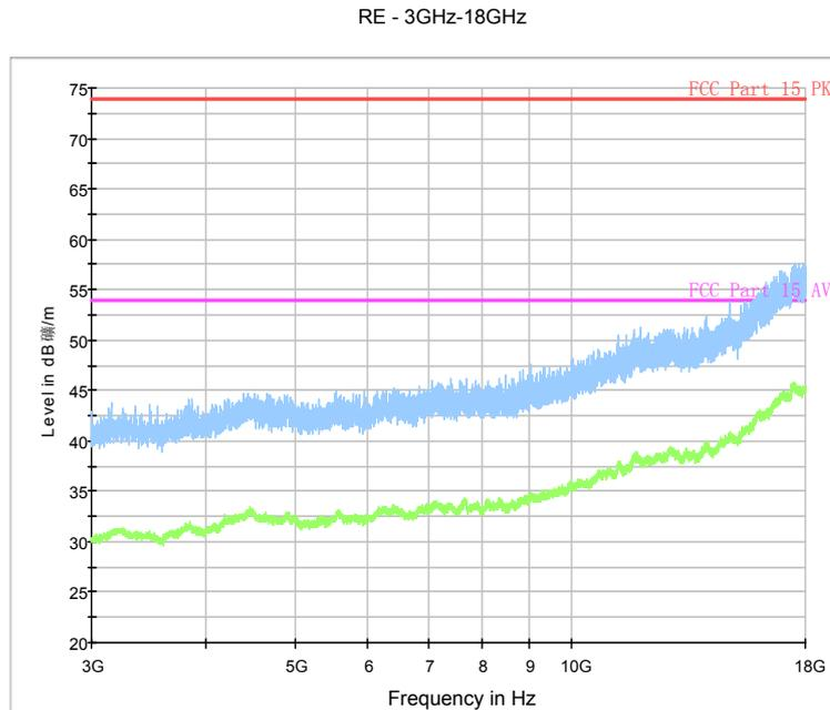
Fig.78. Radiated emission:  $\pi/4$  DQPSK, Channel 78, 3 GHz - 18 GHz
