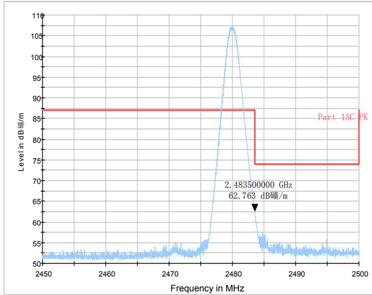
Fig.68. Radiated emission (Power) GFSK, high channel
