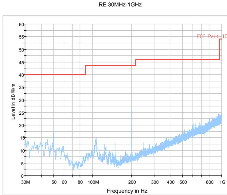
Fig.82. Radiated emission: 8DPSK, Channel 0, 30 MHz - 1 GHz
