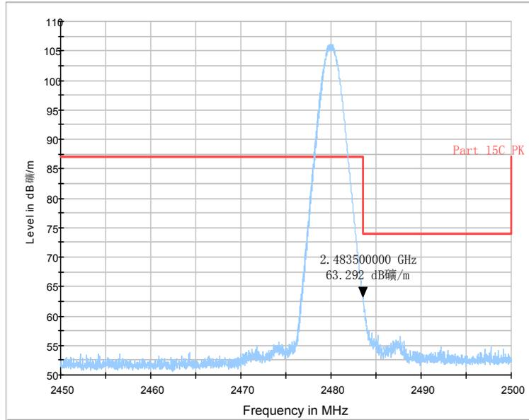
Fig.80. Radiated emission (Power):  $\pi/4$  DQPSK, high channel
