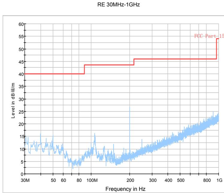
Fig.70. Radiated emission:  $\pi/4$  DQPSK, Channel 0, 30 MHz - 1 GHz
