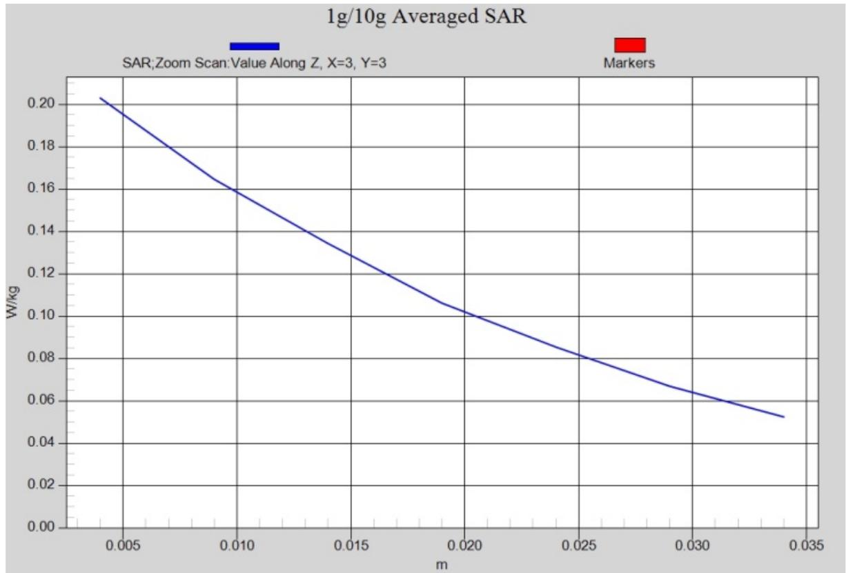
**Fig. 1-1 Z-Scan at power reference point (850 MHz CH190)**
