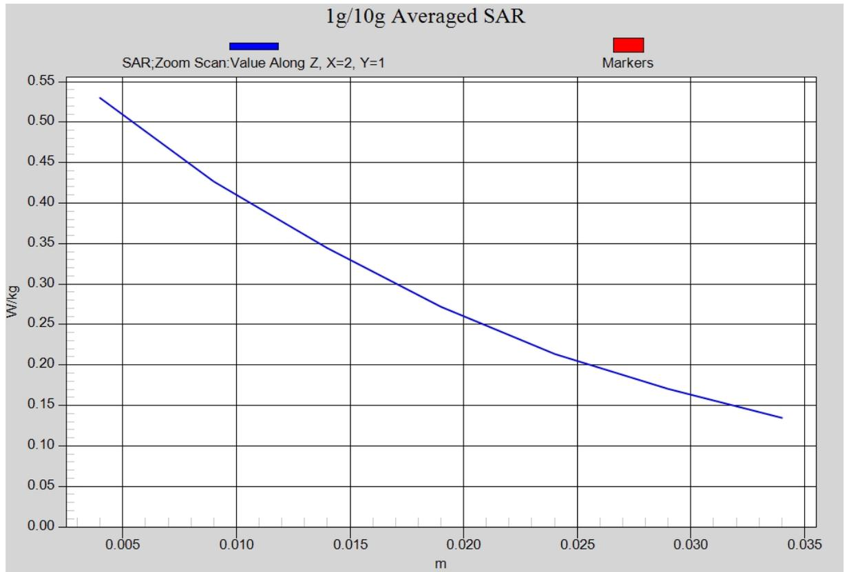
**Fig. 6-1 Z-Scan at power reference point (WCDMA850 CH4132)**
