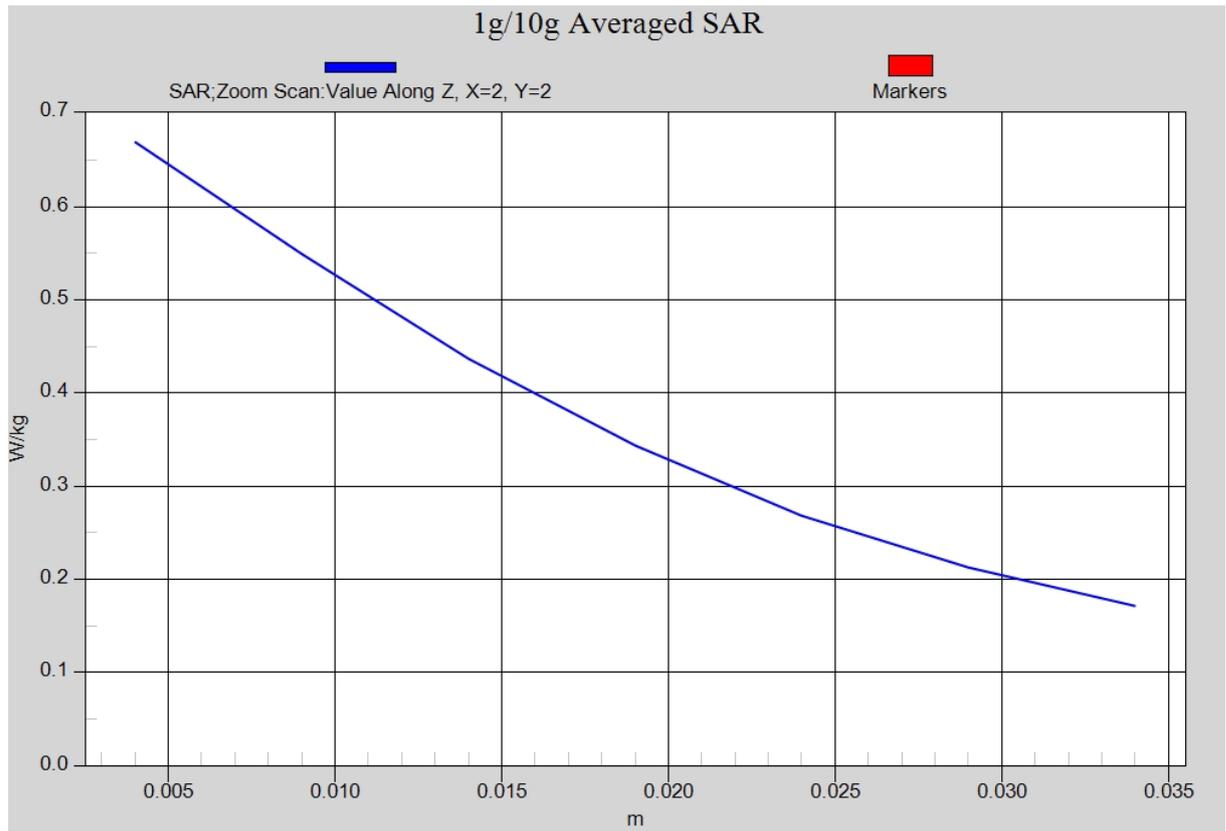
Fig. 2-1 Z-Scan at power reference point (850 MHz CH128)
