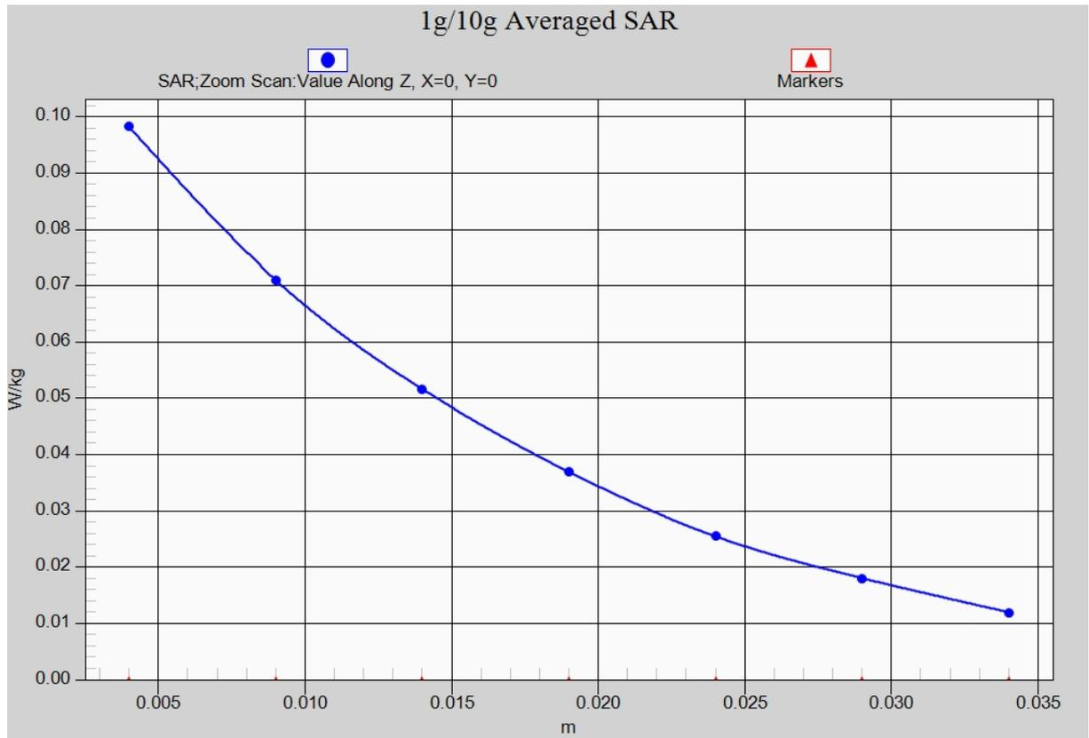
Fig. 7-1 Z-Scan at power reference point (WCDMA1900 CH9400)
