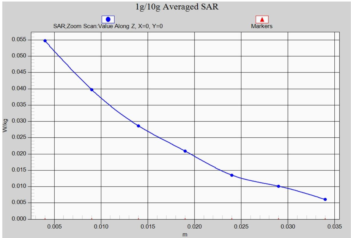
Fig. 3-1 Z-Scan at power reference point (1900 MHz CH810)
