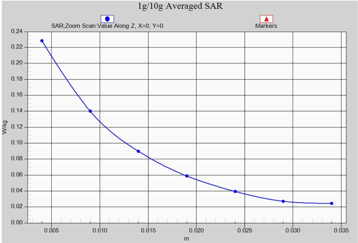
Fig.4-1 Z-Scan at power reference point (1900 MHz CH810)
