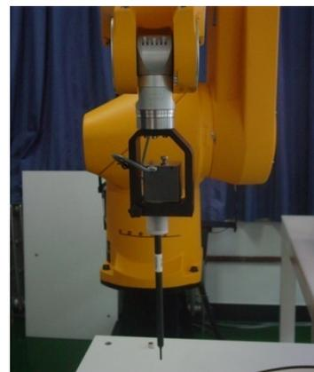
Picture C.3 E-field Probe
