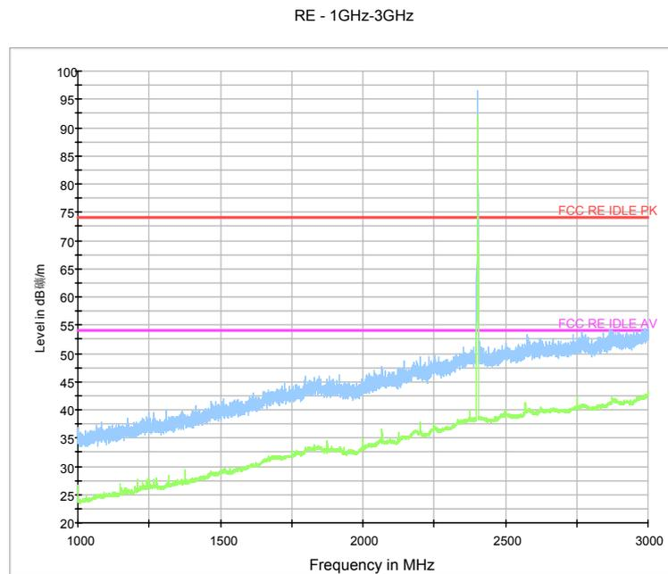
Fig.19. Radiated emission: GFSK, 2402MHz, 1 GHz - 3GHz
