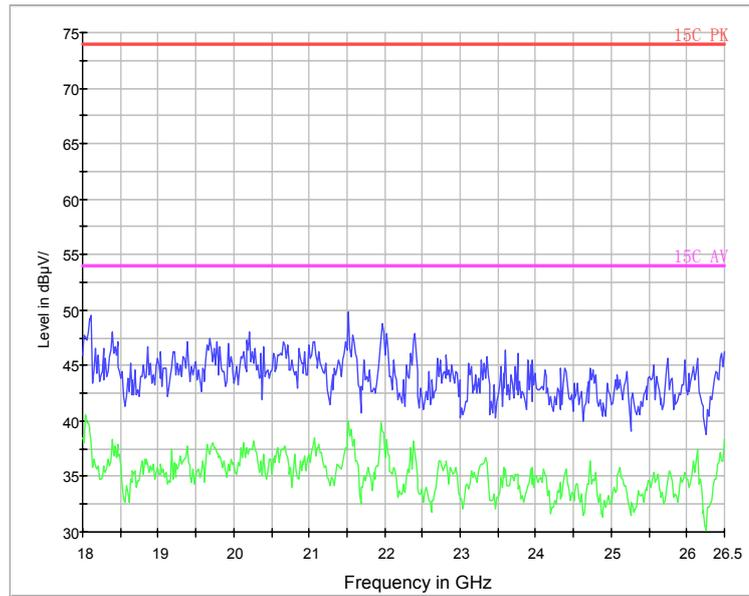
Fig.29. Radiated emission: GFSK, 18 GHz - 26 GHz
