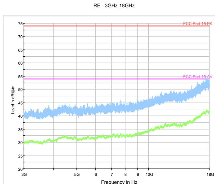
Fig.20. Radiated emission: GFSK, 2402MHz, 3 GHz - 18 GHz
