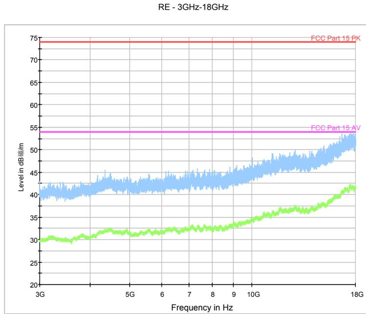
Fig.23. Radiated emission: GFSK, 2440MHz, 3 GHz - 18 GHz
