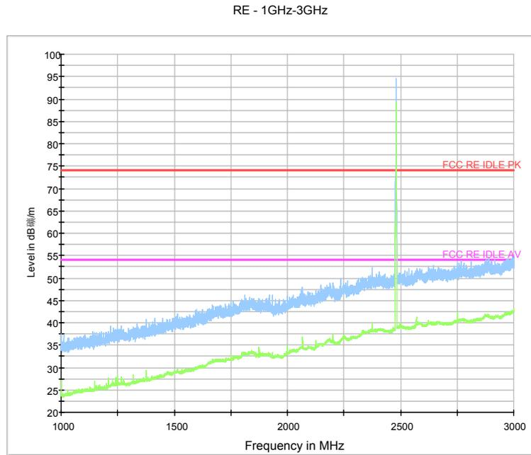
Fig.25. Radiated emission: GFSK, 2480MHz, 1 GHz - 3 GHz
