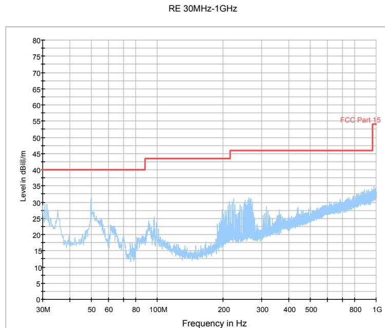
Fig.18. Radiated emission: GFSK, 2402MHz, 30 MHz - 1 GHz
