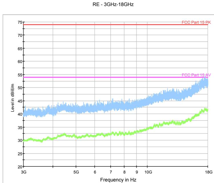
Fig.26. Radiated emission: GFSK, 2480MHz, 3 GHz - 18 GHz
