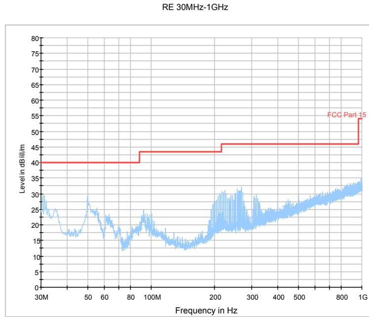
Fig.21. Radiated emission: GFSK, 2440MHz, 30 MHz - 1 GHz
