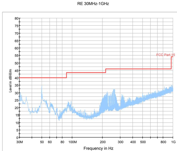
Fig.24. Radiated emission: GFSK, 2480MHz, 30 MHz - 1 GHz
