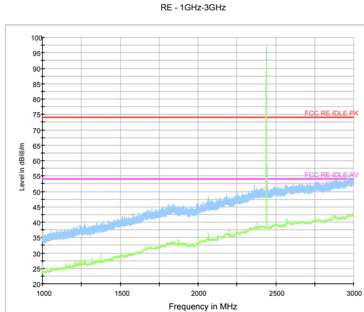
Fig.22. Radiated emission: GFSK, 2440MHz, 1 GHz - 3 GHz
