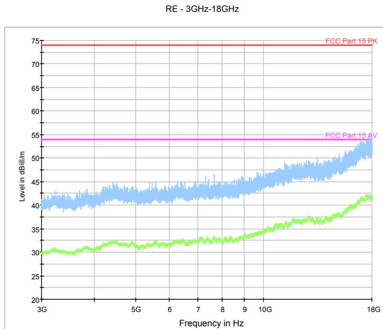
Fig.84. Radiated emission: 8DPSK, Channel 0, 3 GHz - 18 GHz
