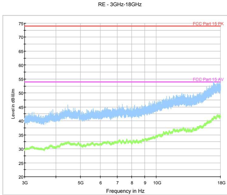
Fig.63. Radiated emission: GFSK, Channel 39, 3 GHz - 18 GHz
