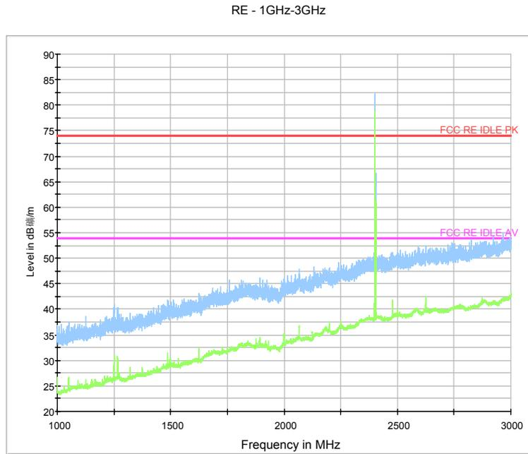
Fig.83. Radiated emission: 8DPSK, Channel 0, 1 GHz - 3 GHz
