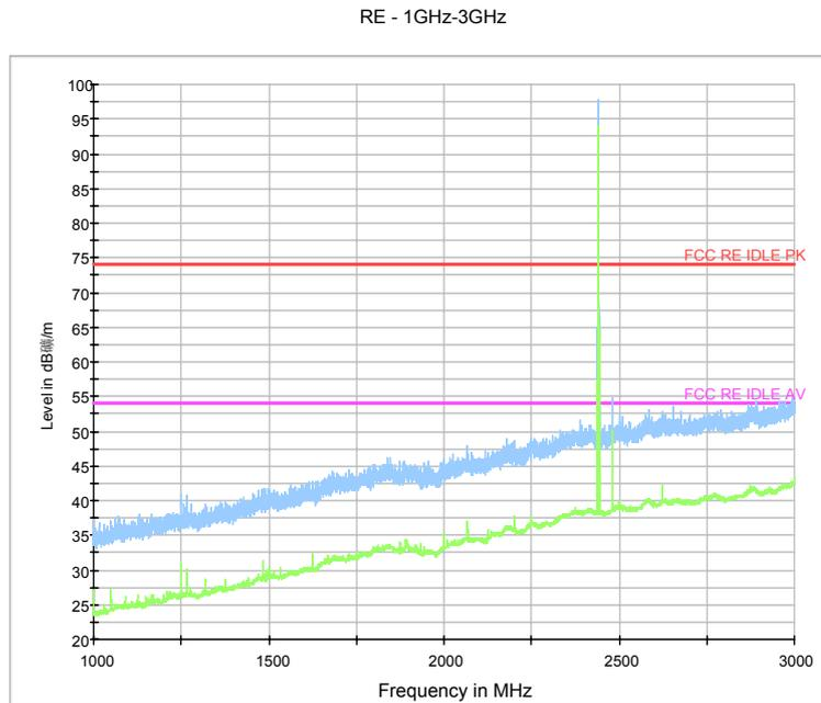
Fig.74. Radiated emission:  $\pi/4$  DQPSK, Channel 39, 1 GHz - 3 GHz
