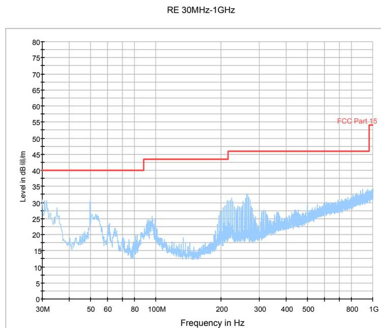
Fig.58. Radiated emission: GFSK, Channel 0, 30 MHz - 1 GHz
