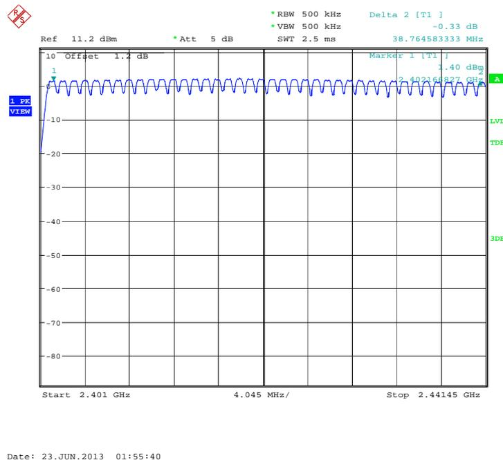
Fig.124. Number of hopping frequencies: GFSK, Channel 0 - 39
