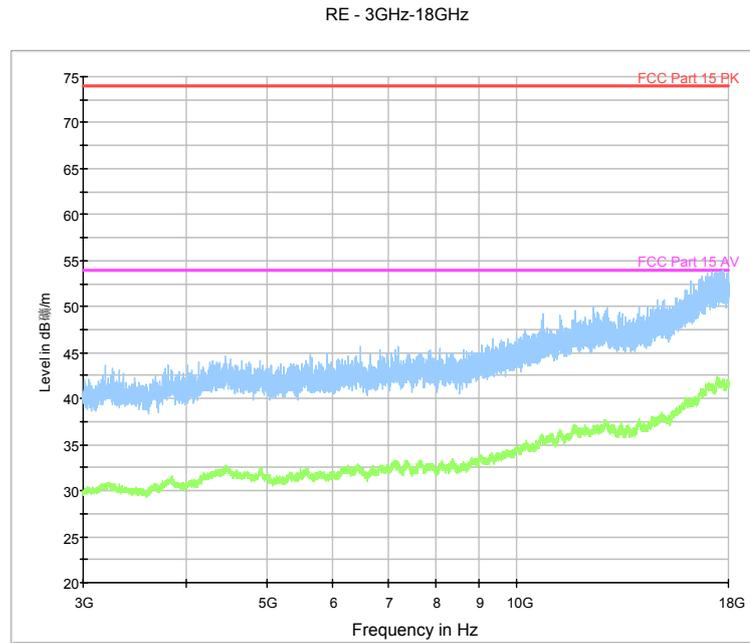
Fig.87. Radiated emission: 8DPSK, Channel 39, 3 GHz - 18 GHz
