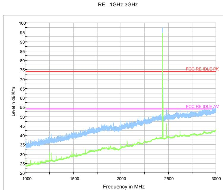
Fig.86. Radiated emission: 8DPSK, Channel 39, 1 GHz - 3 GHz
