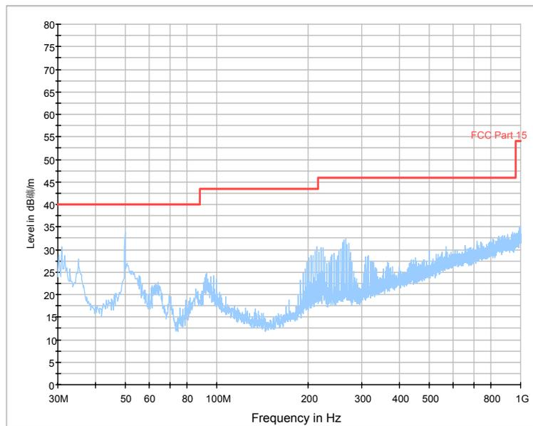
Fig.70. Radiated emission:  $\pi/4$  DQPSK, Channel 0, 30 MHz - 1 GHz
