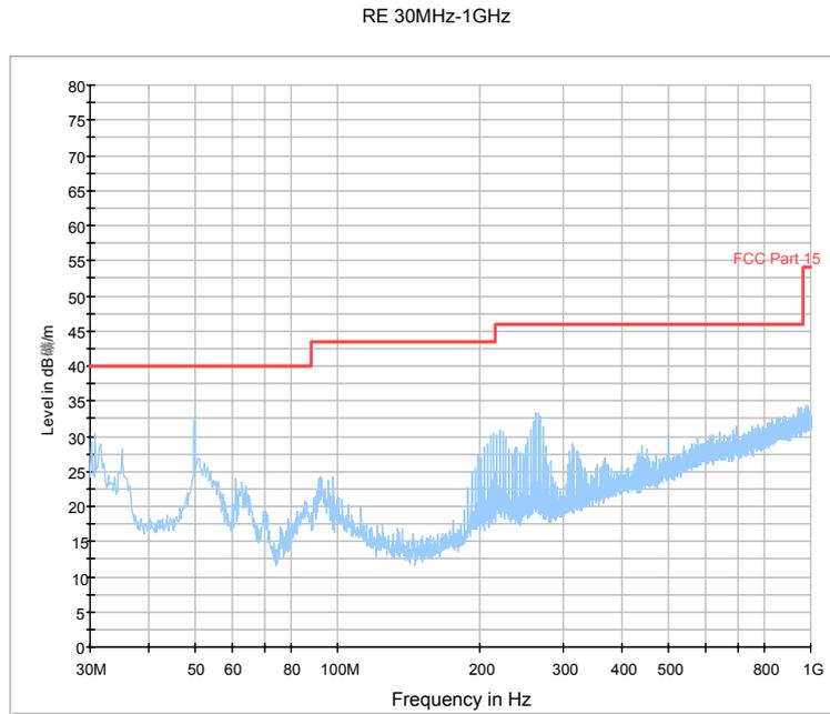
Fig.73. Radiated emission:  $\pi/4$  DQPSK, Channel 39, 30 MHz - 1 GHz
