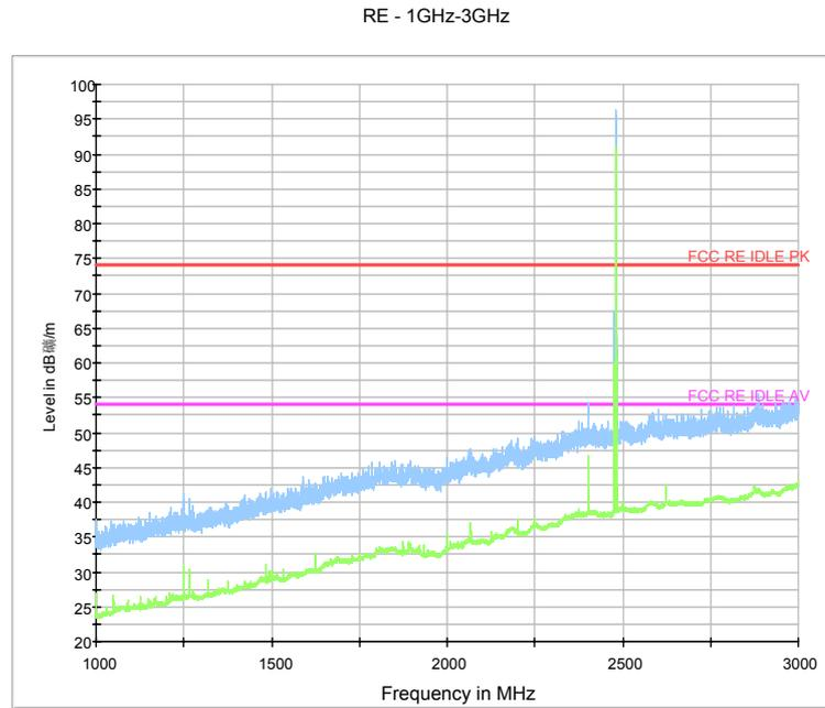
Fig.77. Radiated emission:  $\pi/4$  DQPSK, Channel 78, 1 GHz - 3 GHz
