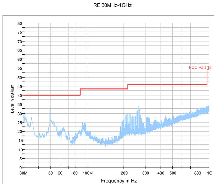
Fig.64. Radiated emission: GFSK, Channel 78, 30 MHz - 1 GHz
