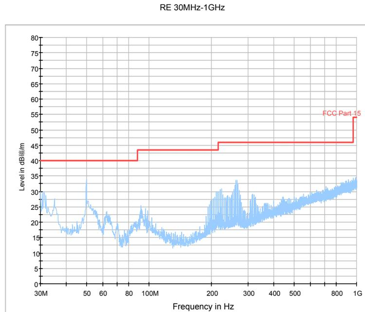
Fig.76. Radiated emission:  $\pi/4$  DQPSK, Channel 78, 30 MHz - 1 GHz
