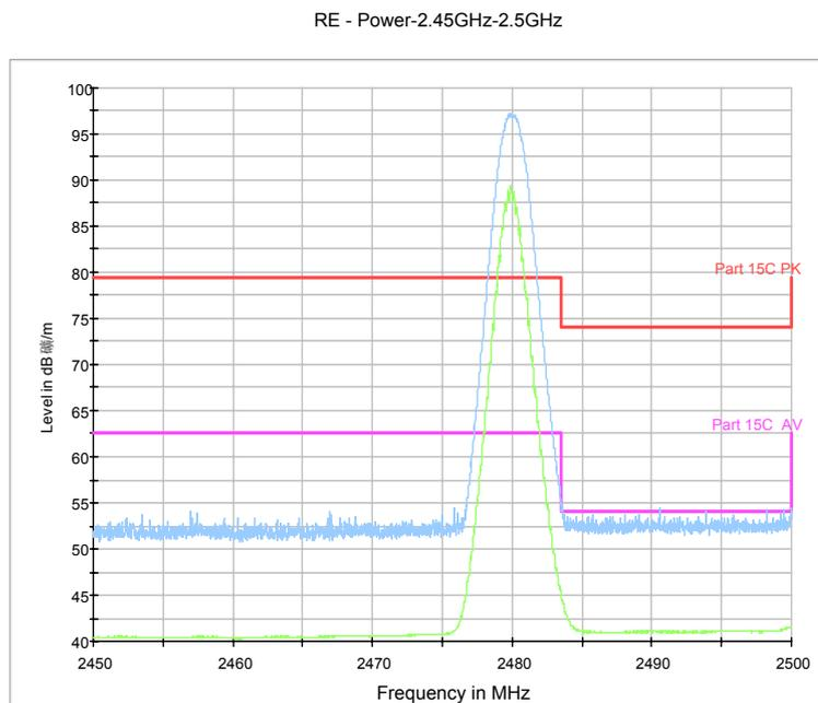
Fig.80. Radiated emission (Power):  $\pi/4$  DQPSK, high channel
