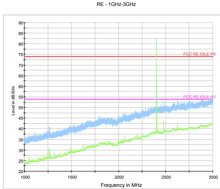
Fig.59. Radiated emission: GFSK, Channel 0, 1 GHz - 3 GHz
