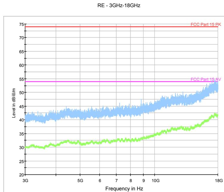
Fig.60. Radiated emission: GFSK, Channel 0, 3 GHz - 18 GHz
