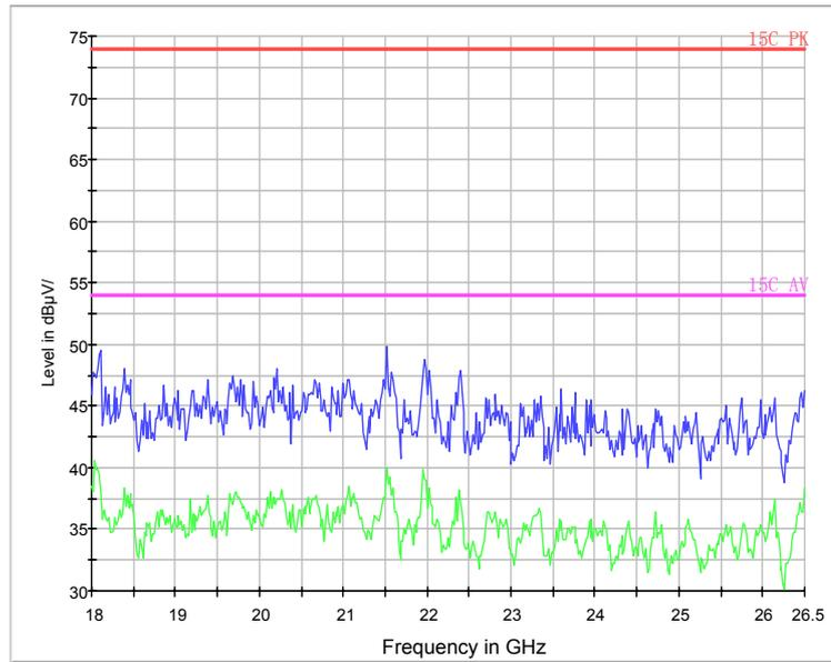
Fig.93. Radiated emission: 8DPSK, 18 GHz - 26 GHz
