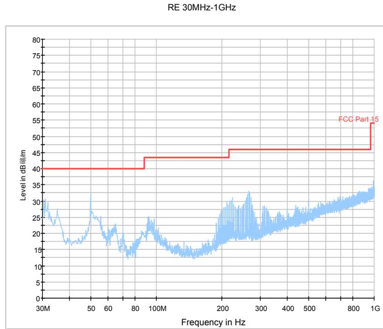
Fig.61. Radiated emission: GFSK, Channel 39, 30 MHz - 1 GHz
