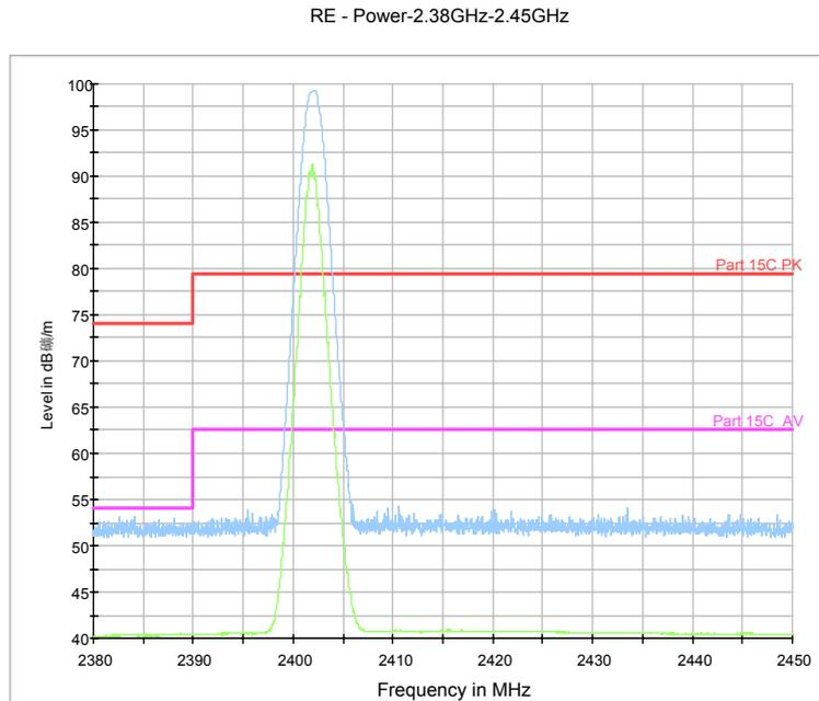
Fig.79. Radiated emission (Power):  $\pi/4$  DQPSK, low channel
