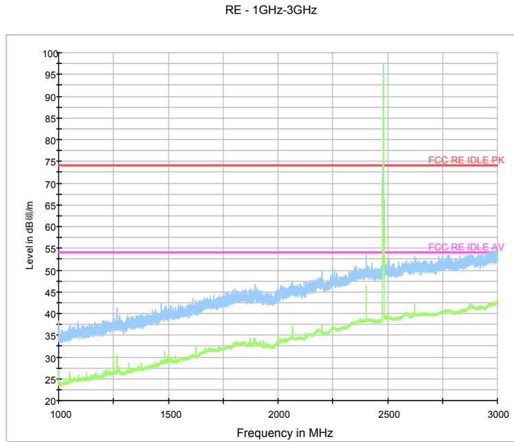
Fig.89. Radiated emission: 8DPSK, Channel 78, 1 GHz - 3 GHz
