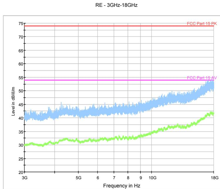
Fig.72. Radiated emission:  $\pi/4$  DQPSK, Channel 0, 3 GHz - 18 GHz
