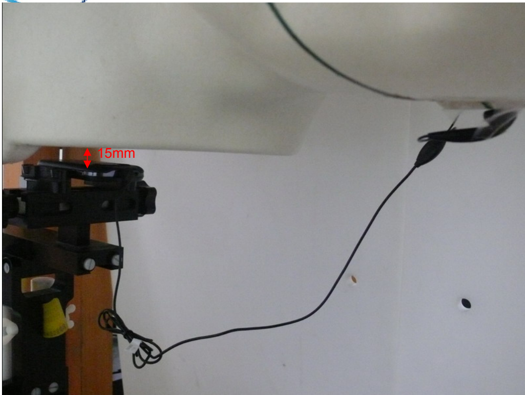
Picture 15: Body with earphone, The EUT display towards ground, the distance from handset to the bottom of the Phantom is 15mm
