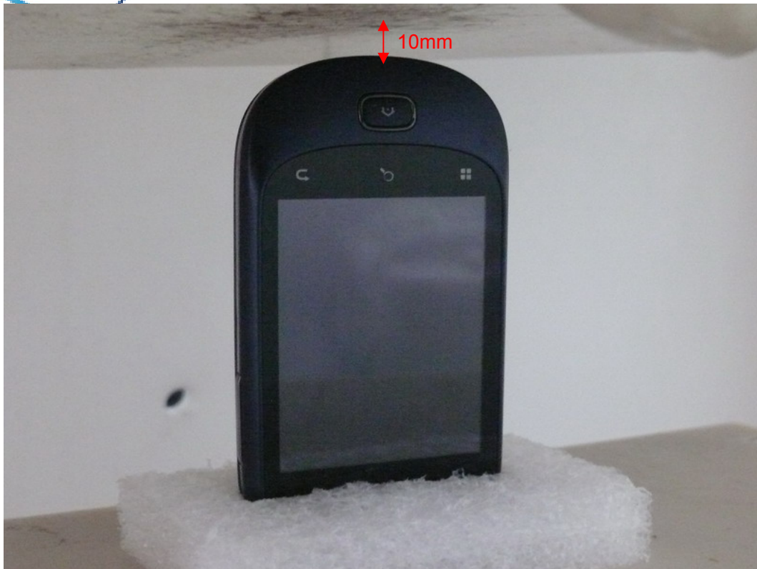
Picture 21: Bottom edge, the distance from handset to the bottom of the Phantom is 10mm
