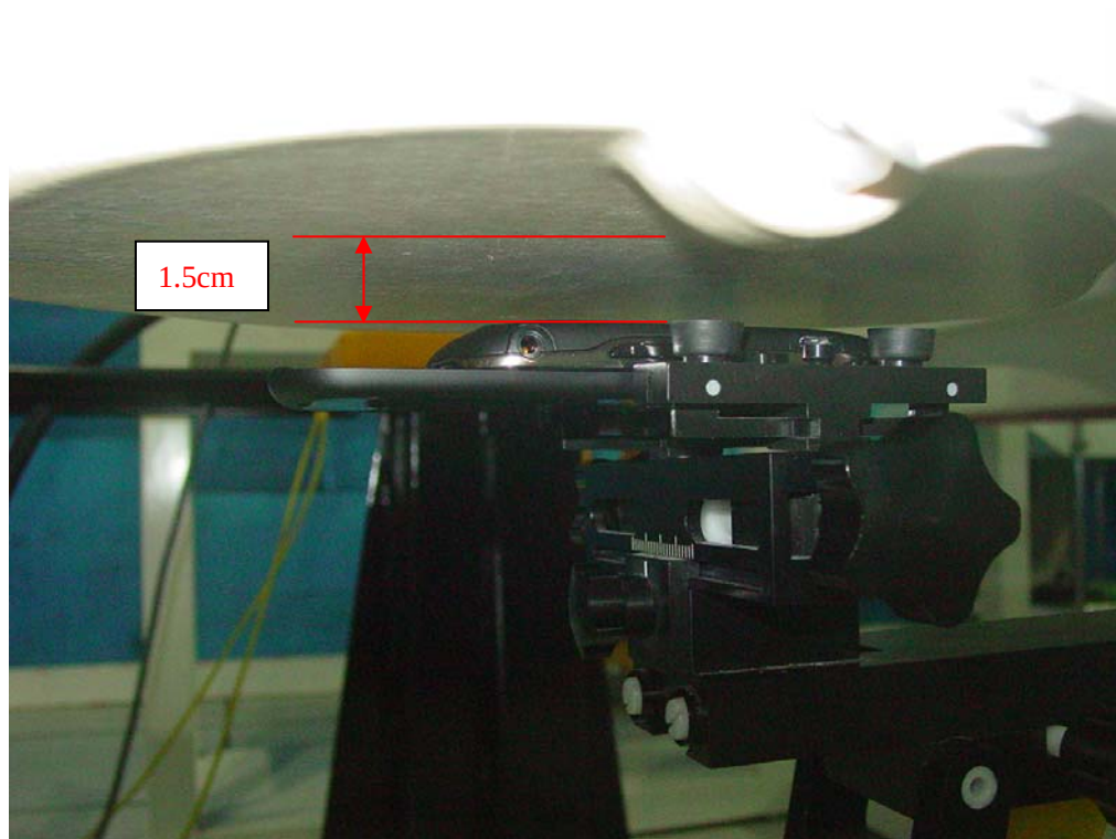
Picture B15: Body-worn Position (towards ground, the distance from handset to the bottom of the Phantom is 1.5cm) – Slide up
