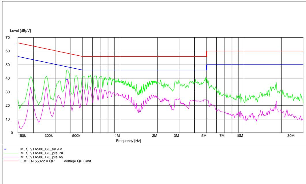
Fig. 34 AC Powerline Conducted Emission with charger 1
