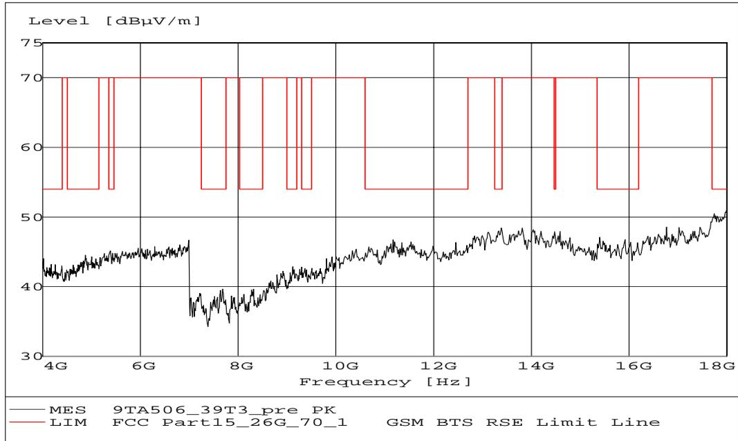
Fig. 19 Radiated emission: Channel 39, 4 GHz - 18 GHz
