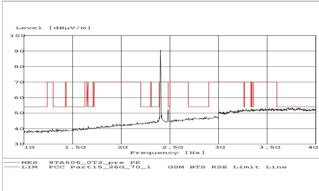
Fig. 15 Radiated emission: Channel 0, 1 GHz - 4 GHz
