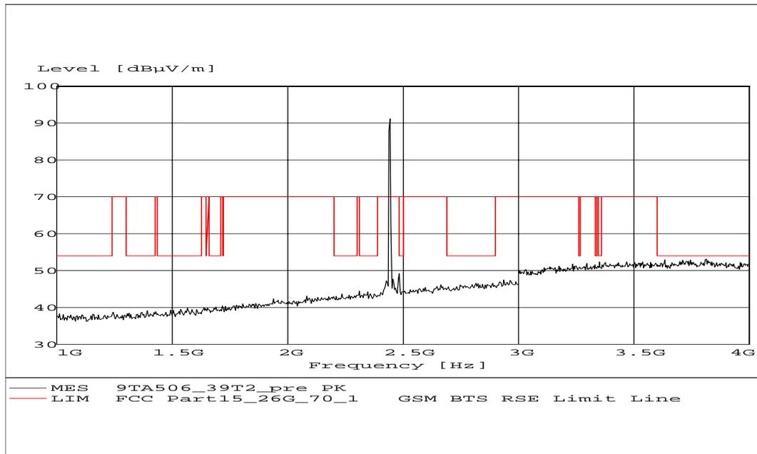
Fig. 18 Radiated emission: Channel 39, 1 GHz - 4 GHz
