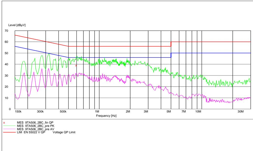
**Fig. 35 AC Powerline Conducted Emission with charger 2**
