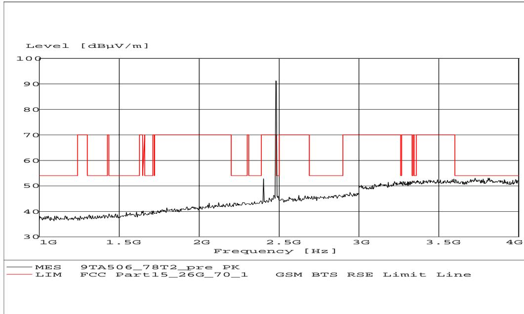
Fig. 21 Radiated emission: Channel 78, 1 GHz - 4 GHz
