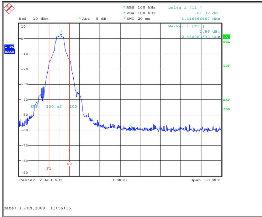
Fig. 3 Frequency Band Edges: Channel 78, Hopping Off
