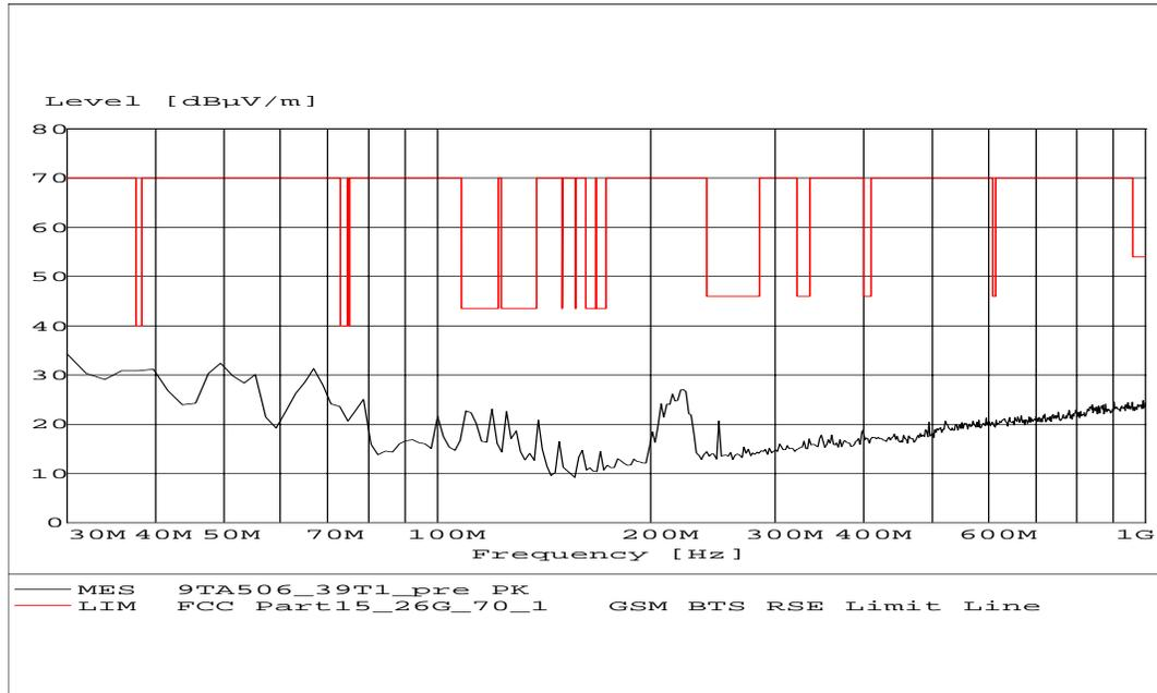
Fig. 17 Radiated emission: Channel 39, 30 MHz - 1 GHz
