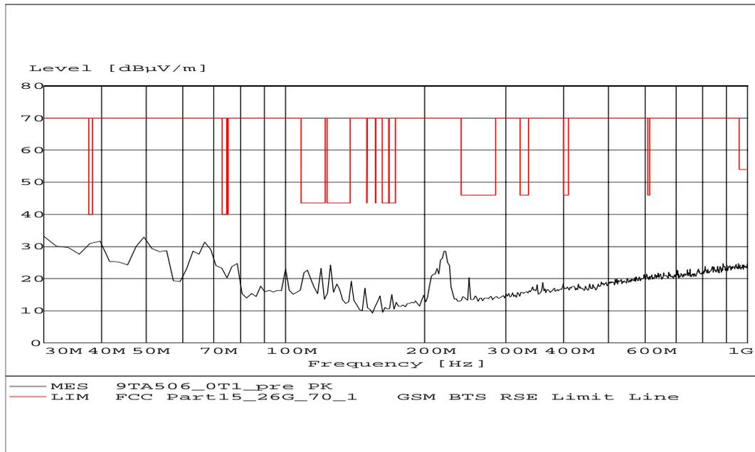
Fig. 14 Radiated emission: Channel 0, 30 MHz - 1 GHz
