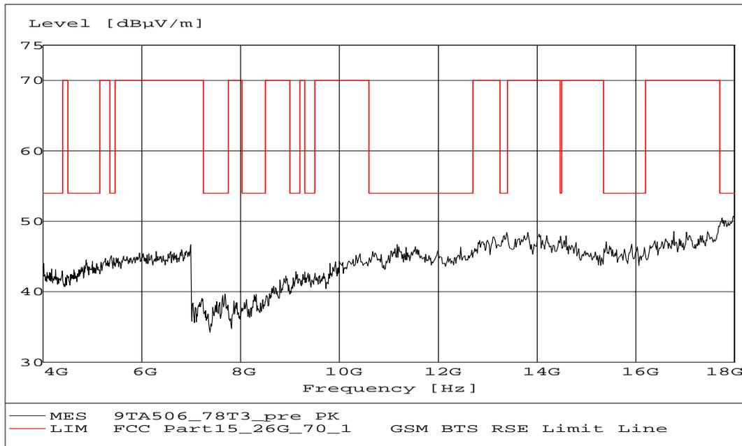
Fig. 22 Radiated emission: Channel 78, 4 GHz - 18 GHz
