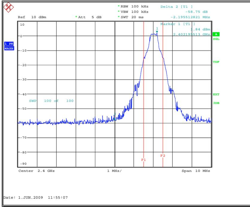
Fig. 1 Frequency Band Edges: Channel 0, Hopping Off
