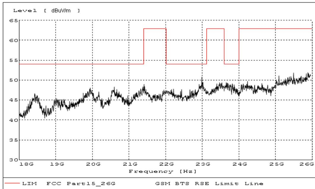
Fig. 24 Radiated emission: 18 GHz - 26 GHz
