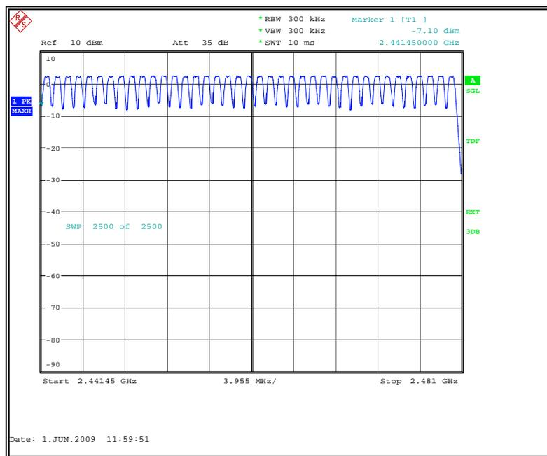
Fig. 33 Number of hopping frequencies: Channel 40 - 78
