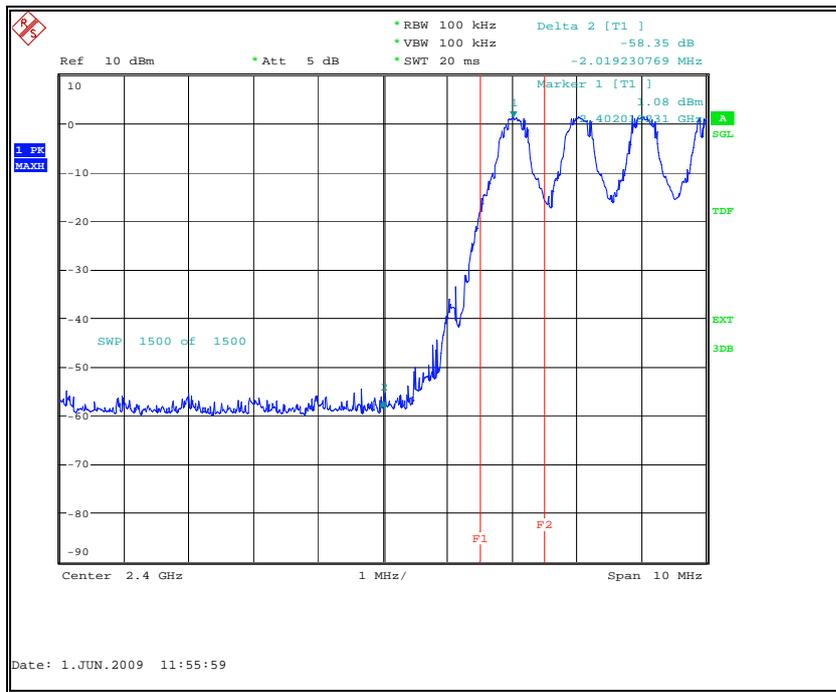
Fig. 2 Frequency Band Edges: Channel 0, Hopping On
