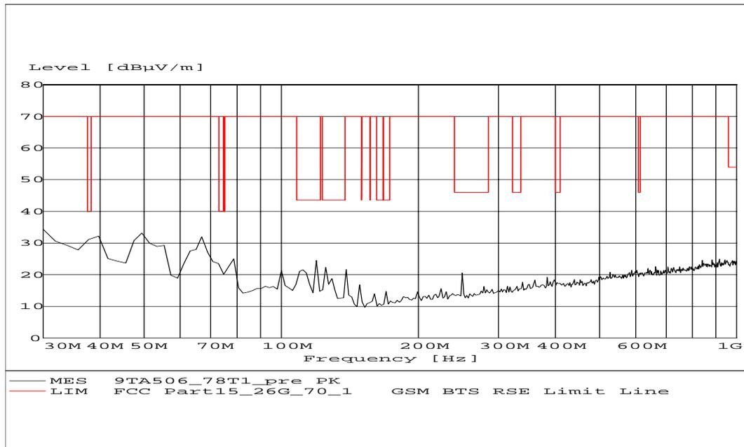
Fig. 20 Radiated emission: Channel 78, 30 MHz - 1 GHz
