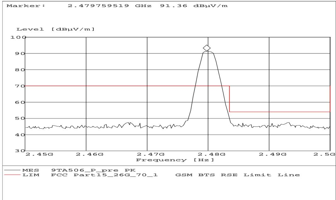
Fig. 23 Radiated emission (Power): 2.45GHz - 2.5GHz
