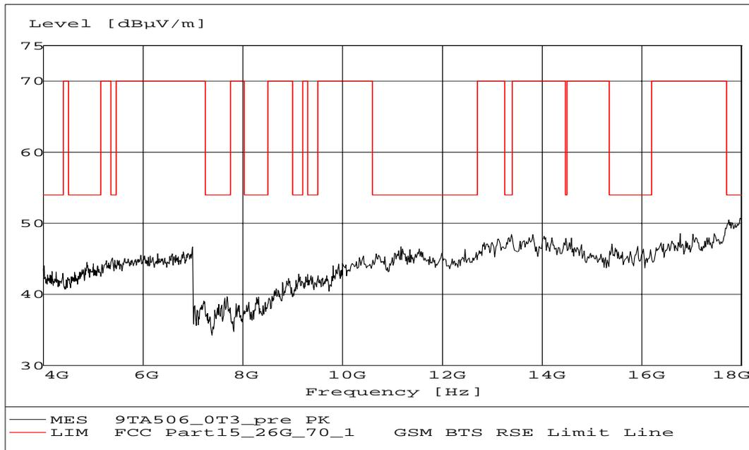
Fig. 16 Radiated emission: Channel 0, 4 GHz - 18 GHz
