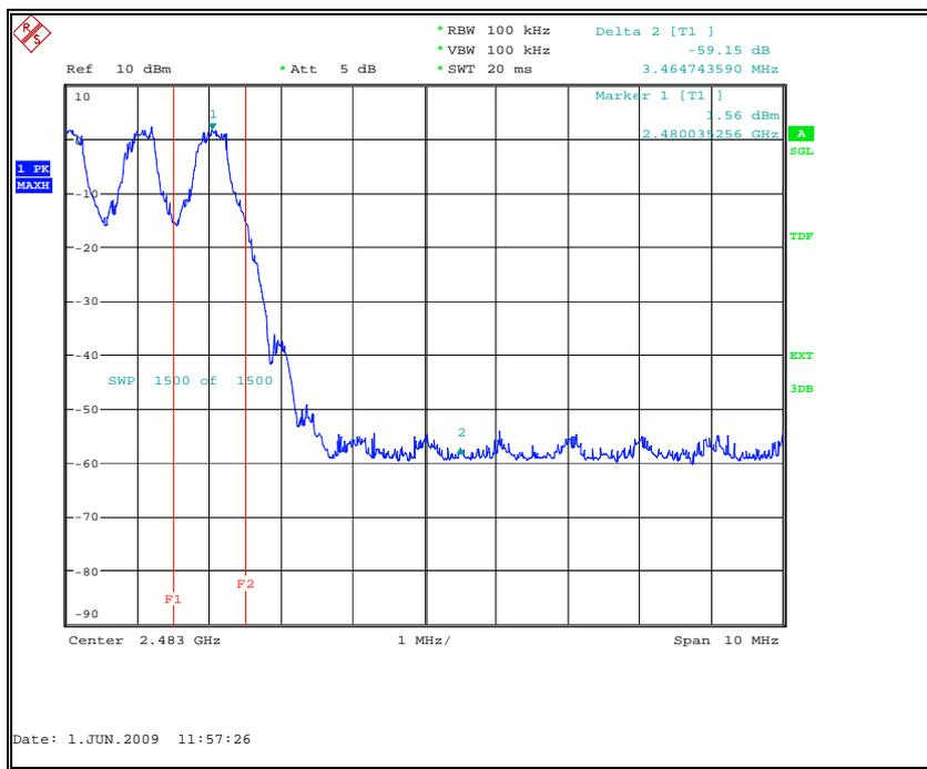
Fig. 4 Frequency Band Edges: Channel 78, Hopping On
