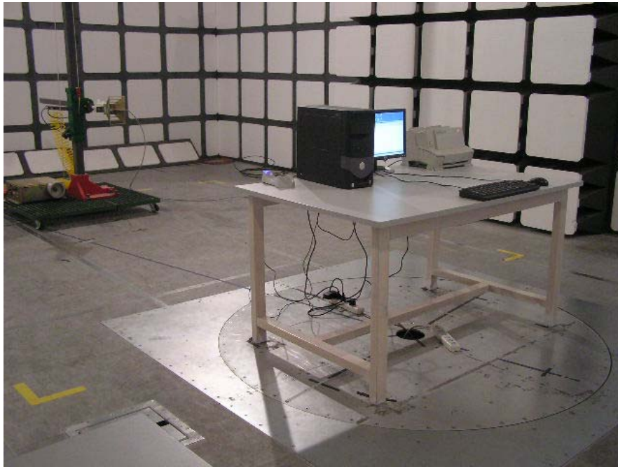
MI9535 Transmitting: Radiated Emission - Front View (Above 1 GHz)
