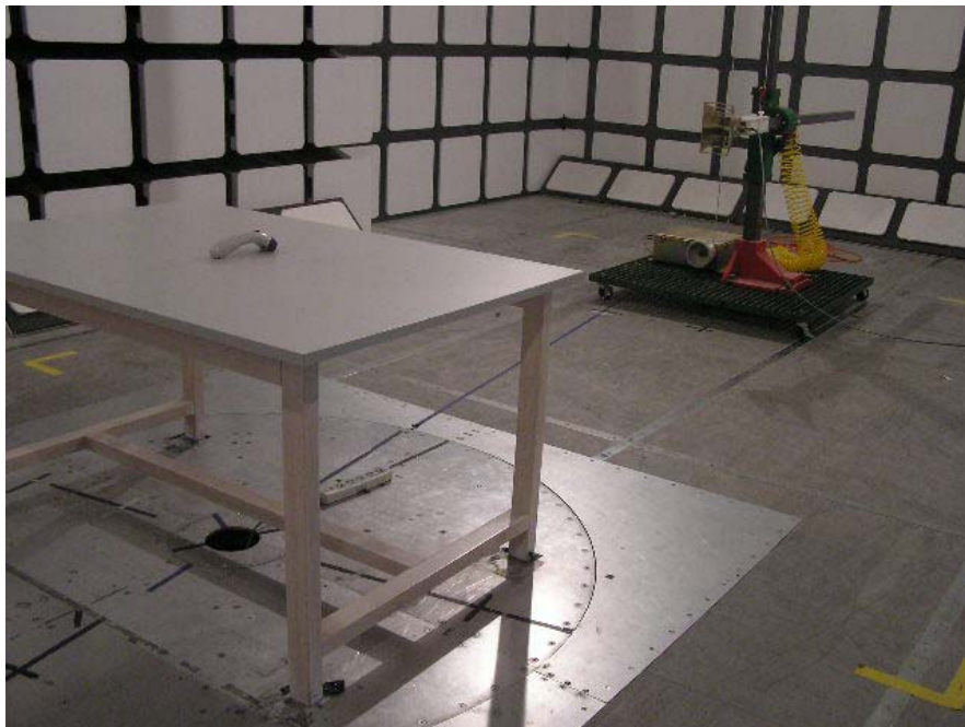
MS9535 Transmitting: Radiated Emission - Rear View (Above 1 GHz)
