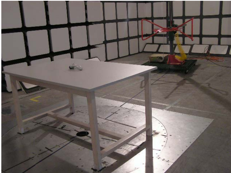
MS9535 Transmitting: Radiated Emission - Front View (30 MHz-1 GHz)
