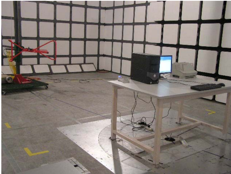
MI9535 Transmitting: Radiated Emission - Front View (30 MHz-1 GHz)
