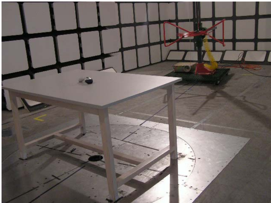
MS9535 Transmitting: Radiated Emission - Rear View (30 MHz-1 GHz)
