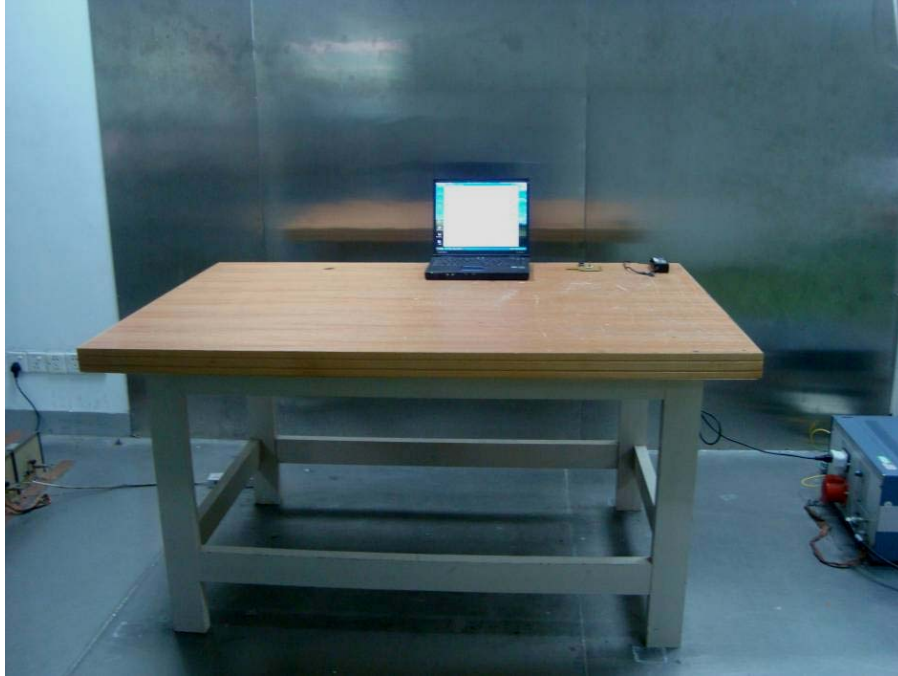
Conducted Emissions - Side View
