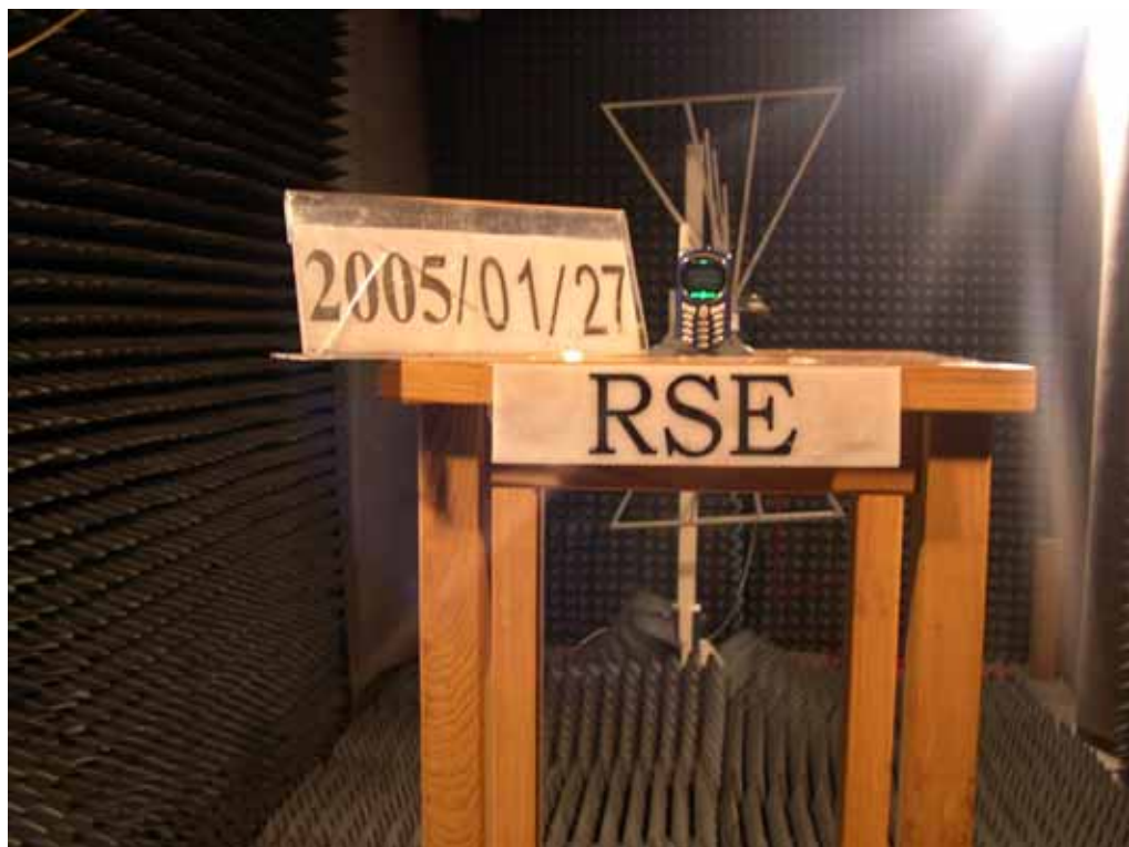
TCL558 Radiated Spurious Emission Test Setup
