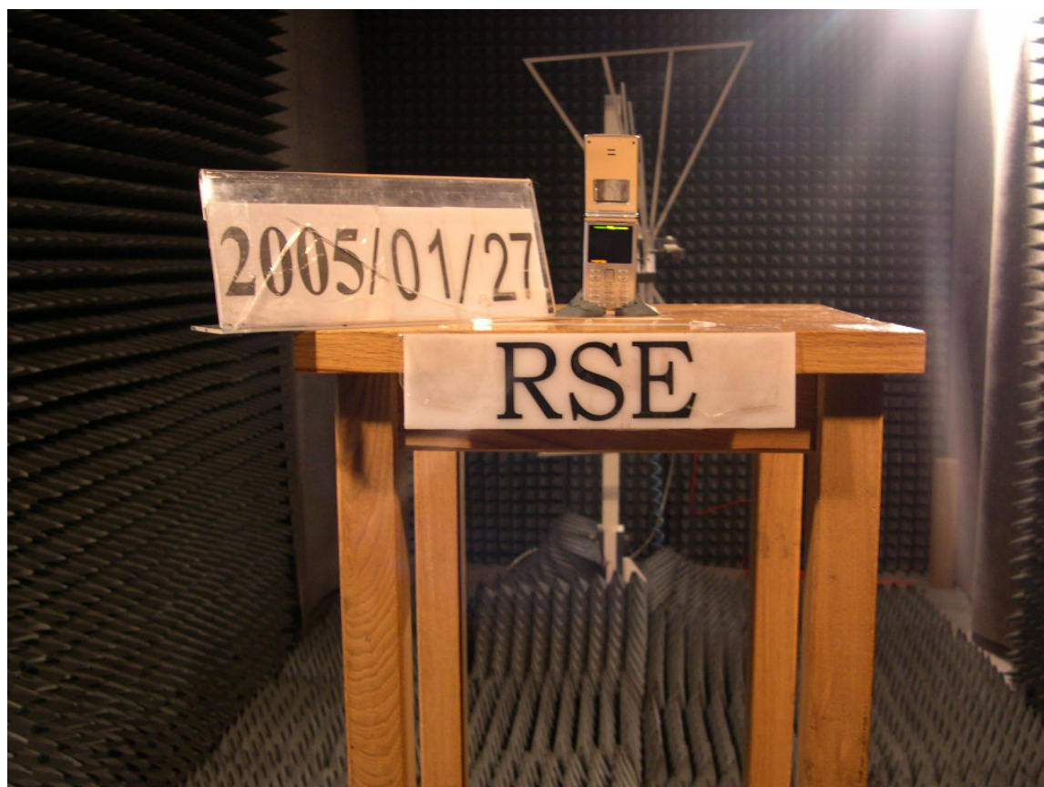
Pic2 Radiated Spurious Emission
