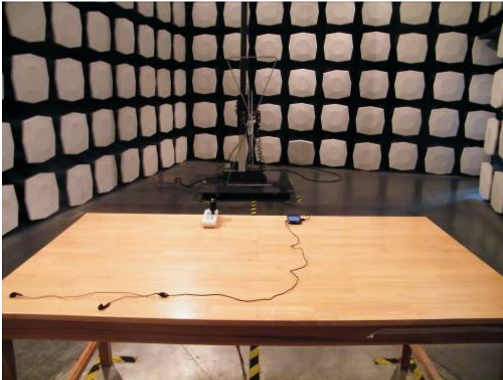
Picture 2 Radiated Emission Test Setup
