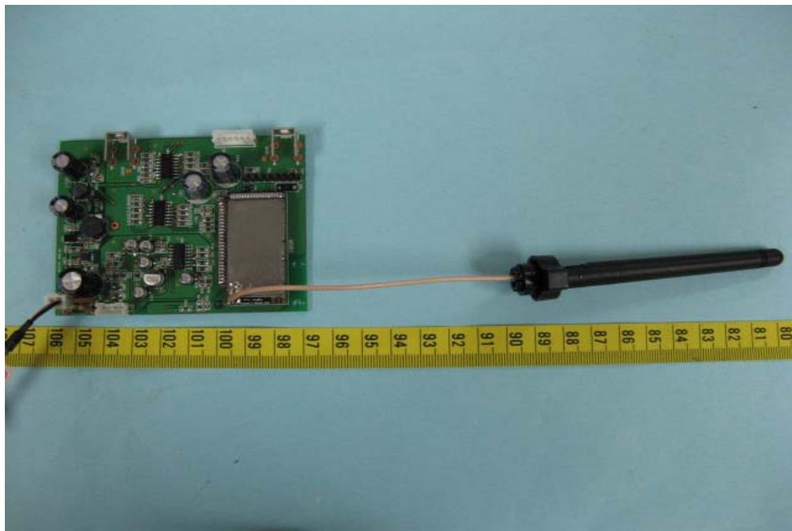
2. The EUT with its RF shielding
