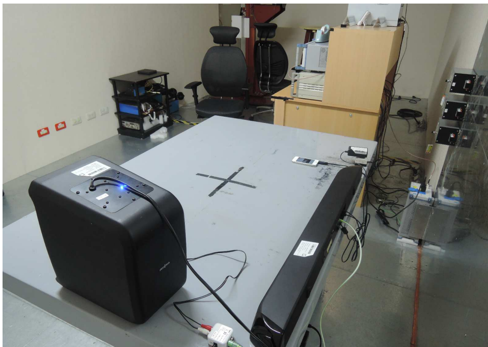
Photograph 5: Set-up for for Mains Conducted testing Back
