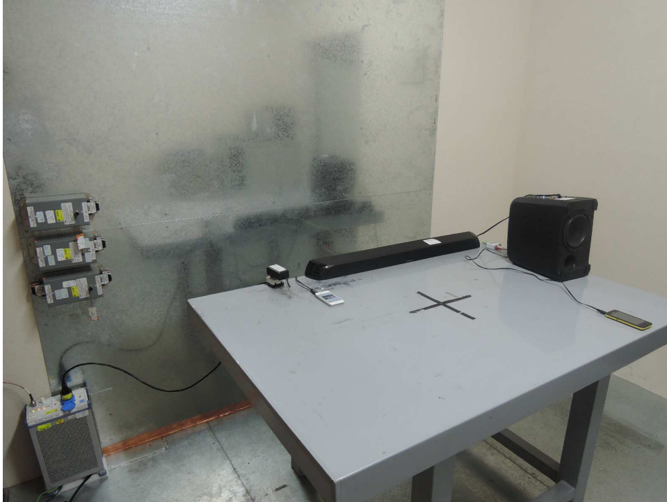
Photograph 6: Set-up for for Mains Conducted testing Front
