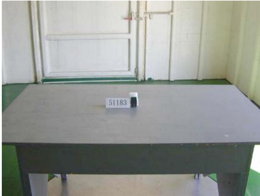
Photo 3: Radiated Emission Test Set-up (Tx)
