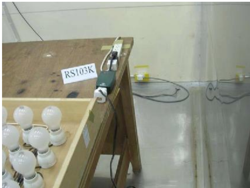
Photo 2: Conducted Emission Test Set-up
