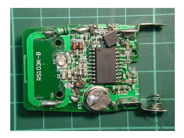
**Photo 5: Internal photo of Tx with two-buttons**
