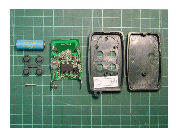
**Photo 2: Internal photo of Tx with four-buttons**
