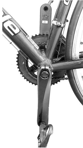
Figure 1. Non-Chain Arm in the 6 o'clock position. Always use this position for the zero offset calibration
