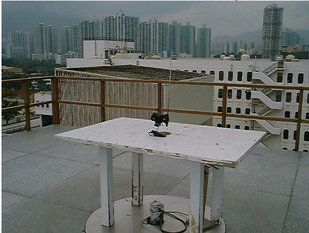
Measurement of Radiated Emission Test Set Up
