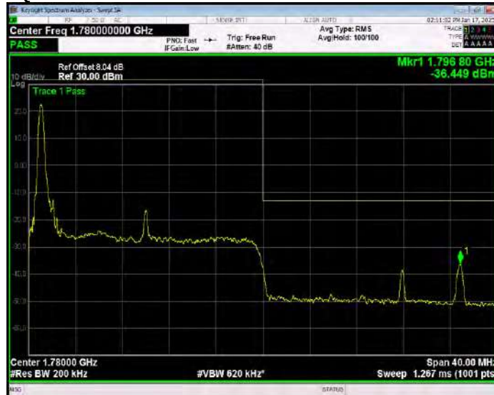
Band66 QPSK BW=20MHz Channel=132572 RB Size=1 Position=#Max Extended
