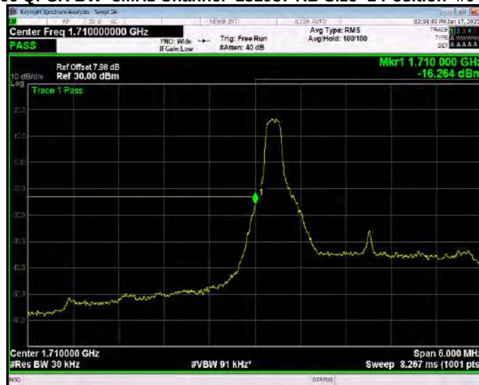
Band66 QPSK BW=3MHz Channel=131987 RB Size=1 Position=#Max Extended
