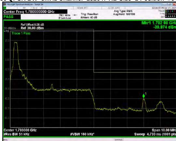
Band66 QPSK BW=5MHz Channel=132647 RB Size=1 Position=#Max Extended
