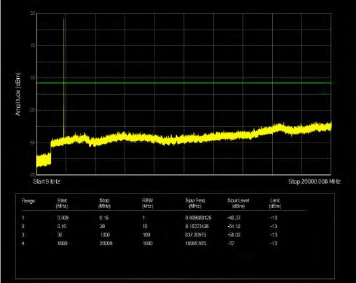
Band2 16QAM BW=1.4MHz Channel=19193 RB Size=1 Position=#0
