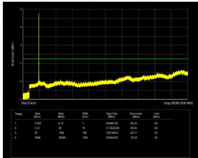
Band7 16QAM BW=5MHz Channel=21100 RB Size=1 Position=#0
