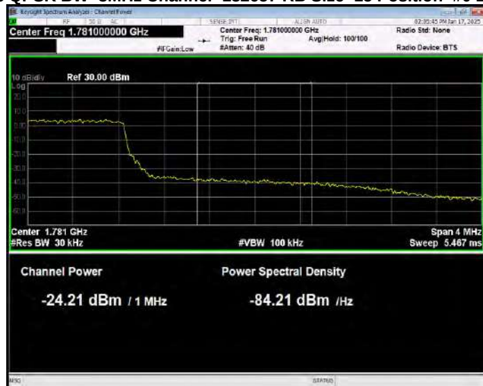
Band66 QPSK BW=3MHz Channel=132657 RB Size=15 Position=#0 Normal
