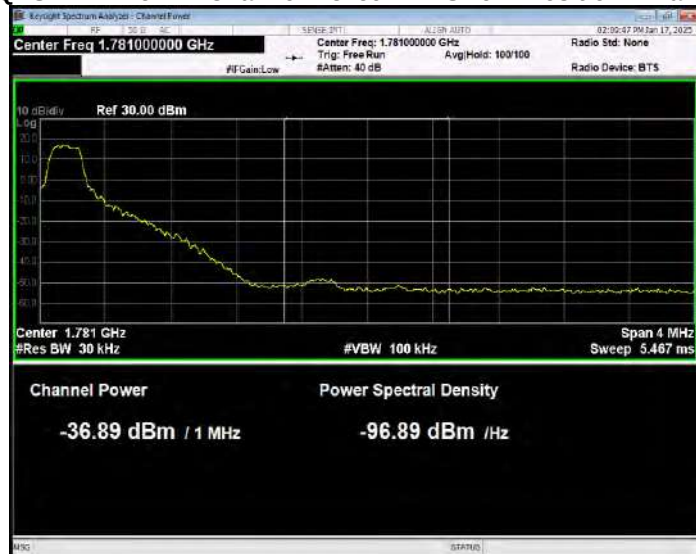
Band66 QPSK BW=15MHz Channel=132597 RB Size=1 Position=#Max Normal
