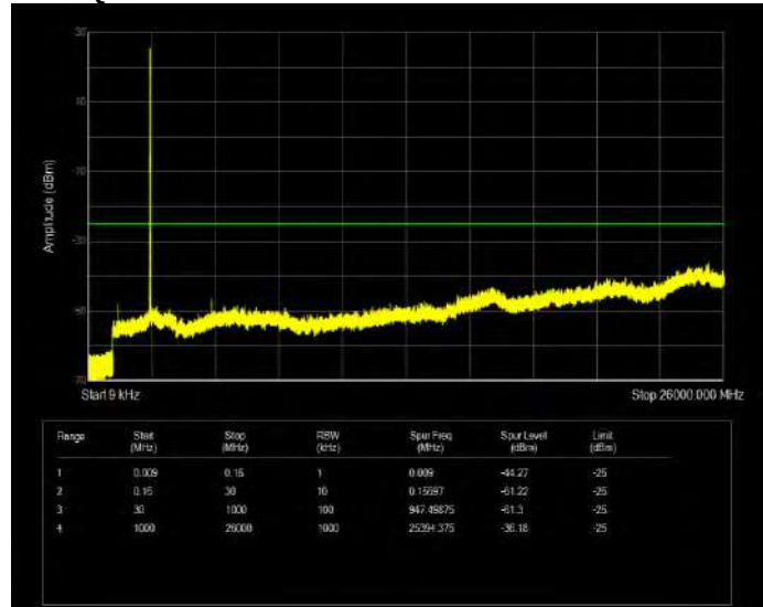
Band7 QPSK BW=5MHz Channel=21425 RB Size=1 Position=#0
