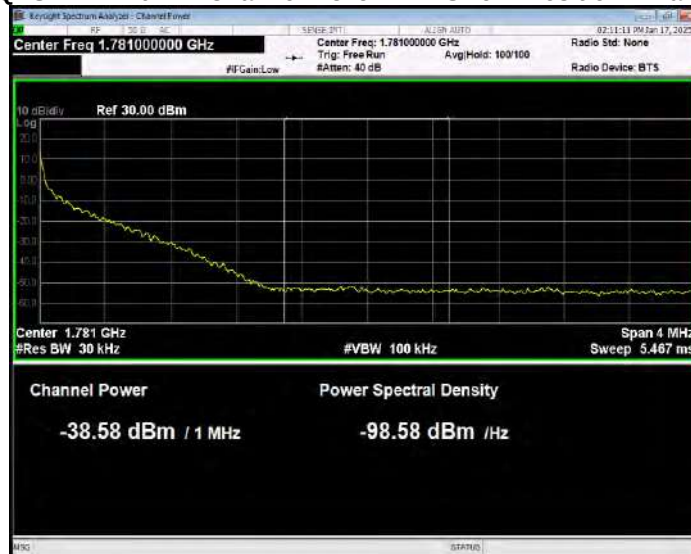
Band66 QPSK BW=20MHz Channel=132572 RB Size=1 Position=#Max Normal
