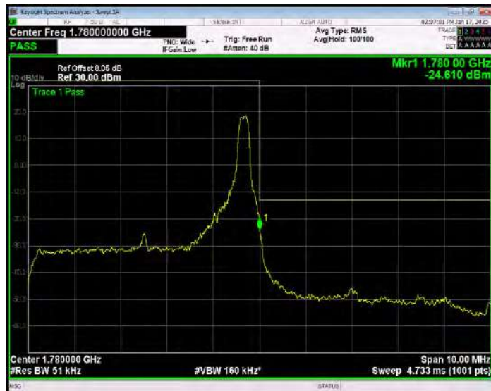
Band66 QPSK BW=5MHz Channel=132647 RB Size=25 Position=#0 Extended
