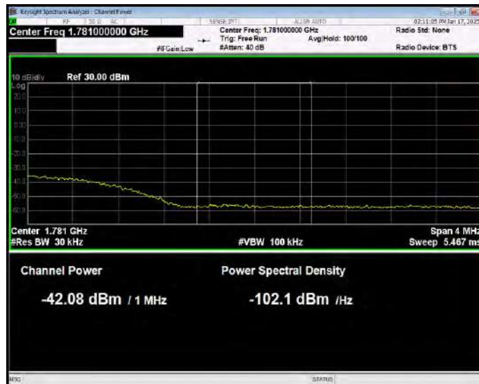
Band66 QPSK BW=20MHz Channel=132572 RB Size=1 Position=#0 Normal
