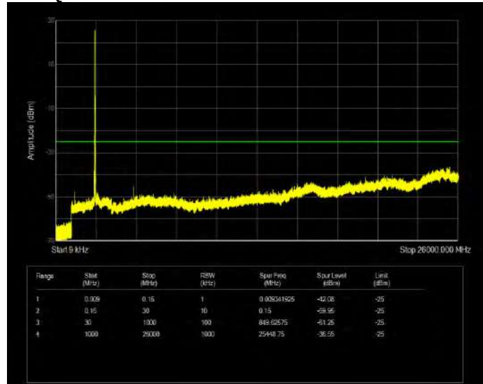
Band7 QPSK BW=15MHz Channel=21375 RB Size=1 Position=#0
