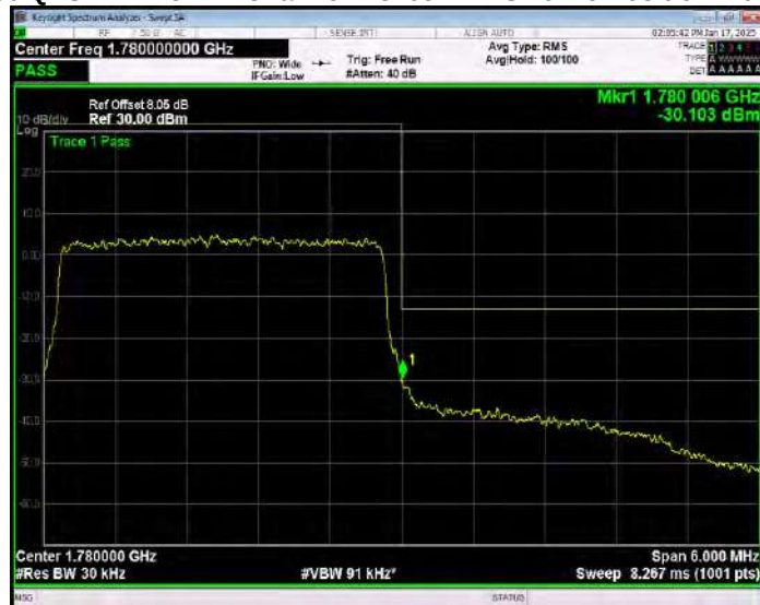
Band66 QPSK BW=5MHz Channel=131997 RB Size=1 Position=#0 Extended
