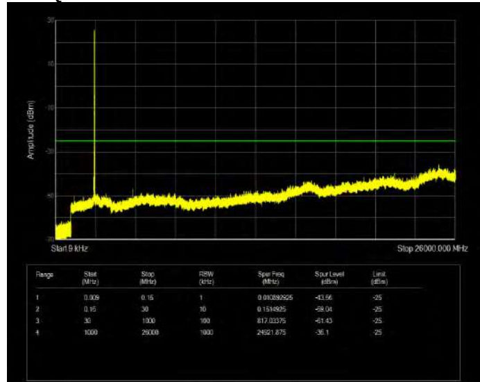
Band7 QPSK BW=10MHz Channel=21400 RB Size=1 Position=#0
