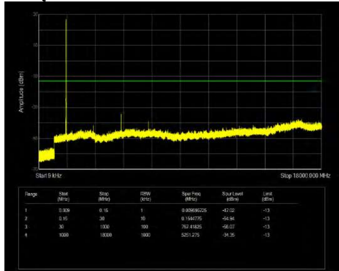
Band5 16QAM BW=1.4MHz Channel=20407 RB Size=1 Position=#0
