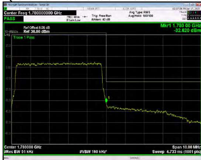
Band66 QPSK BW=5MHz Channel=132647 RB Size=25 Position=#0 Normal
