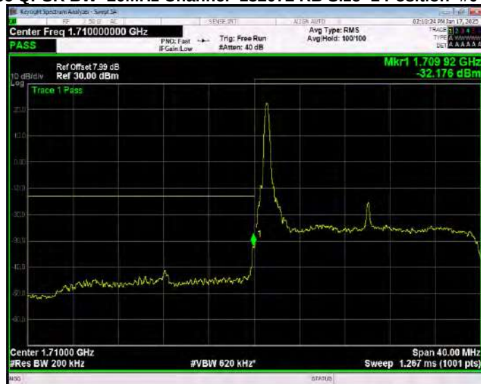
Band66 QPSK BW=20MHz Channel=132072 RB Size=1 Position=#Max Extended
