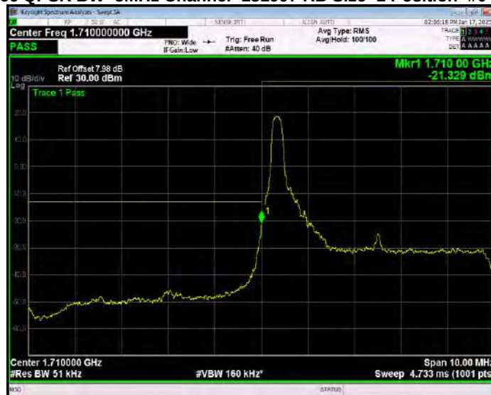
Band66 QPSK BW=5MHz Channel=131997 RB Size=1 Position=#Max Extended
