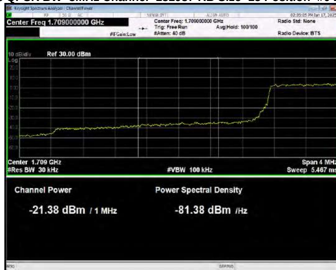
Band66 QPSK BW=3MHz Channel=131987 RB Size=15 Position=#0 Normal
