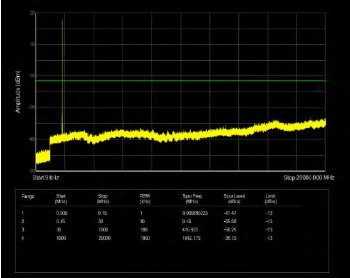
Band2 16QAM BW=1.4MHz Channel=18900 RB Size=1 Position=#0
