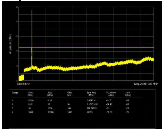
Band7 QPSK BW=20MHz Channel=21350 RB Size=1 Position=#0
