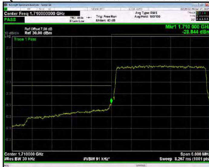
Band66 QPSK BW=3MHz Channel=132657 RB Size=1 Position=#0 Extended
