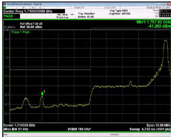
Band66 QPSK BW=5MHz Channel=131997 RB Size=25 Position=#0 Extended
