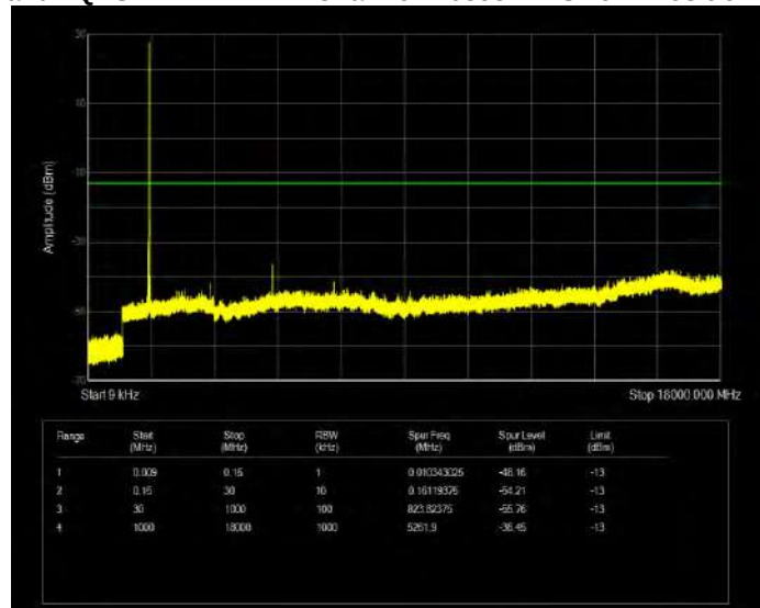
Band4 QPSK BW=10MHz Channel=20000 RB Size=1 Position=#0
