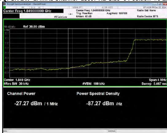
Band2 QPSK BW=1.4MHz Channel=18607 RB Size=6 Position=#0 Normal
