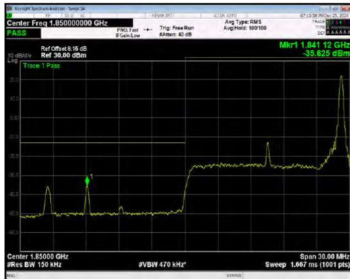
Band2 QPSK BW=15MHz Channel=18675 RB Size=75 Position=#0 Extended
