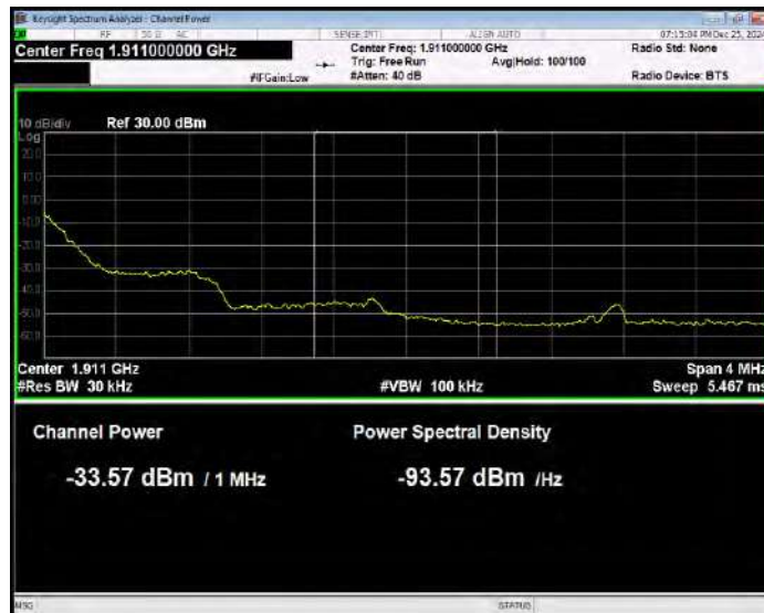
Band2 QPSK BW=1.4MHz Channel=19193 RB Size=1 Position=#0 Normal
