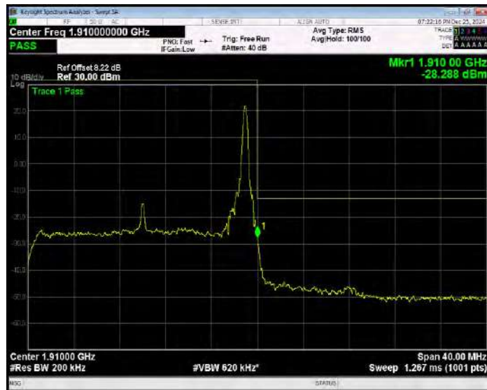
Band2 16QAM BW=20MHz Channel=19100 RB Size=100 Position=#0 Extended
