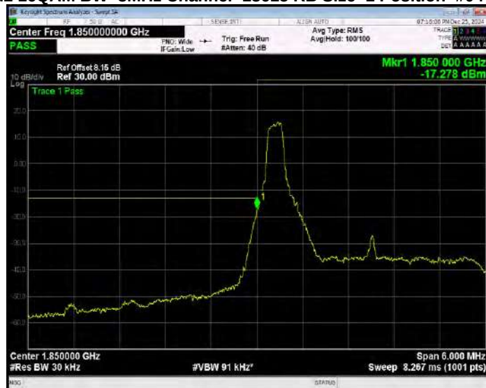
Band2 16QAM BW=3MHz Channel=18615 RB Size=1 Position=#Max Extended
