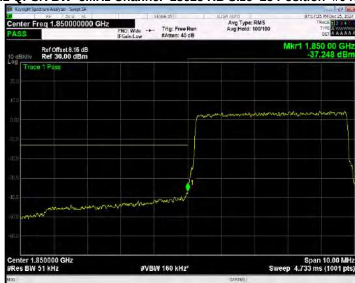
Band2 QPSK BW=5MHz Channel=19175 RB Size=1 Position=#0 Extended
