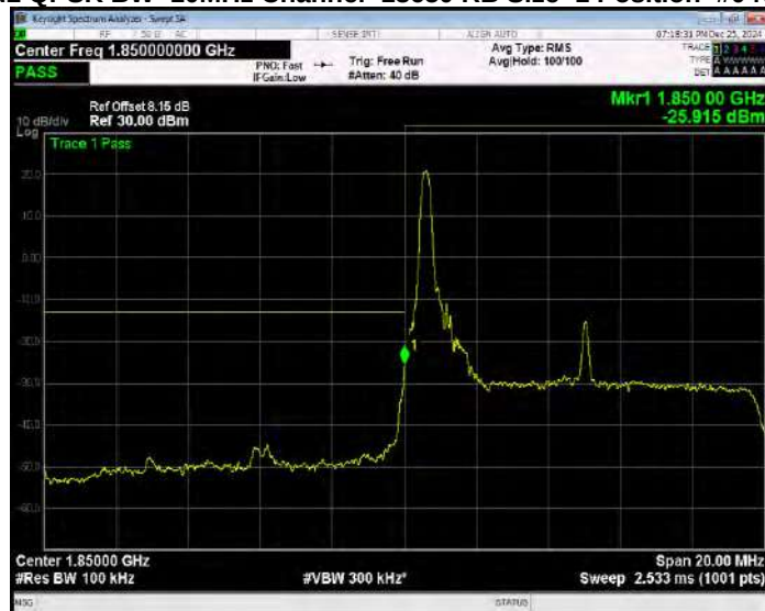
Band2 QPSK BW=10MHz Channel=18650 RB Size=1 Position=#Max Extended
