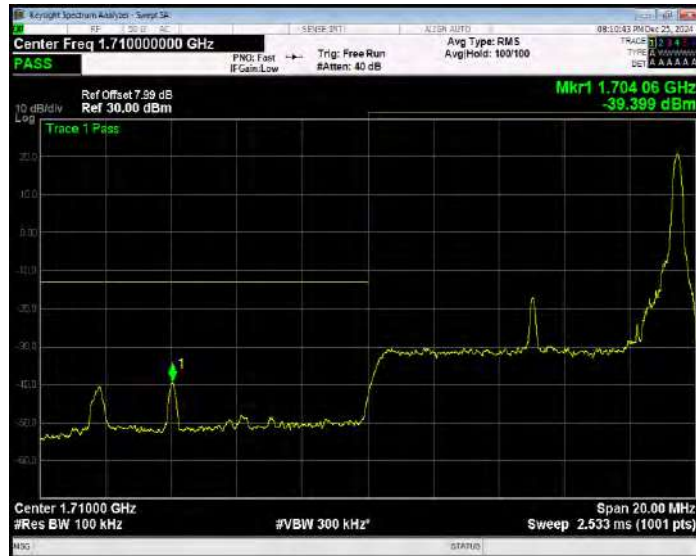
Band4 16QAM BW=10MHz Channel=20000 RB Size=50 Position=#0 Extended
