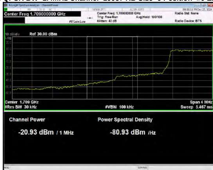
Band4 QPSK BW=1.4MHz Channel=19957 RB Size=6 Position=#0 Normal
