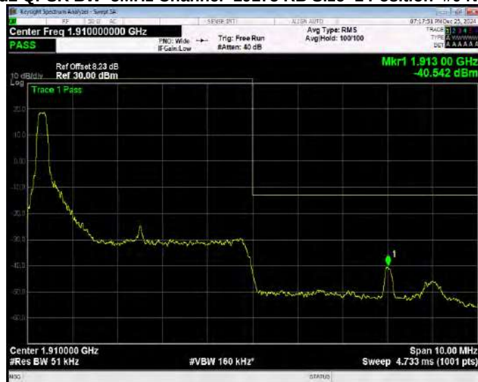
Band2 QPSK BW=5MHz Channel=19175 RB Size=1 Position=#Max Extended
