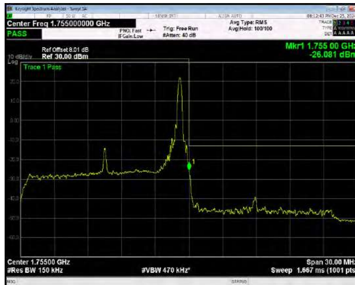
Band4 16QAM BW=15MHz Channel=20325 RB Size=75 Position=#0 Extended
