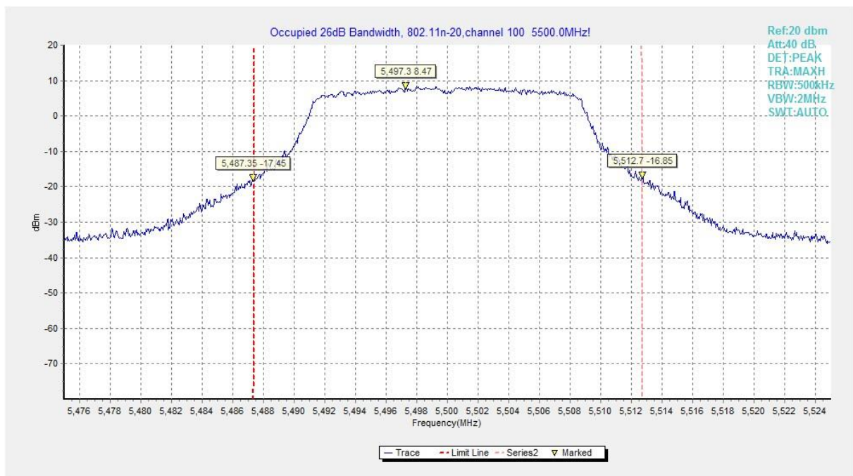
Fig. 16 Occupied 26dB Bandwidth (802.11n-HT20, 5500MHz)
