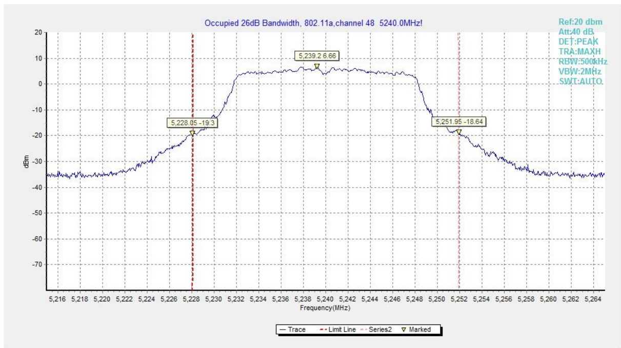
Fig. 3 Occupied 26dB Bandwidth (802.11a, 5240MHz)
