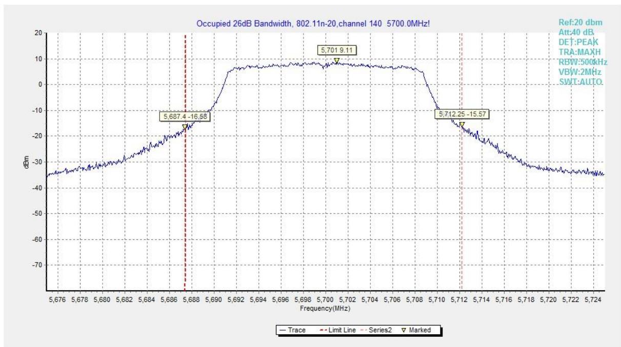
Fig. 18 Occupied 26dB Bandwidth (802.11n-HT20, 5700MHz)
