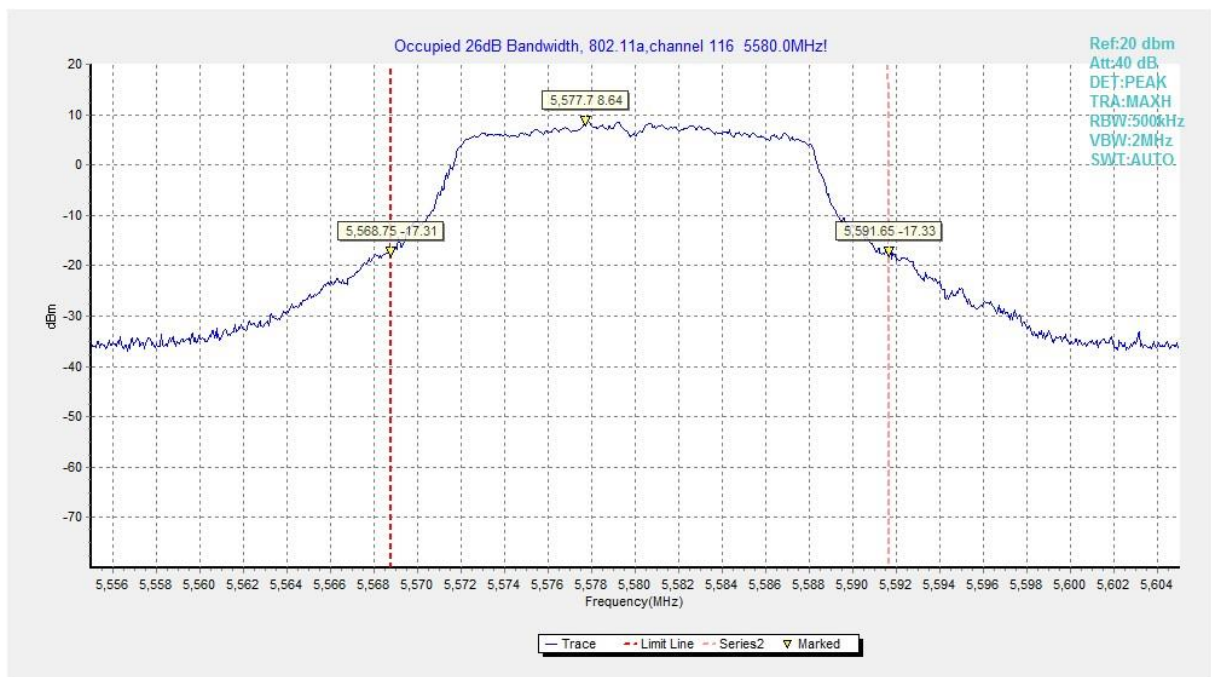
Fig. 8 Occupied 26dB Bandwidth (802. 11a, 5600MHz)
